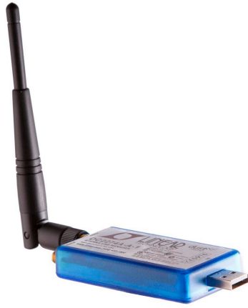
(a) DC2274: Low-power wireless manager (1 deployed)
