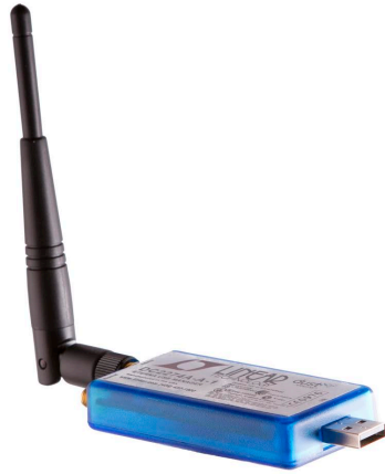
(a) DC2274: Low-power wireless manager (1 deployed)
