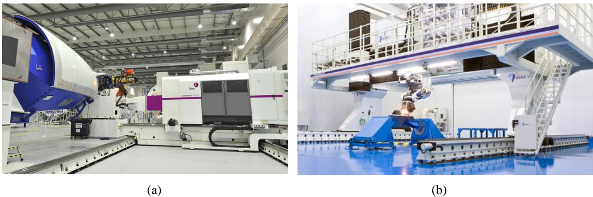
Figure 11 (a) Cincinnati VIPER™ platform for automated fiber placement, © Cincinnati VIPER™ (b) TORRESFIBERLAYUP machine for automated fiber placement, © MTorres.
