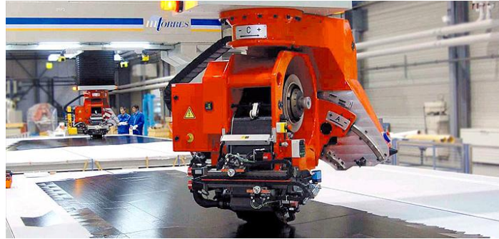
Figure 7 Typical automated tape laying system © MTORRES ( www.mtorres.com/ )
