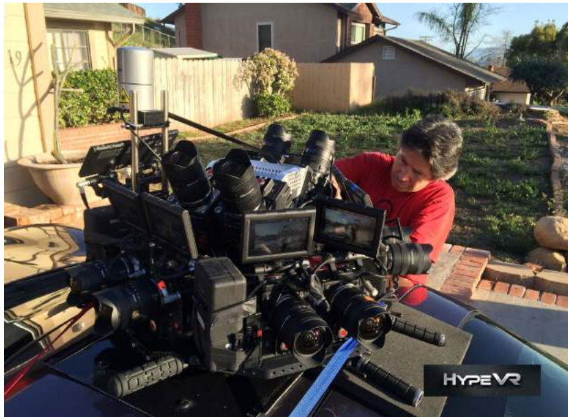
Figure 3.18: The VR capture system designed by HypeVR and Velodyne (figure taken from [Juchmann, 2015])
