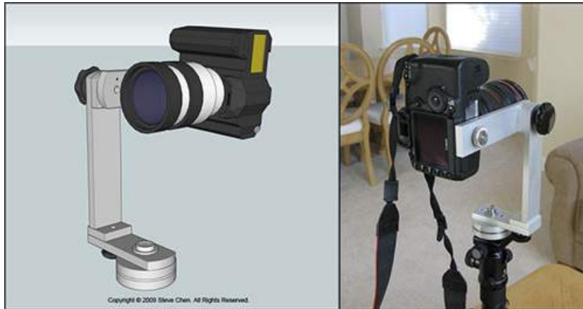
Figure 2.3: Camera gimbal for a parallax-free panorama
