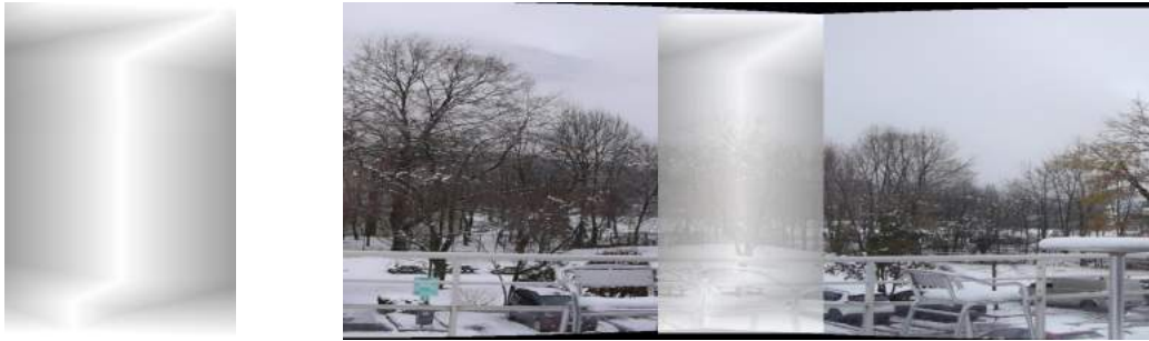
Figure 4.3: Example of the suggested mask created around the boundary of the blending line
