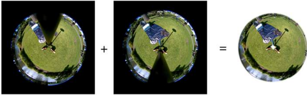
Figure 3.14: Removal of the tripod pole and generation of a new view using two cameras at the bottom of the Facebook Surround 360 rig. Figure taken from [Briggs, 2016]
