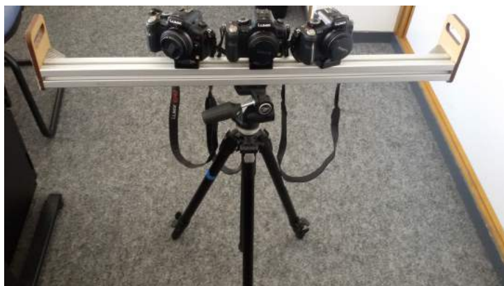
Figure 6.1: 3-camera rig designed with the help of engineers in Amigual4Home [Amigual4Home, 2016]
