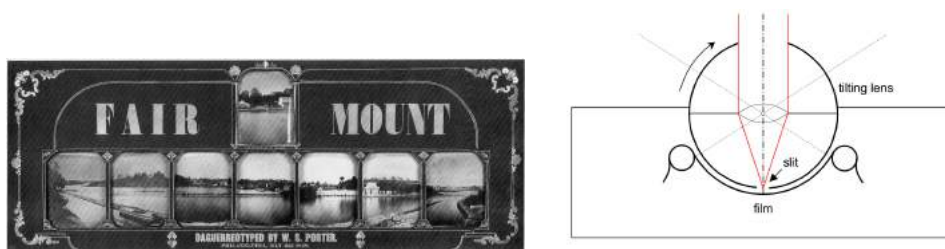
Figure 1.2: Left: Panorama created using 8 daguerrotypes in 1848. Right: Swing lens used for early panorama shooting. (figures taken from [Luhmann, 2004]).
