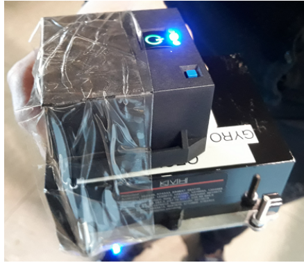
Fig. 3.3 The additional mass taped to ULISS device.
