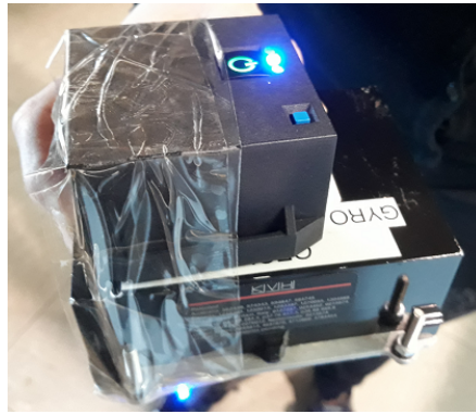
Fig. 3.3 The additional mass taped to ULISS device.
