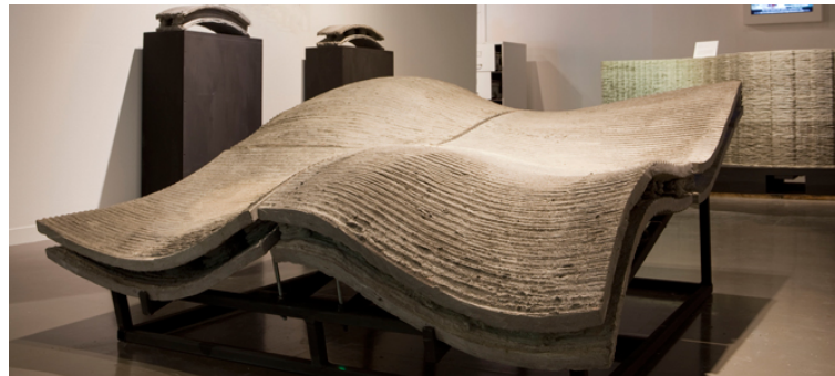
Figure 2.3 – Concrete Printing from Loughborough university
