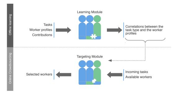
Figure 3.2: An overview on the workflow of CAWS.
