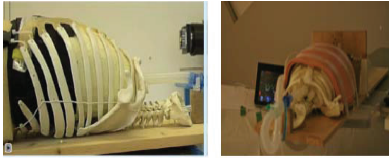
Figure 5.1 – Dynamic anthropomorphic breathing phantom, LuCa (Lung Cancer) developed by the Center for Proton Therapy at the Paul Scherrer Institute (PSI)
