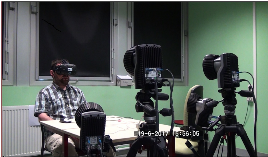
(b) Qualysis ® mocap system capturing mouth movement
