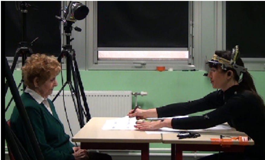
Figure 2.7 – Capturing the multimodal behavior of the human tutor during HHI. Movements of the upper limbs (head, arms and hands) are monitored by tracking 22 markers glued on these segments with a Qualysis ® mocap system. Gaze was tracked using a Perteck ® head-mounted eye tracker.
