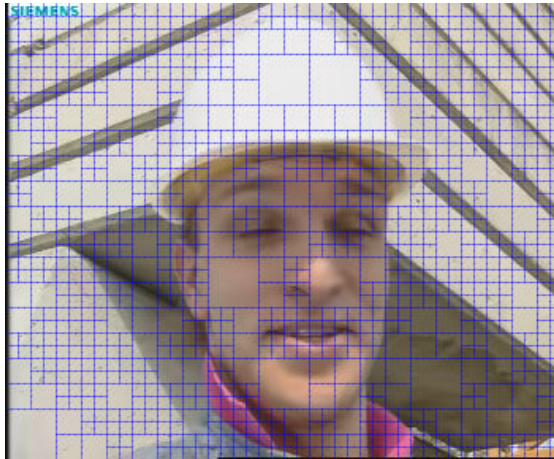
Figure 2.2: Example of the HEVC quad-tree partitioning on the “Foreman” sequence. Only the Coding Unit (CU) partitioning is represented here.
