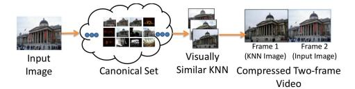
Figure 3.3: Overview of Perra & Frahm compression scheme [24]. The image to be encoded is matched to visually similar images via a k-nearest neighbour search in a large canonical database. From each image in the closest k results two-frame videos are encoded. The reference image yielding the best compression ratio is then selected, and the resulting bit-stream is stored. *Source*: Perra & Frahm [24].
