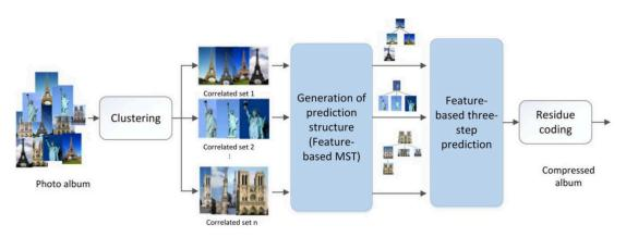
Figure 3.2: Photo album compression scheme of Shi *et al.* [21]. The images are first clustered by scenes based on clustered local features. Global geometric compensations are then derived from the locally matched features via RANSAC [22] and the geometric distortions are corrected. Finally, local disparities are compensated with residual coding by encoding the tree as a pseudo-video sequence. *Source:* Shi *et al.* [21].
