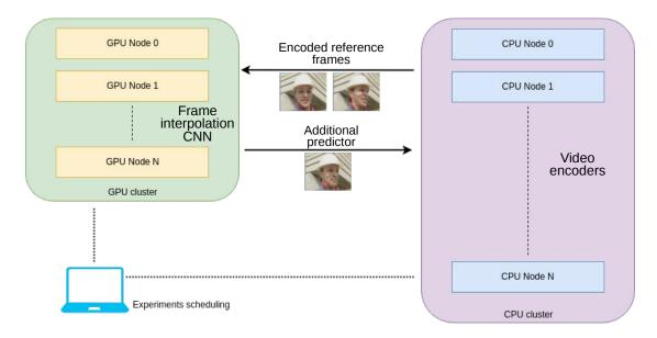
Figure 6.3: Illustration of the experimental setup for running the compression experiments.
