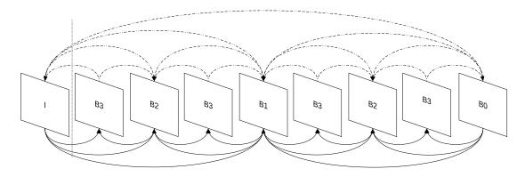
Figure 6.4: Coding scheme: illustration for a GOP of 8 frames with the default *random access* configuration. The dashed lines on top represent the default references, the straight lines below represent the extra reference from the interpolation.
