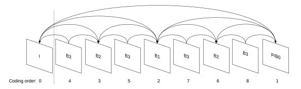
Figure 2.6: A traditional hierarchical GOP structure. P and B frames can be predicted from multiple reconstructed reference frames.
