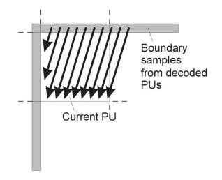
Figure 2.5: Intra prediction pixel samples available from the neighbouring reconstructed blocks.
