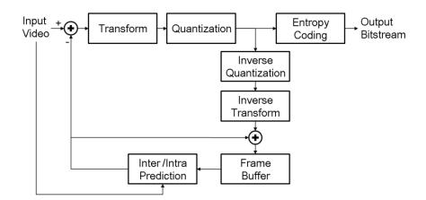
Figure 2.1: Illustration of the hybrid video coding framework [10].
