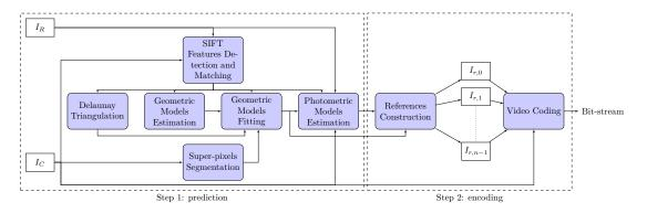
Figure 5.2: Illustration of the proposed compression scheme.
