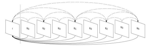
Figure 5.10: Coding scheme: illustration for a GOP of 8 frames with the default *random access* configuration. The dashed lines on top represent the default references, the straight lines below the extra reference for the proposed mode.
