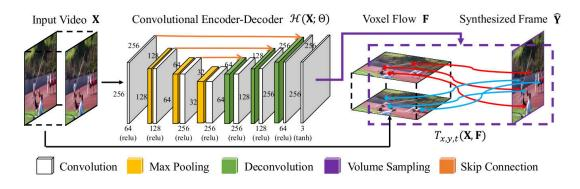
Figure 6.1: Deep Voxel Flow architecture [67].
