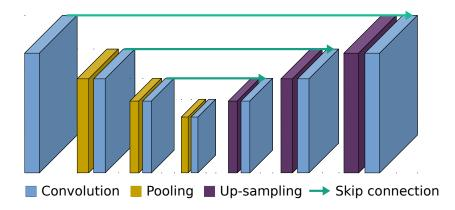
Figure 3.5: Convolutional auto-encoder architecture. The skip connections allow the network to keep spatial details and high level information. Pooling layers are usually average or max pooling layers. The up-sampling layer can either be a simple bilinear up-sampling or a deconvolution operation. Trainable layers are followed by an activation function such as tanh or ReLU [72]. Batch normalization [73] may also be used before the activation function.
