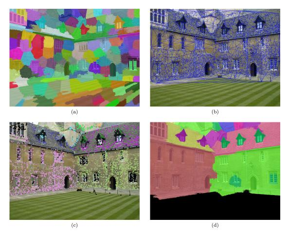
Figure 5.3: Region-based geometric estimation: (a) SLIC segmentation of  $I_C$ . (b) Mesh of the Delaunay triangulation of the matched keypoints. (c) Keypoints labels, each keypoint is assigned a homography model, the outliers points are represented in black. (d) Final region segmentation.
