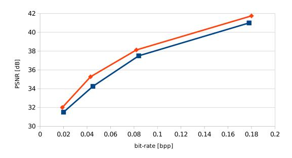
Figure 2.10: Example Rate-Distortion curve. Bit-rates and PSNRs are measured for four different quantization levels, *e.g.* 22, 27, 32 and 37 for HEVC.
