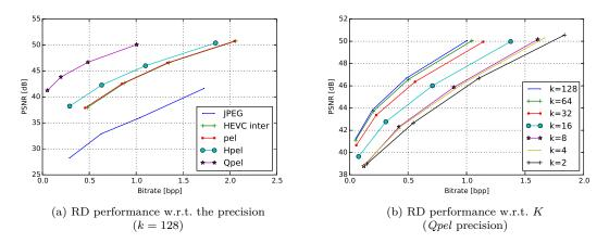
Figure 4.5: Rate-distortion (RD) performance comparison.
