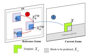
Figure 4.2: K-NN search in the reference image using template-matching.
