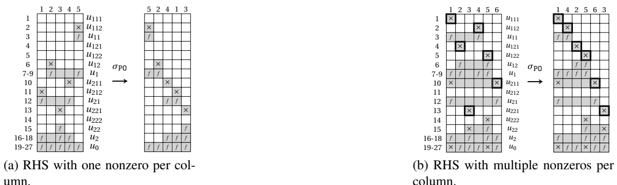
Figure 1.10: Illustration of the postordering of two RHS with one or more nonzeros per column.
