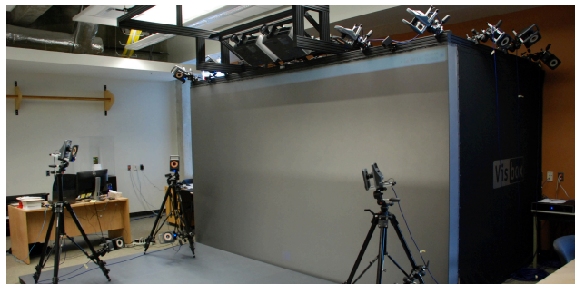
Figure 5.8: We built our true-3D prototype in a VisCube 3D immersive system, tracking the mobile device using optical tracking.
