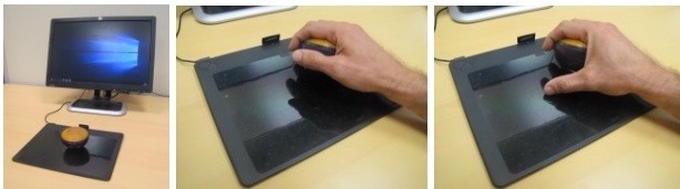
Figure 7. Overview of the RPM input apparatus (left): rolling RPM (centre) and tapping on the tablet to validate (right).
