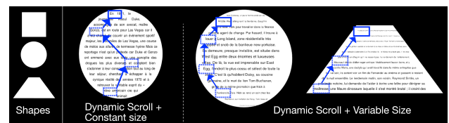
Figure 8. Shapes used in exp. 4 to test the combination of Scroll type and Token Size. Blue boxes and arrows illustrate how a word would move when text is dynamically scrolled.
