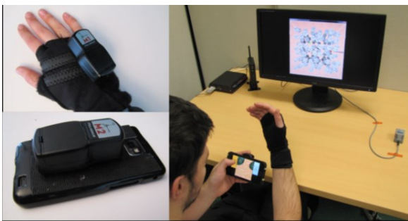
Figure 3. Tracker on hand and on smartphone (left) and user performing the Mid-Air Hand technique (right).
