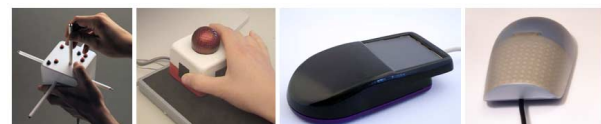
Figure 6: From left to right, the Cubic Mouse [14], the GlobeMouse [13], the PadMouse [2] and the CapMouse [40].
