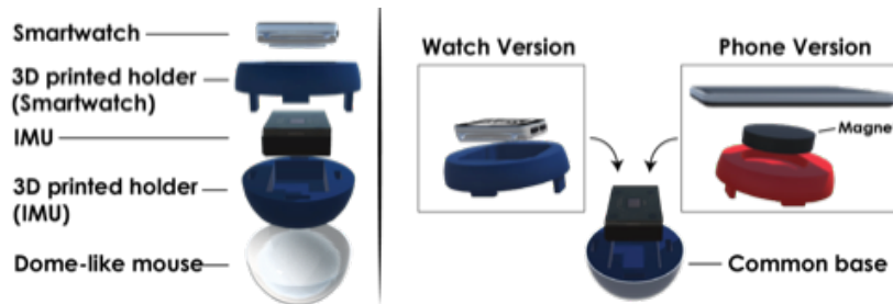
Figure 3.7: Arrangement of TDome elements.
