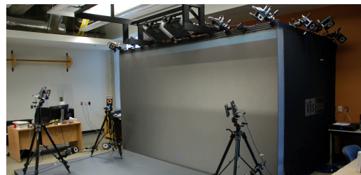
Figure 3. We built our prototype in a VisCube 3D [27] immersive system, tracking the mobile device using optical tracking.
