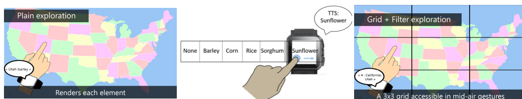
Figure 2.11: We investigated three non-visual map exploration techniques: plain (left), filter (center) and grid-filter explorations (right).
