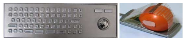
Figure 4: Illustration of the Human effectors property. Trackball keyboard [37]: <keyboard: non dom. hand; trackball: dom. hand> (left). The Inflatable Mouse [22]: <mouse: dom. hand; balloon: dom. hand> (right).
