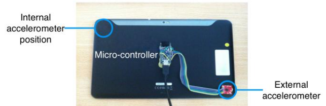
Figure 3. Test prototype with an external accelerometer.
