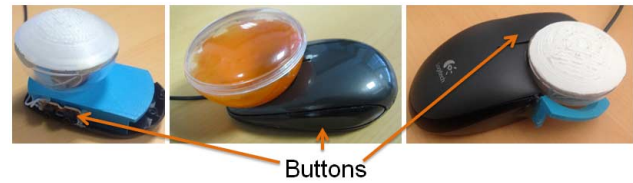
Figure 8: Different versions of the (A←B) compound device, from left to right: based on a 3D printed support (prototype v2), carved on the center of the mouse (prototype v3a) and carved on the right side of the mouse (prototype v3b)
