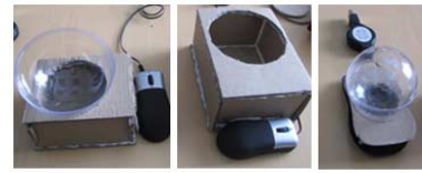
Figure 7: Cardboard prototypes of RPM2: the mouse is on the right side (left), on the back (center) or under (right) RPM.
