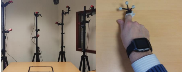
Figure 4. Left: Experimental setup with the infrared cameras. Right: marker on the finger.
