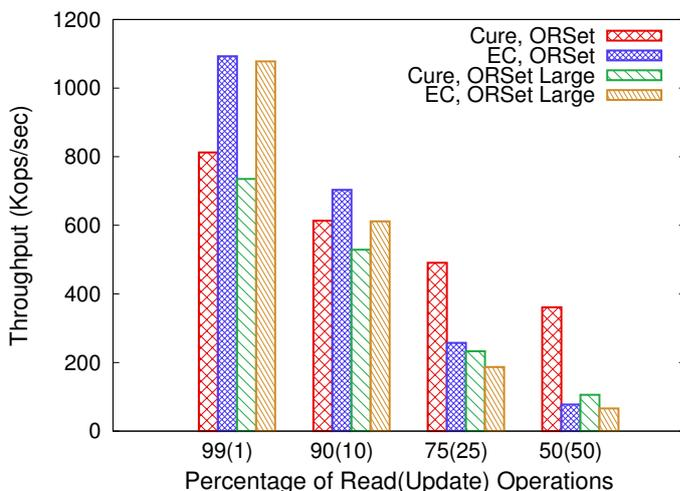
Figure 7.3: Comparison of Cure to an eventually-consistent system using CRDT sets.
