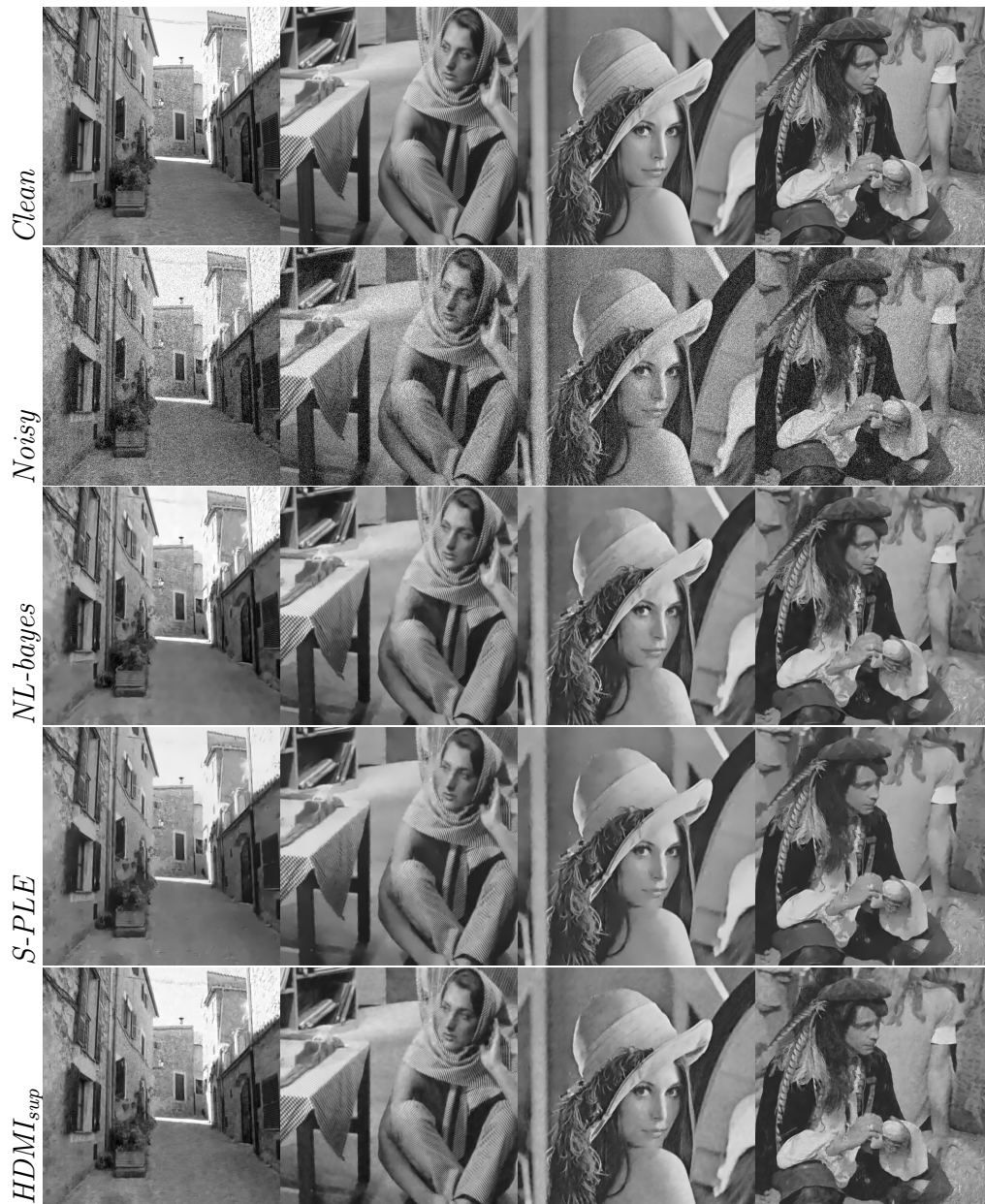
Figure 4.10 – Comparative results on the grey-scale images Alley , Barbara , Lena and Man with \sigma = 30 . For each column, from top to bottom: original image, noisy image, NL-Bayes [35], SURE-PLE [71], HDMI. Images should be seen at full resolution on the electronic version of the manuscript.
