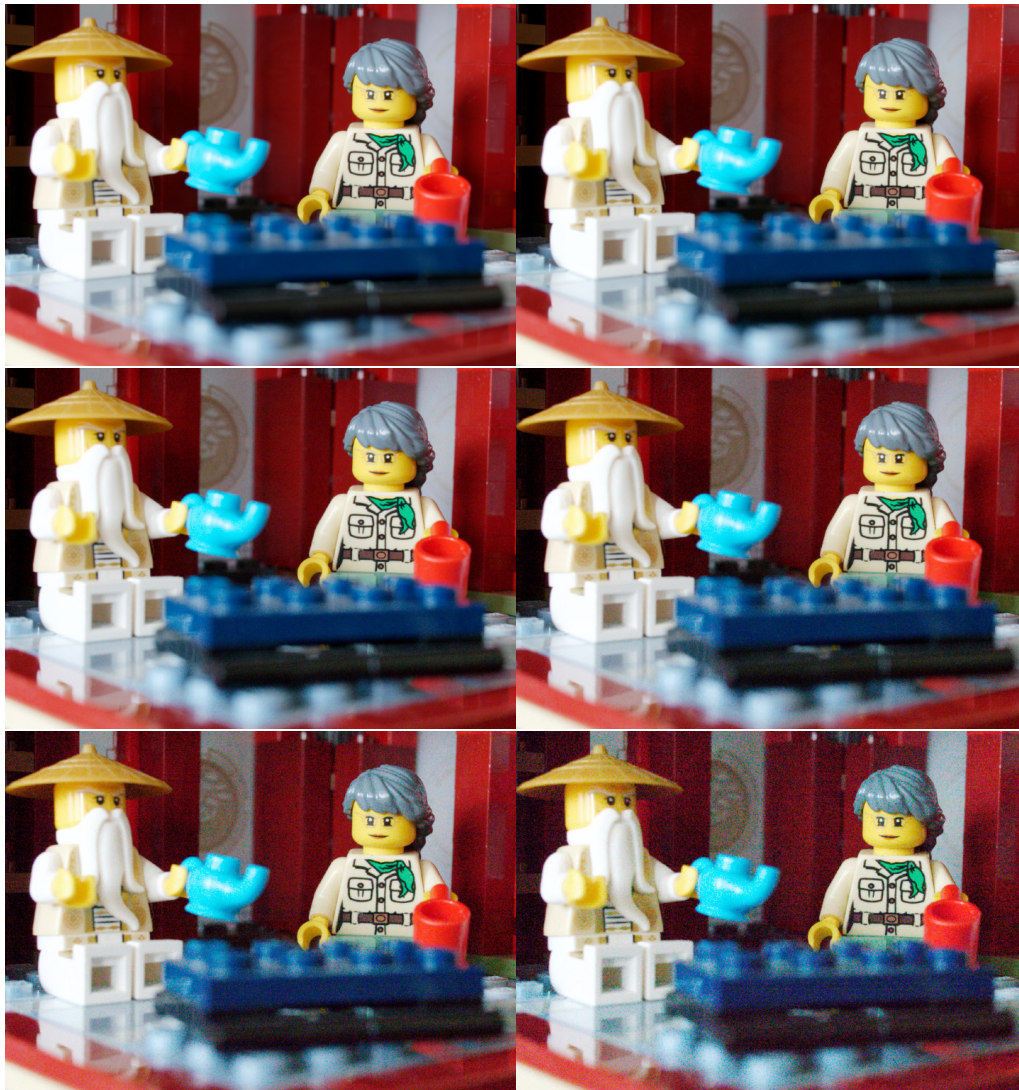
Figure 1.4 – Real noise in images. The same scene shot at different ISO settings but with constant exposure. From left to right and top to bottom , 200 ISO, 800 ISO, 3200 ISO, 6400 ISO, 12800 ISO and 25600 ISO. Lower ISOs are compensated by longer exposures to achieve an equivalent brightness level. In practice larger ISOs are necessary in low light and/or highly dynamic scenes which would result in motion blur with longer exposures. Images credit Julie Delon.
