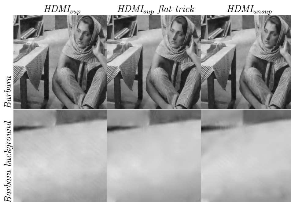
Figure 4.13 – Result of HDMI denoising with K = 40 groups for the image Barbara with noise \sigma = 30 . Left HDMI (PSNR = 29.35dB), middle HDMI with the flat area trick (PSNR = 29.36dB), right unsupervised HDMI (PSNR = 29.11dB).
