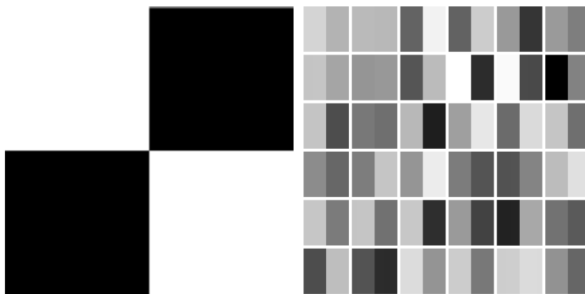
Figure 3.2 – Left: a covariance matrix \Sigma with 1 (white) on the second and third quarters, and 0 (black) on the first and fourth quarters. Right: patches drawn from the Gaussian distribution \mathcal{N}(\mu, \Sigma) with \mu a constant patch equal to 0.5.
