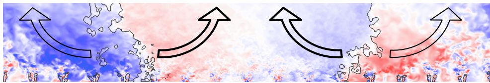
Figure 5.27: Field of azimuthal velocity at t = 30 ms (see Fig. 5.26d). Arrows indicate the streamlines in the fresh gases (thick lines) and burnt gases (thin line).
