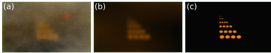
Figure 5.1: (a) Illustration of an aircraft landing scenario in low visibility conditions due to the presence of intense background illumination (ambient spurious light) and strong light scattering causing reduction of the visibility and of the spatial resolution of the light beacons. (b) Illustration of the resulting image after perfect background removal processing. (c) Illustration of the resulting image expected after ideal ballistic photon imaging process.
