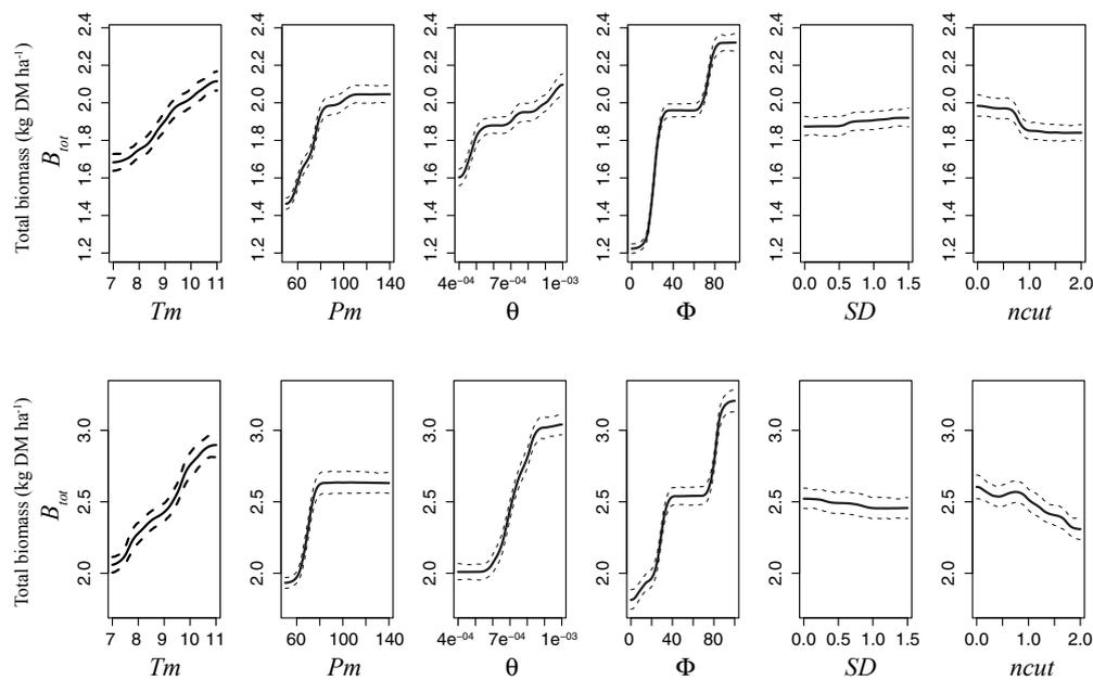
**Figure III.11** – Main effects of six key parameters on total biomass  $B_{tot}$ , from dynamic trees performed on *DynaGraM2* (A) and *DynaGraM21* (B) outputs. Climate parameters:  $Tm$  (temperature),  $Pm$  (precipitation); soil fertility parameters:  $\Phi$  (fertiliser input),  $\theta$  (mineralization rate); defoliation parameters:  $SD$  (livestock density),  $ncut$  (mowing frequency).
