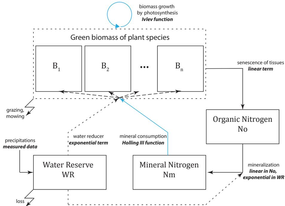
**Figure II.1** – Structure of the *DynaGraM* model and link between all state variables. For more details, refer to Table II.1. Solid lines denote flows of matter or energy and dashed lines denote reducers. Blue arrows correspond to the two main processes described in equations (II.1) and (II.2).
