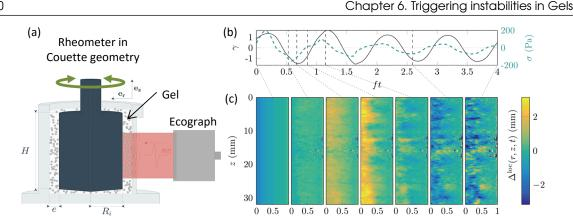
Figure 6.4: Large Oscillatory Rheology from Echography (LORE) to study rupture of a casein gel. (a) LORE [336]. (b) Strain  $\gamma$  and stress  $\sigma$  as a function of *ft* during the rupture of a casein gel. Note that the rheometer fails to apply a perfectly constant amplitude. (c) Local displacement maps  $\Delta^{loc}$  obtained with LORE [248] during gel breakdown.
