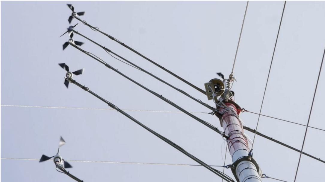
**Figure 4.9:** Photo of the sensors on the met mast
