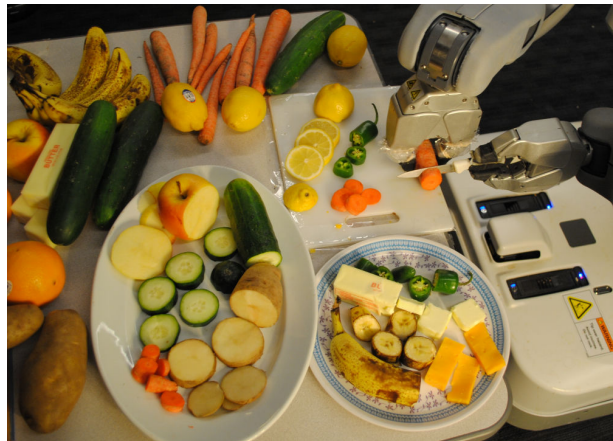
Figure 1.9 – The PR2 robot learning Deep MPC control for slicing food from [Lenz et al., 2015].
