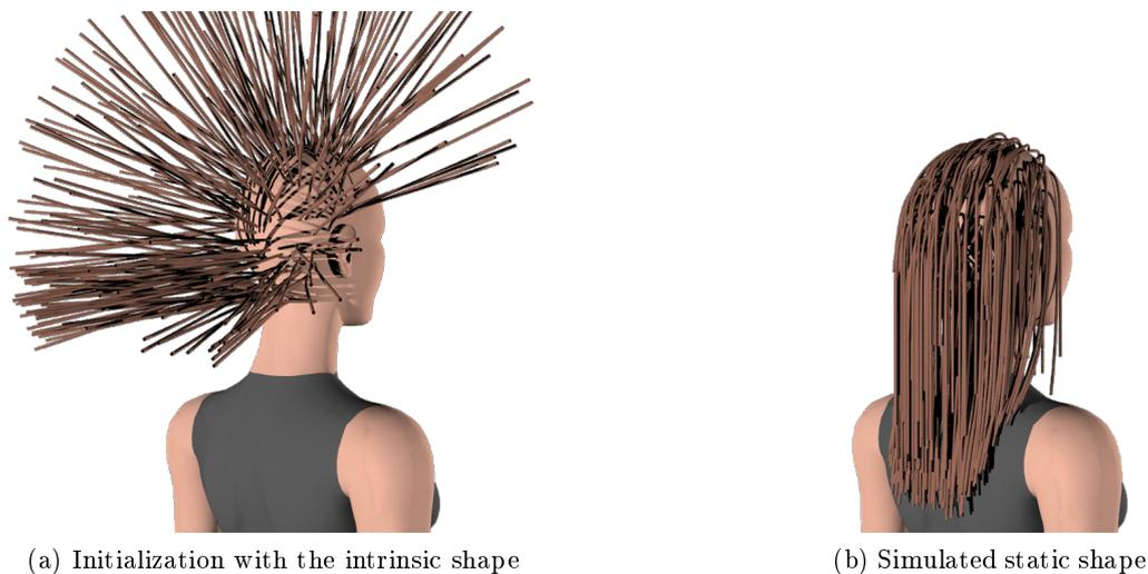
Figure 4.2 – Classical initialization of a physics-based simulator. The initial configuration  $\mathbf{q}(t = 0)$  is set to a trivial intrinsic shape  $\bar{\mathbf{q}}$  — here, a set of straight rods (a). Then, after feeding the simulator with other parameters (such as the mass and stiffness of each rod), a static shape  $\mathbf{q}^{\text{eq}}$  can be computed under gravity and frictional contacts (b).
