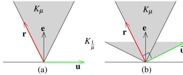
Figure 3.7 – Changes of variables applied onto (a) the relative velocity  $\mathbf{u}$  and the contact force  $\mathbf{r}$ , in order to exhibit (b) the complementarity of  $\tilde{\mathbf{u}}$  and  $\mathbf{r}$  proposed by De Saxcé and Feng [1998].
