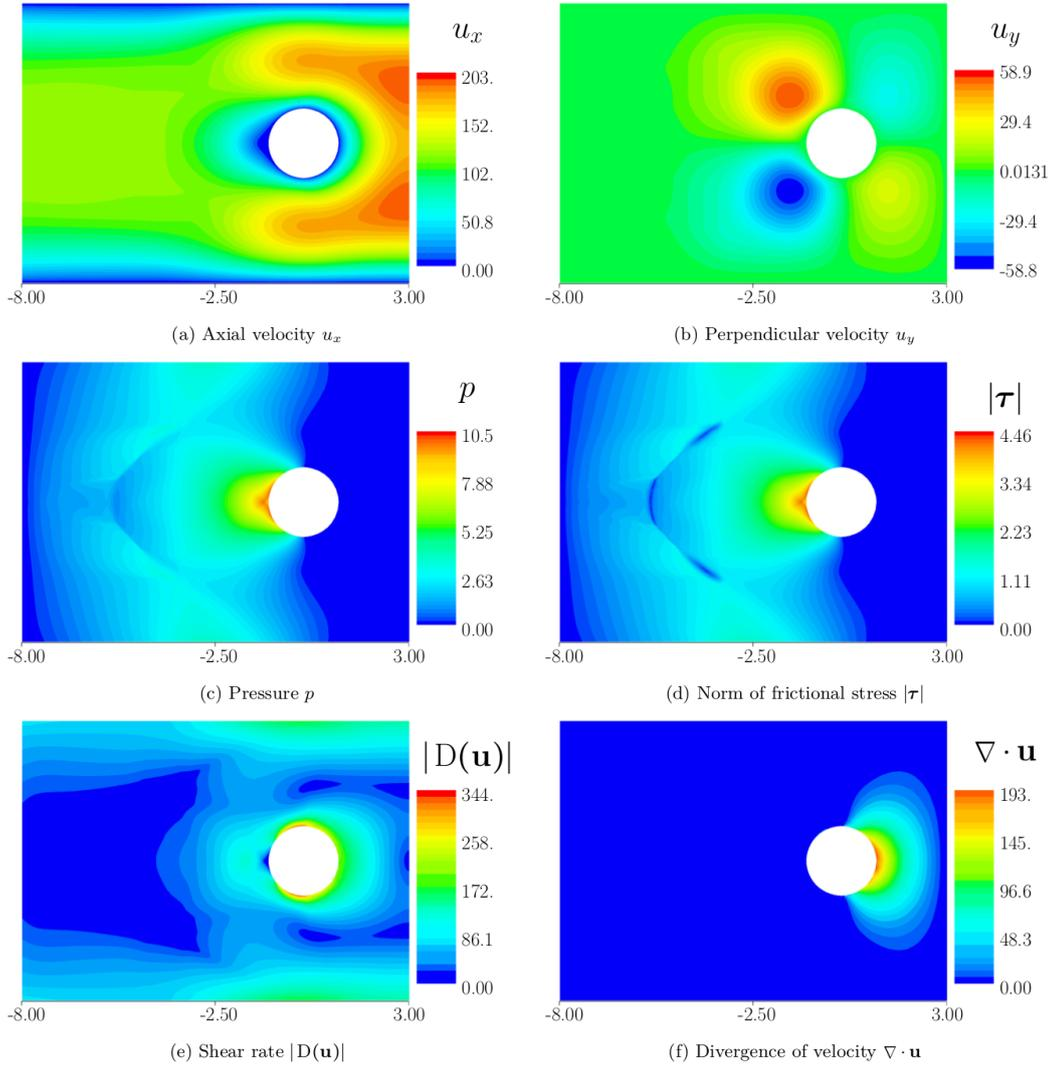
Figure 3.10 – Simulation of a granular flow with our nonsmooth numerical method, with  $\hat{\mu} = 0.3$ . The velocity and stress fields are shown in the case where the granular flows from left to right in a narrow channel, around a cylindrical obstacle.
