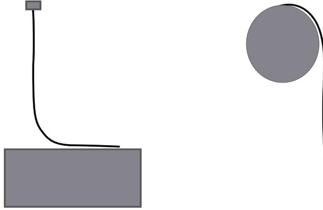
Figure 4.9 – Two examples of input configurations  $\mathbf{q}$  that should, intuitively, be accounted for by contact forces and not just by the intrinsic shape  $\bar{\mathbf{q}}$  of the rods.
