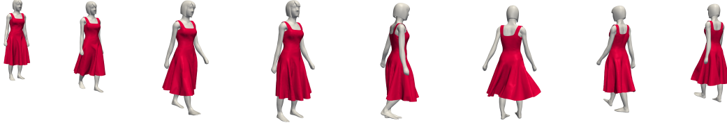
Figure 3.9 – Our body-cloth contact solver captures exact Coulomb friction both efficiently and robustly. On this dress example featuring 6000 cloth vertices and 1000 contact points on average, our solver converges at each time step ( dt = 1\text{ms} ) in a few hundred milliseconds..
