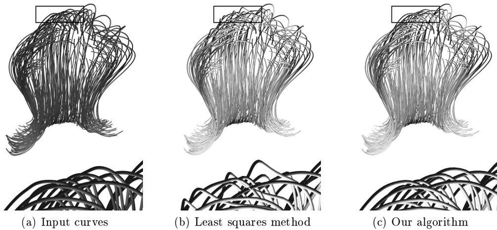
Figure 4.7 – Comparison of helical approximations (with  $N = 15$  elements) on a input curve dataset (a), between least-squares optimization (b) and our floating tangents algorithm (c). Our method proves not only more accurate, but also faster ( $10\times$  on this example) than least-squares optimization.
