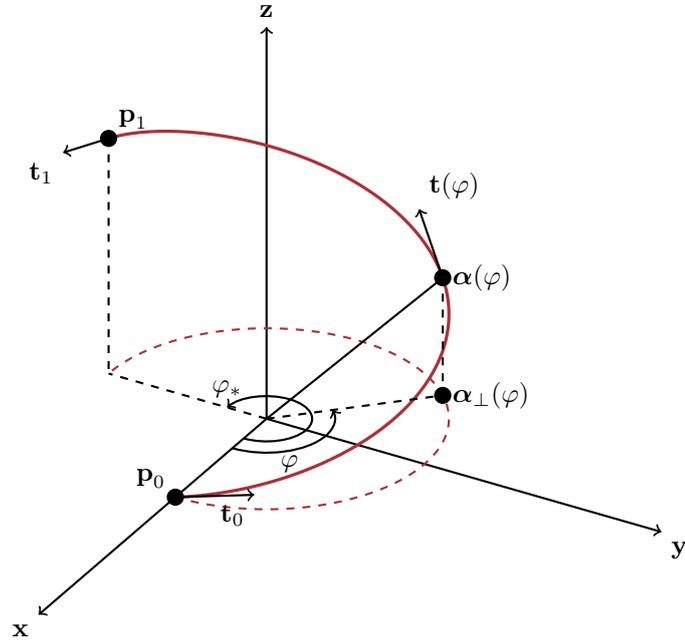
Figure 4.6 – In red, the unique short helix that interpolates  $\mathbf{p}_0$  and  $\mathbf{p}_1$  with tangents  $\mathbf{t}_0$  and  $\mathbf{t}_1$  when Equation (4.7) is satisfied. The helix is said to be short if  $\varphi^* \leq 2\pi$ .
