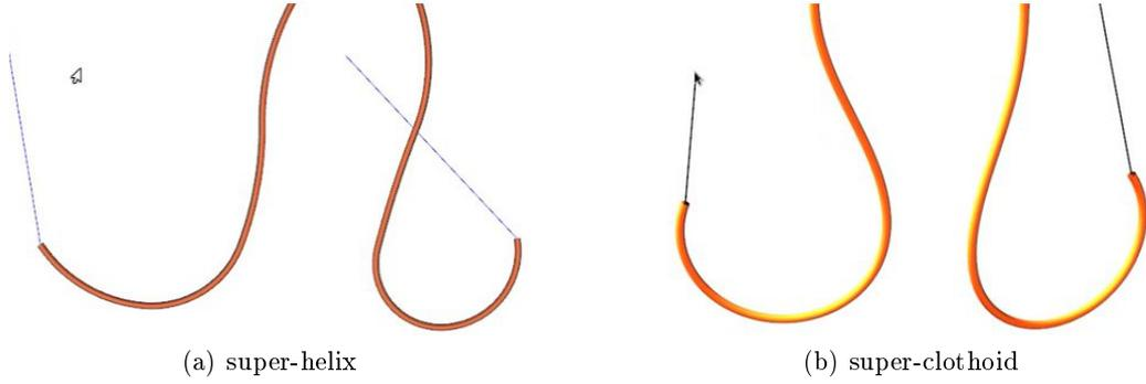
Figure 2.2 – Comparison of *fairness* (or smoothness) between (a) the super-helix model and (b) the super-clothoid model. Whereas joints between elements are particularly visible for the super-helix model (5 elements here), the super-clothoid model generates a smooth, visually pleasing shape even at a very coarse resolution (2 elements here).
