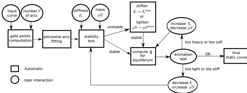
Figure 4.5 – Our inverse design process for an isolated fiber.
