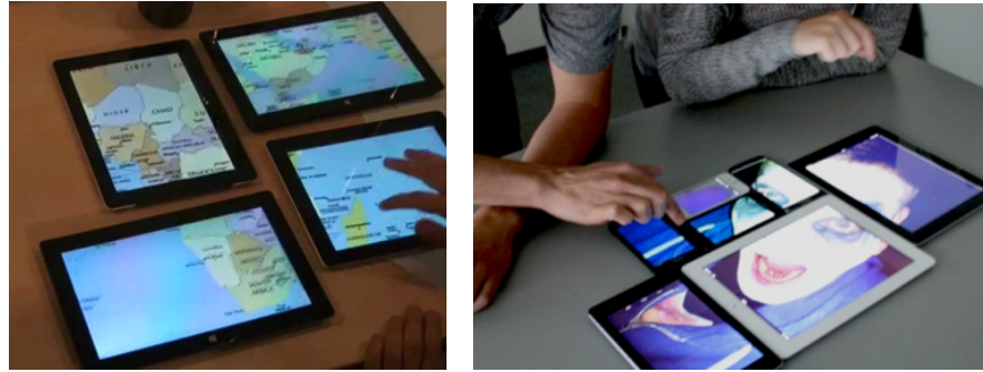
Figure 16: Two examples of combining personal devices to form a large tiled displays. Left: HuddleLamp [122]. Right: JuxtaPinch [102]
