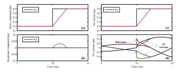
Figure IV-27: Proposed controllers dynamics with 2 ms sampling period: (a) direct component for AC currents, (b) quadrature component for AC currents, (c) DC current, (d) three phase AC currents.
