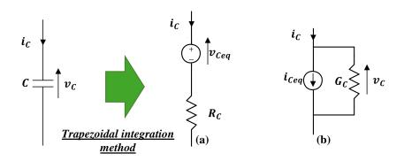
Figure II-10: Capacitor equivalent circuit: (a) resistive, (b) conductance.
