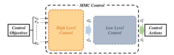
Figure III-1: General scheme of MMC control.
