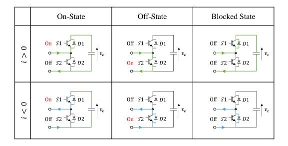
Figure I-17: Different states for Half-Bridge SM.
