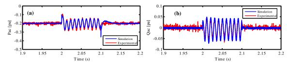
Figure V-19: Experimental results for symmetric AC voltage dip (50%): (a) active and reactive powers, (b) DC voltage with DC current, (c) AC current, (d) AC voltage, (e) upper average SM voltages, (f) lower average SM voltages
