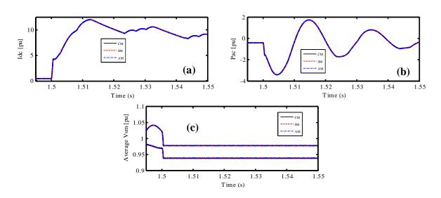
Figure A-11: Dynamics response of averaged models for a pole-to-pole DC fault: (a) DC current, (b) active power, (c) average SM voltages for upper and lower arms for phase a.
