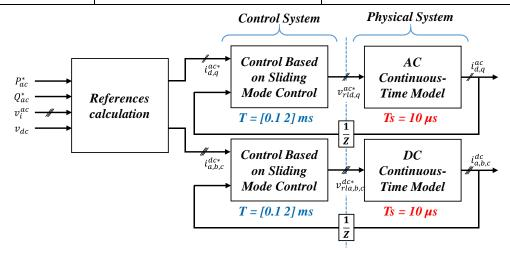
Figure IV-7: Simulation circuit for sliding mode control validation.
