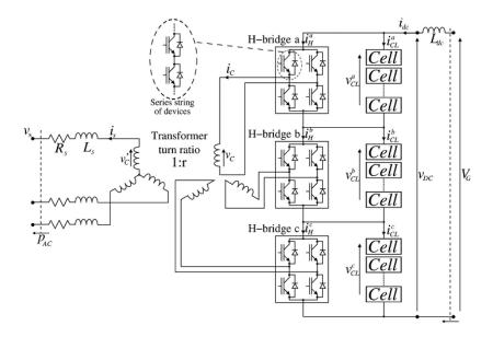
Figure I-23: Series bridge converter (SBC) [35].
