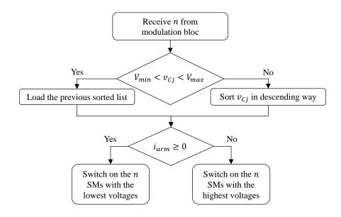
Figure III-15: Cell tolerance band algorithm flowchart.
