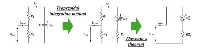
Figure II-11: From detailed to equivalent model.
