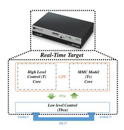
Figure V-3: Zoom on the HIL configuration.
