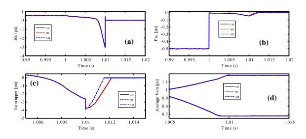
Figure A-10: Dynamics response of averaged models for a three phase AC fault: (a) DC current, (b) active power, (c) upper arm current for phase (a), (d) average SM voltages for upper and lower arms for phase a.
