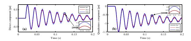
Figure IV-22: AC discrete-time models dynamics with 50  $\mu$ s: (a)  $i_q^{ac}$ , (b)  $i_q^{ac}$  variations.
