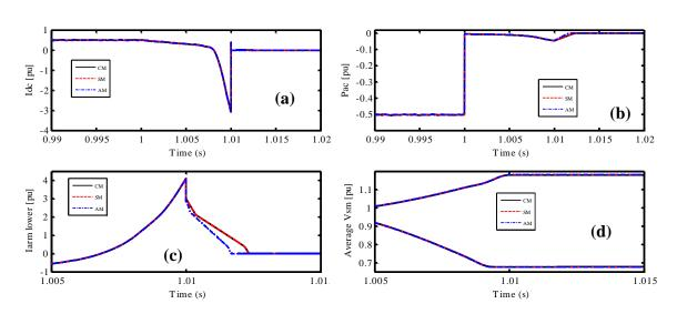
Figure A-3: Dynamics response of equivalent models for a three phase AC fault: (a) DC current, (b) active power, (c) lower arm current for phase (a), (d) average SM voltages for upper and lower arms for phase a.
