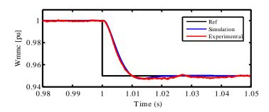
Figure V-15: Comparison between simulation and experimental results for energy step change with AC control strategy ( $\alpha_w = 0$ ).
