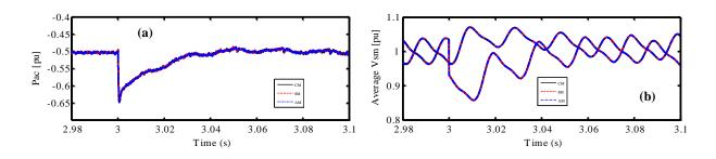
Figure A-6: Dynamics response of equivalent models for a loss of 10% SMs in one arm: (a) active power, (b) average SM voltages for upper and lower arms for phase a.
