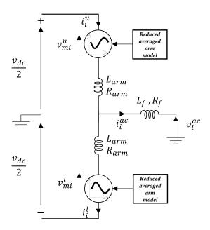
Figure III-24: Simplified circuit for one MMC leg.
