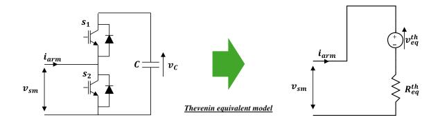
Figure II-3: Equivalent Thevenin model for one SM.
