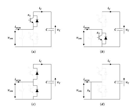
Figure II-16: SM Configurations including blocked and fault states.
