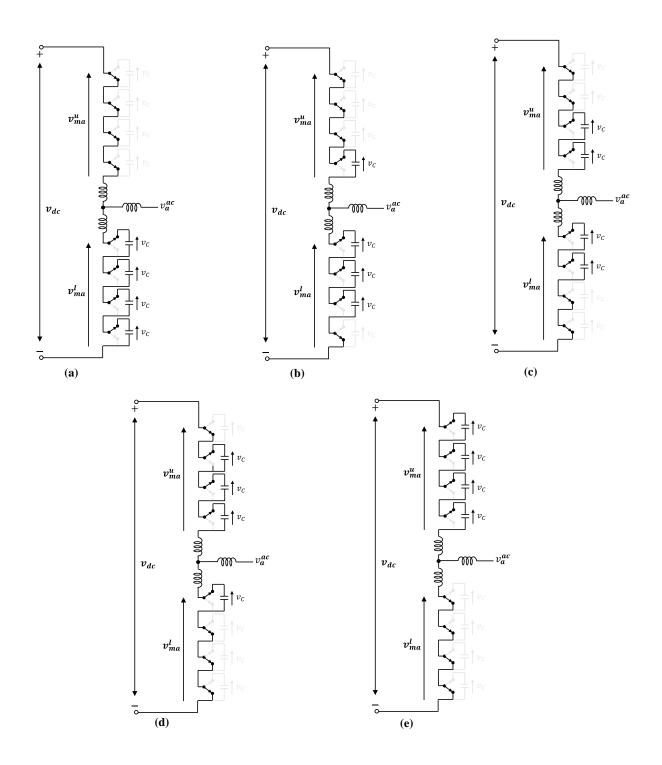
Figure I-16: Operation principle of 5-level MMC.
