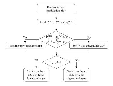
Figure III-14: Average tolerance band algorithm flowchart.
