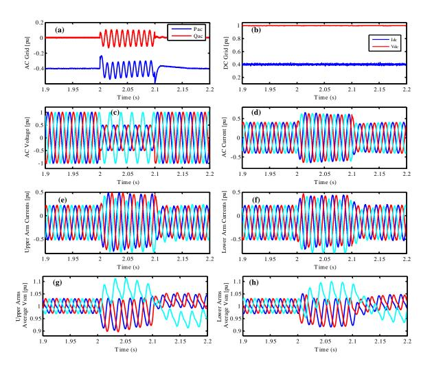
Figure A-27: Simulation results for asymmetrical AC voltage dip with 0.2 ms sampling period: (a) active and reactive power, (b) DC current with DC voltage, (c) AC voltages, (d) AC currents, (e) upper arm currents, (f) lower arm currents, (g) average SM voltages for upper arms, (h) average SM voltages for lower arms
