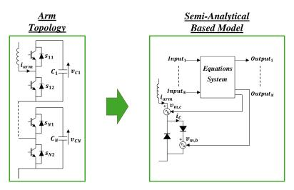
Figure II-17: Semi-analytical model proposed in [61].
