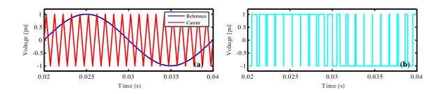
Figure I-13: (a) Requested AC voltage, (b) generated AC voltage with VSC.
