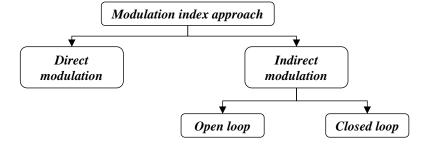
Figure III-4: Modulation index classification.
