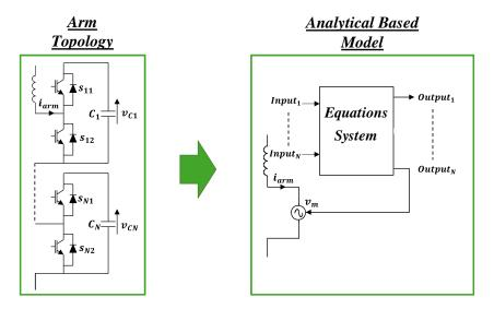
Figure II-22: Proposed analytical model.
