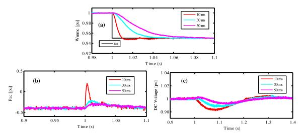
Figure V-13: Experimental results for energy step change with AC control strategy( $\alpha_W = 0$ ): (a) MMC energy, (b) active power, (c) DC voltage.
