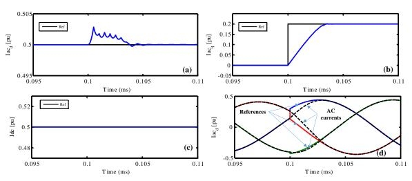
Figure IV-17: Simulation results for reactive power reference change with T=0.5 ms  $(k_i^{ac} = k_i^{dc} = 10000, \ \sigma = 50, \ k_p^{ac} = k_p^{dc} = 3200)$ : (a) direct component for AC currents, (b) quadrature component for AC currents, (c) DC current, (d) three phase AC currents.
