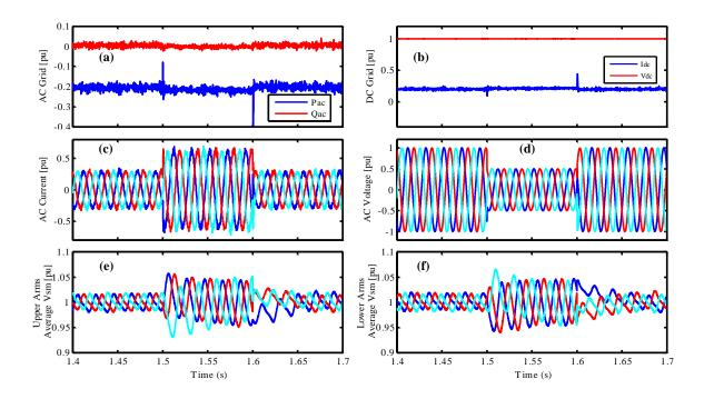
Figure V-16: Experimental results for symmetric AC voltage dip (50%): (a) active and reactive powers, (b) DC voltage with DC current, (c) AC current, (d) AC voltage, (e) upper average SM voltages, (f) lower average SM voltages.
