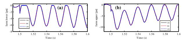
Figure A-12: Arm currents dynamics of averaged models for a pole-to-pole DC fault.
