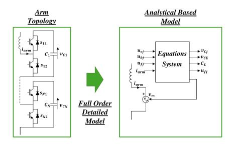
Figure II-23: Full order detailed model based on analytical modeling technique.
