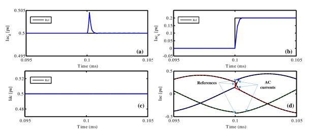
Figure IV-15: Simulation results for reactive power reference change ( $k_i^{ac} = k_i^{dc} = 10000$ ,  $\sigma = 50$ ,  $k_p^{ac} = k_p^{dc} = 3200$ ): (a) direct component for AC currents, (b) quadrature component for AC currents, (c) DC current, (d) three phase AC currents.
