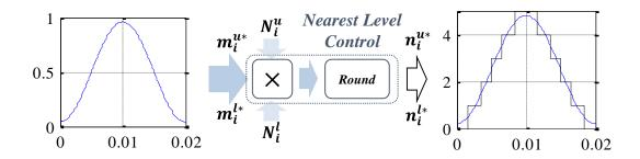
Figure III-7: Nearest level modulation scheme.
