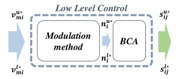
Figure III-2: Architecture of low level control.
