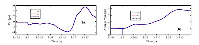
Figure A-7: Dynamics response of equivalent models for a loss of one arm: (a) active power, (b) average SM voltages for upper and lower arms for phase a.
