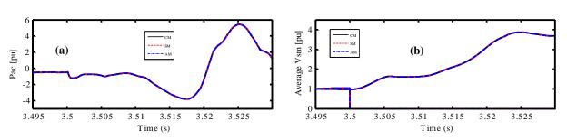
Figure A-14: Dynamics response of averaged models for a loss of one arm: (a) active power, (b) average SM voltages for upper and lower arms for phase a.
