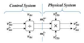
Figure III-34: Direct modulation indexes calculation.
