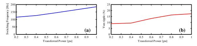
Figure III-23: (a) Switching frequency, (b) voltage ripple variations regarding transferred power level using ATB algorithm.
