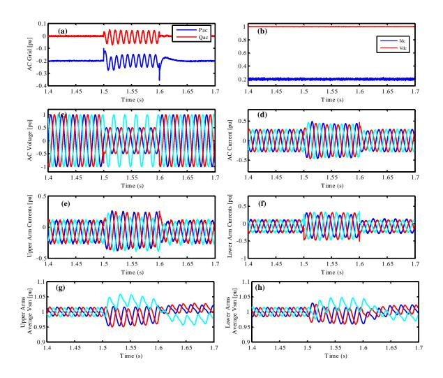
Figure IV-39: Simulation results for Asymmetrical AC voltage dip with 0.2 ms sampling period: (a) Active and reactive power, (b) DC current with DC voltage, (c) AC voltages, (d) AC currents, (e) Upper arm currents, (f) lower arm currents, (g) Average SM voltages for upper arms, (h) Average SM voltages for lower arms.
