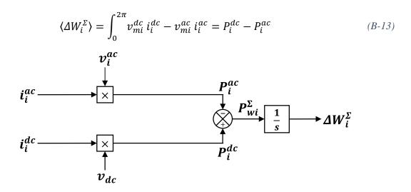
Figure A-19: Block diagram of energy leg (sum) equivalent model.
