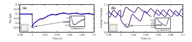
Figure II-37: Dynamics response of detailed models for a loss of 10% SMs in one arm: (a) active power, (b) average SM voltages for upper and lower arms for phase a.
