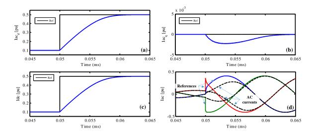
Figure IV-10: Simulation results for active power reference change  $(k_i^{ac} = k_i^{dc} = 10000, \sigma = 50)$ : (a) direct component for AC currents, (b) quadrature component for AC currents, (c) DC current, (d) three phase AC currents.
