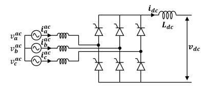
Figure I-8: Three phase Line-Commuted Converter (LCC).
