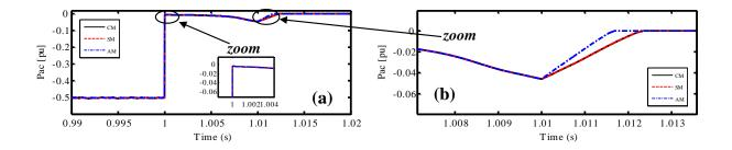
Figure II-29: Active power dynamics of detailed models for a three phase AC fault.
