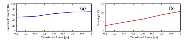
Figure III-21: (a) Switching frequency, (b) voltage ripple variations regarding transferred power level using IRSF algorithm.
