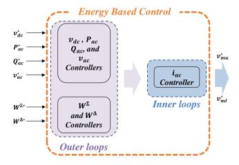
Figure III-36: Energy based control diagram (first version).
