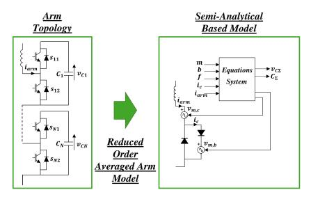
Figure II-21: Reduced order averaged arm model based on semi-analytical modeling technique.
