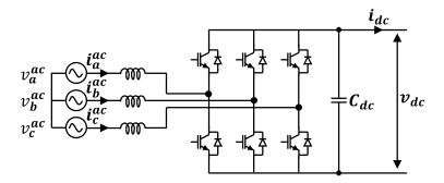
Figure I-12: Three-phase 2-level Voltage Souce Converter (VSC).
