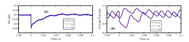
Figure A-13: Dynamics response of averaged models for a loss of 10% SMs in one arm: (a) active power, (b) average SM voltages for upper and lower arms for phase a.
