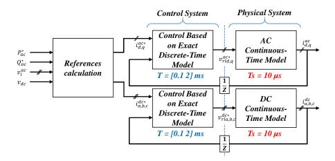
Figure IV-25: Simulation circuit for discrete-time controller validation.
