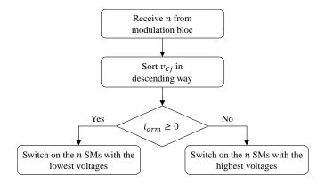
Figure III-8: Basic BCA flowchart.
