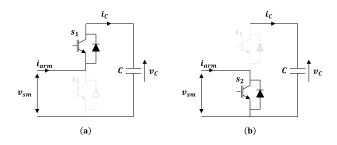
Figure II-9: SM configurations for controlled states.
