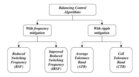
Figure III-11: Balancing control algorithms classification.
