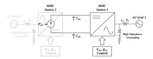
Figure II-26: Simulation circuit for models validation.
