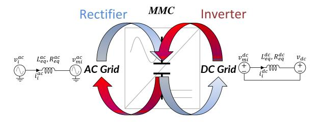
Figure III-28: Power exchange inside the MMC.
