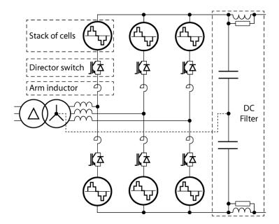
Figure I-22: Alternative Arm Converter (AAC) [34].
