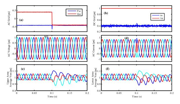
Figure V-7: HIL simulation results for reactive power step change: (a) active and reactive powers, (b) DC voltage with DC current, (c) AC voltage, (d) AC current, (e) upper average SM voltages, (f) lower average SM voltages.
