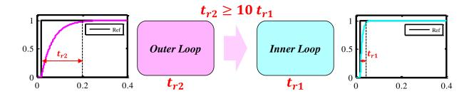
Figure III-31: Cascaded control principle.
