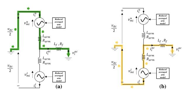
Figure III-25: Upper and lower voltage loops.
