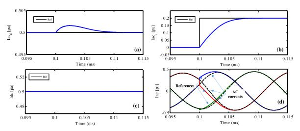
Figure IV-11: Simulation results for reactive power reference change ( $k_i^{ac} = k_i^{dc} = 10000$ ,  $\sigma = 50$ ): (a) direct component for AC currents, (b) quadrature component for AC currents, (c) DC current, (d) three phase AC currents.
