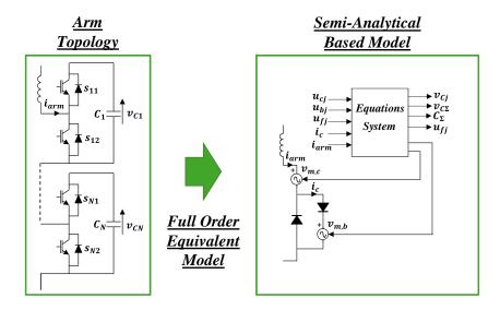
Figure II-20: Full order equivalent model based on semi-analytical modeling technique.
