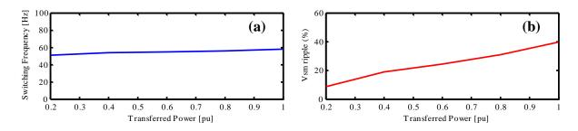
Figure III-19: (a) Switching frequency, (b) voltage ripple variations regarding transferred power level using RSF-algorithm.
