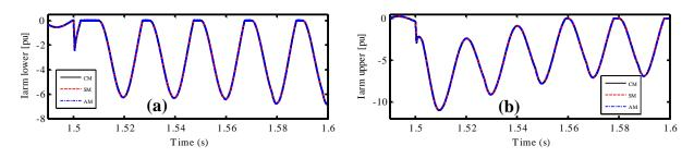
Figure A-5: Arm currents dynamics of equivalent models for a pole-to-pole DC fault.
