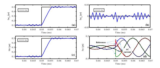
Figure IV-18: Simulation results for active power reference change with T=1 ms ( $k_i^{ac}=k_i^{dc}=10000$ ,  $\sigma=50$ ,  $k_p^{ac}=k_p^{dc}=3200$ ): (a) direct component for AC currents, (b) quadrature component for AC currents, (c) DC current, (d) three phase AC currents.
