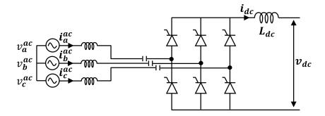
Figure I-11: Three phase Capacitor-Commutated Converter (CCC)
