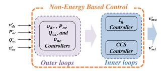
Figure III-35: Non energy based control diagram including CCSC.
