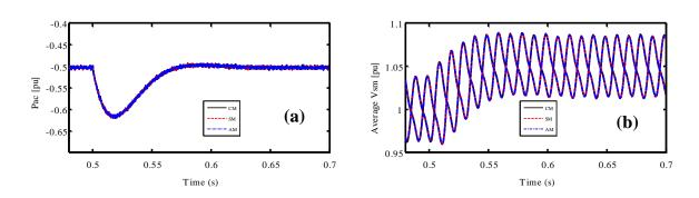
Figure A-9: Dynamics response of averaged models for a stored energy step change: (a) active power, (b) average SM voltages for upper and lower arms for phase a.
