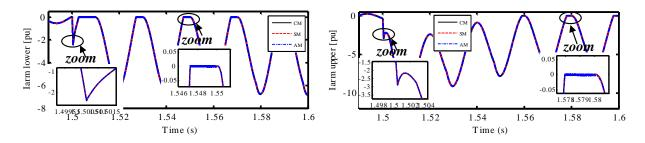
Figure II-36: Arm currents dynamics of detailed models for a pole-to-pole DC fault (phase a).
