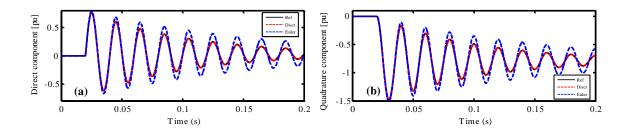
Figure IV-23: AC discrete-time models dynamics with 100  $\mu$ s: (a)  $i_q^{ac}$ , (b)  $i_q^{ac}$  variations.
