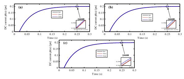
Figure IV-24: DC discrete-time models dynamics:  $i_a^{dc}$  variation with (a) 10  $\mu$ s, (b) 50  $\mu$ s and (c) 100  $\mu$ s.
