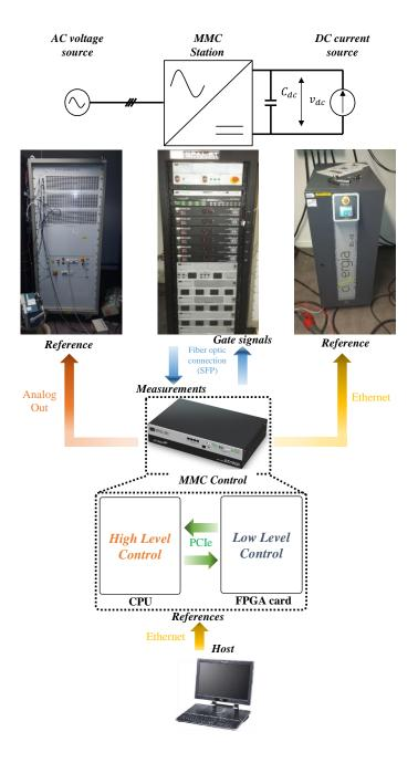
Figure V-9: Experimental test bench setup.
