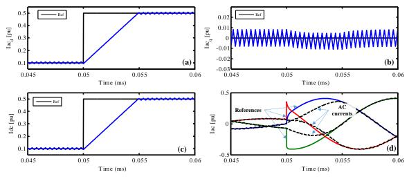
Figure IV-8: Simulation results for active power reference change  $(k_i^{ac} = k_i^{dc} = 10000)$ : (a) direct component for AC currents, (b) quadrature component for AC currents, (c) DC current, (d) three phase AC currents.
