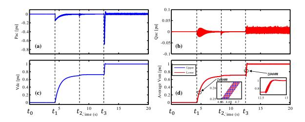
Figure V-4: HIL results for start-up sequence: (a) active power, (b) reactive power, (c) DC grid voltage, (d) average SM voltages for leg (a).
