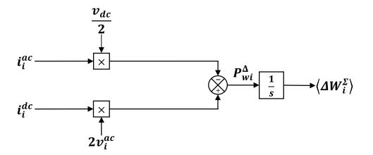
Figure A-21: Block diagram of energy difference equivalent model.
