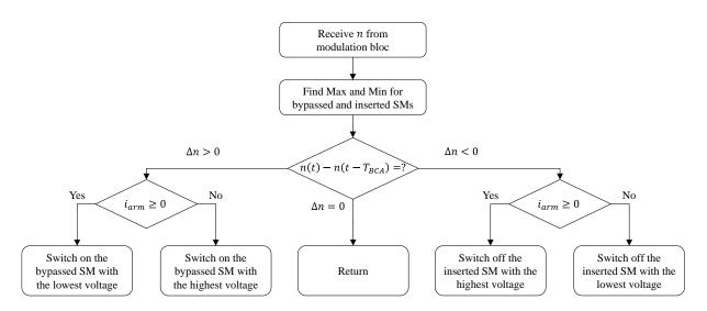
Figure III-12: Reduced switching frequency algorithm flowchart.
