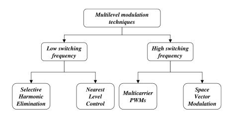
Figure III-5: Multilevel modulation classification.
