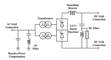
Figure I-10: LCC-HVDC station.
