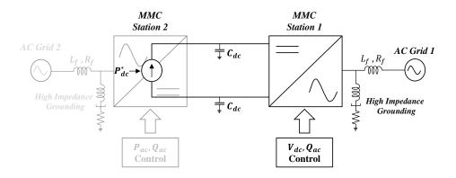
Figure IV-31: Simulation circuit for offline control validation.
