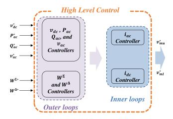
Figure III-37: Energy based control diagram (second version).
