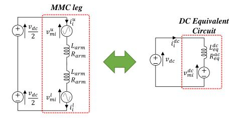
Figure III-27: MMC equivalent circuit from DC standpoint.
