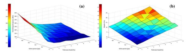
Figure IV-2: (a) Switching frequency, (b) voltage ripple variations regarding transferred power and tolerance band parameter.
