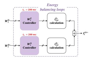
Figure III-41: Zoom on energy balancing loops configuration.
