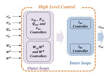
Figure III-32: Cascaded control scheme for MMC.
