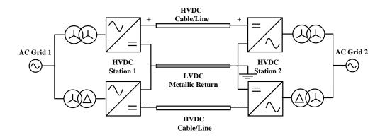
Figure I-7: Bipolar scheme with metallic return.
