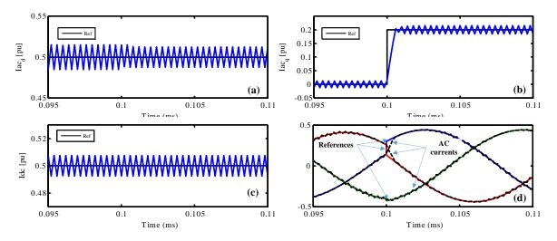
Figure IV-13: Simulation results for reactive power reference change ( $k_i^{ac} = k_i^{dc} = 30000$ ,  $\sigma = 50$ ): (a) direct component for AC currents, (b) quadrature component for AC currents, (c) DC current, (d) three phase AC currents.
