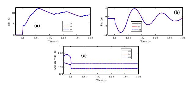
Figure A-4: Dynamics response of equivalent models for a pole-to-pole DC fault: (a) DC current, (b) active power, (c) average SM voltages for upper and lower arms for phase a.
