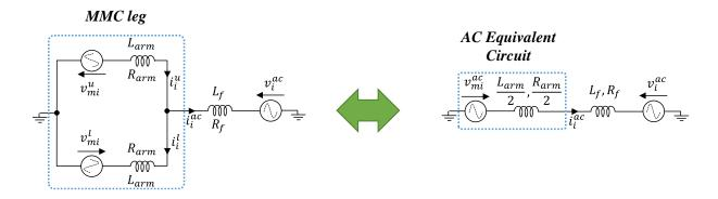
Figure III-26: MMC equivalent circuit from AC standpoint.
