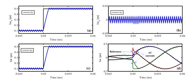
Figure IV-12: Simulation results for active power reference change  $(k_i^{ac} = k_i^{dc} = 30000, \sigma = 50)$ : (a) direct component for AC currents, (b) quadrature component for AC currents, (c) DC current, (d) three phase AC currents.
