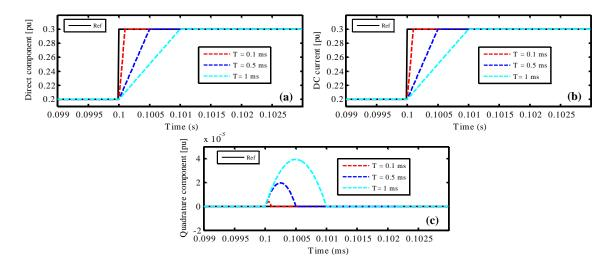
Figure IV-28: Proposed controllers dynamics with different sampling periods: (a) direct component for AC currents, (b) DC current, (c) quadrature component for AC currents.
