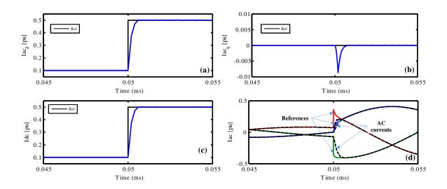
Figure IV-14: Simulation results for active power reference change  $(k_i^{ac} = k_i^{dc} = 10000, \sigma = 50, k_p^{ac} = k_p^{dc} = 3200)$ : (a) direct component for AC currents, (b) quadrature component for AC currents, (c) DC current, (d) three phase AC currents.
