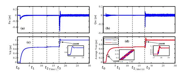
Figure V-10: Experimental results for start-up sequence: (a) Active power, (b) reactive power, (c) DC grid voltage, (d) average SM voltages for leg (a).
