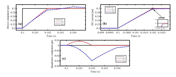
Figure IV-30: Discrete-time controllers performances with 2 ms sampling period: (a) direct component for AC currents, (b) DC current, (c) quadrature component for AC currents.
