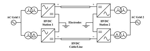
Figure I-6: Bipolar scheme without metallic return.
