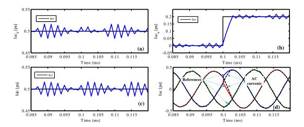
Figure IV-19: Simulation results for reactive power reference change with T=1 ms ( $k_i^{ac}=k_i^{dc}=10000$ ,  $\sigma=50$ ,  $k_p^{ac}=k_p^{dc}=3200$ ): (a) direct component for AC currents, (b) quadrature component for AC currents, (c) DC current, (d) three phase AC currents.
