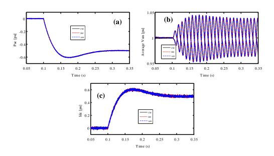
Figure A-1: Dynamics response of equivalent models for a DC power step change: (a) active power, (b) average SM voltages for upper and lower arms for phase a, (c) DC current.
