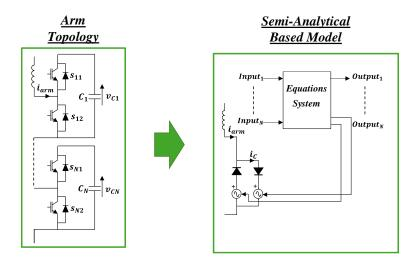
Figure II-18: Semi-analytical model proposed in [64]
