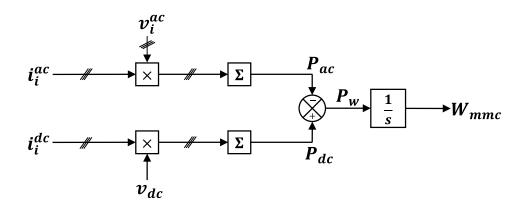
Figure A-17: Block diagram for MMC energy equivalent model.
