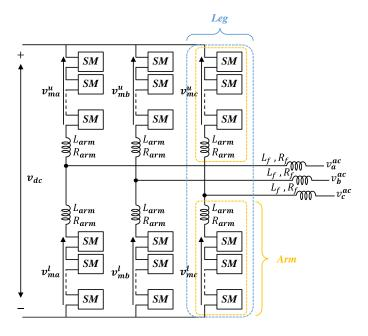
Figure I-15: Three-phase Modular Multilevel Converter (MMC).
