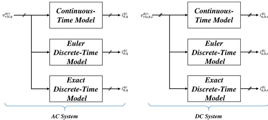
Figure IV-20: Simulation circuit for discrete-time models validation.
