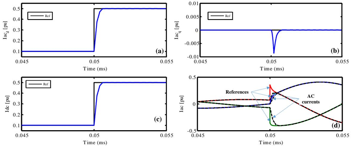
Figure IV-14: Simulation results for active power reference change ( $k_i^{ac}=k_i^{dc}=10000$ ,  $\sigma=50$ ,  $k_p^{ac}=k_p^{dc}=3200$ ): (a) direct component for AC currents, (b) quadrature component for AC currents, (c) DC current, (d) three phase AC currents.
