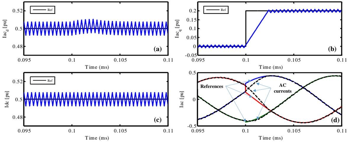
Figure IV-9: Simulation results for reactive power reference change ( $k_i^{ac}=k_i^{dc}=10000$ ): (a) direct component for AC currents, (b) quadrature component for AC currents, (c) DC current, (d) three phase AC currents.
