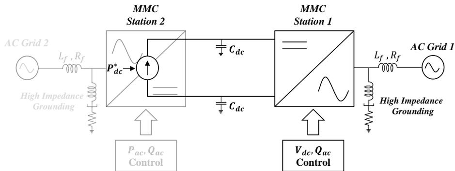
Figure IV-31: Simulation circuit for offline control validation.
