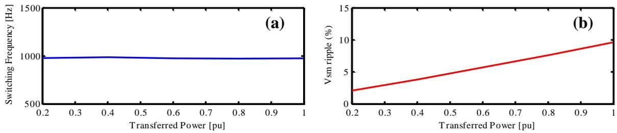
Figure III-17: (a) Switching frequency, (b) voltage ripple variations regarding transferred power level using Basic BCA.
