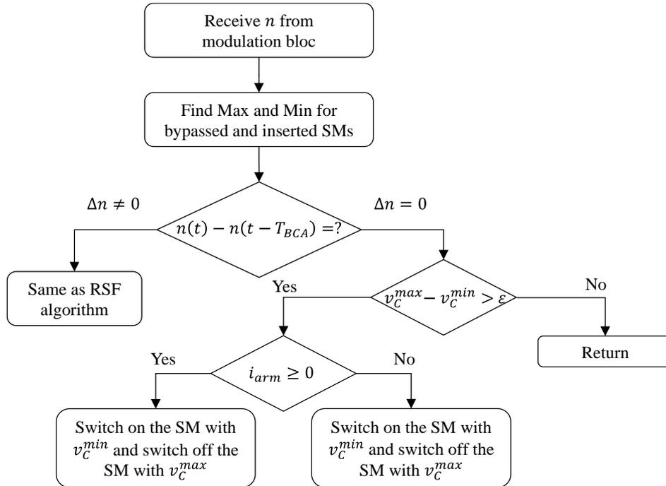
Figure III-13: Improved reduced switching frequency algorithm flowchart.
