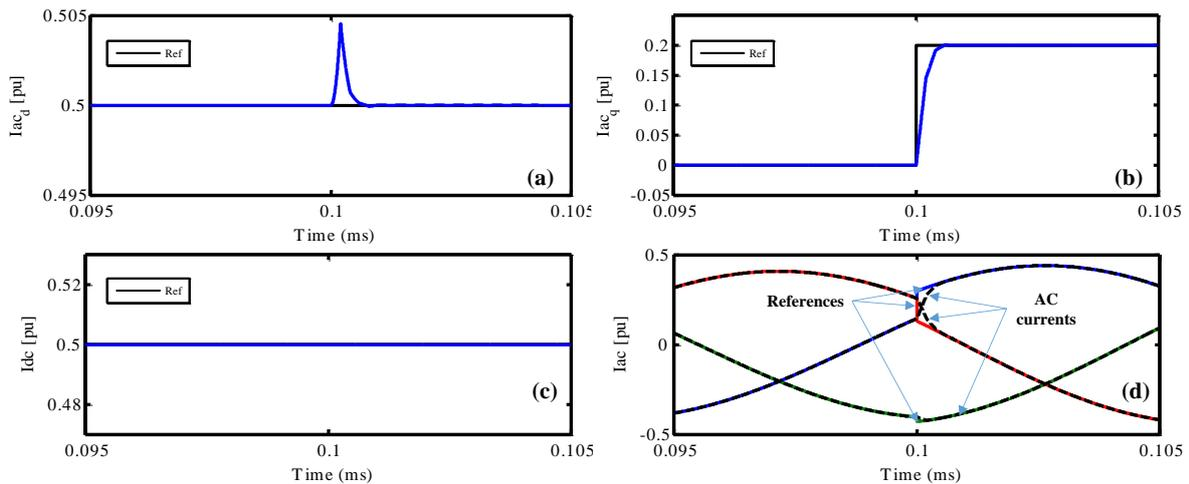
Figure IV-15: Simulation results for reactive power reference change ( $k_i^{ac}=k_i^{dc}=10000$ ,  $\sigma=50$ ,  $k_p^{ac}=k_p^{dc}=3200$ ): (a) direct component for AC currents, (b) quadrature component for AC currents, (c) DC current, (d) three phase AC currents.
