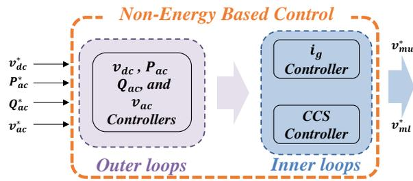
Figure III-35: Non energy based control diagram including CCSC.
