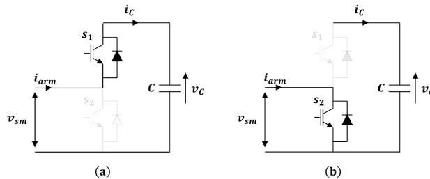
Figure II-9: SM configurations for controlled states.
