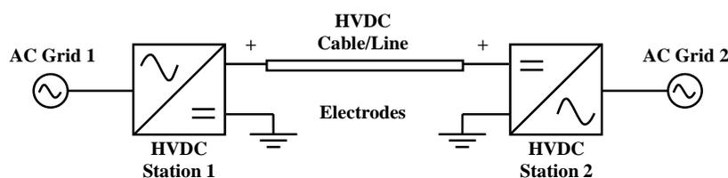
Figure I-3: Asymmetric monopolar scheme without metallic return.
