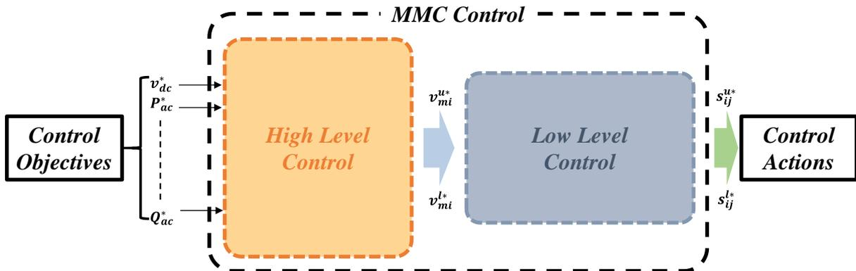
Figure III-1: General scheme of MMC control.
