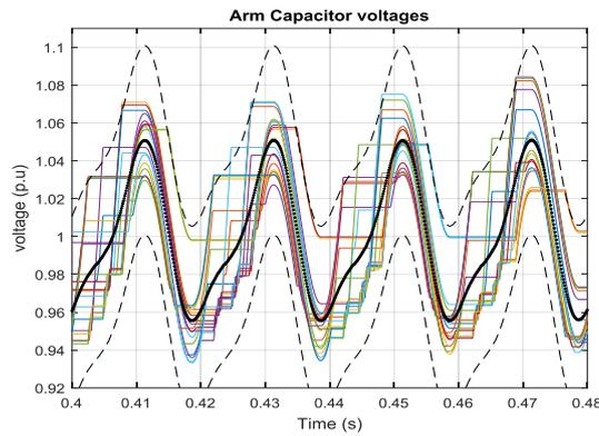
Figure IV-1: SM voltages variation using ATB algorithm.
