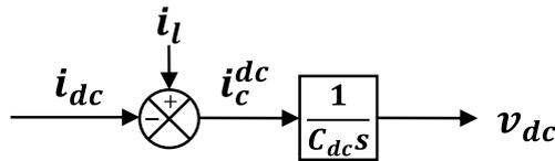
Figure A-15: Block diagram for DC voltage equivalent model.
