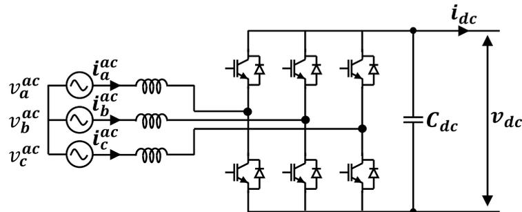
Figure I-12: Three-phase 2-level Voltage Source Converter (VSC).
