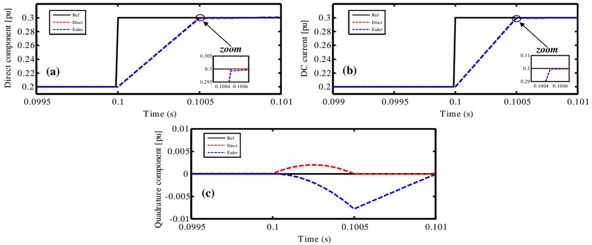
Figure IV-29: Discrete-time controllers performances with 0.5 ms sampling period: (a) direct component for AC currents, (b) DC current, (c) quadrature component for AC currents.
