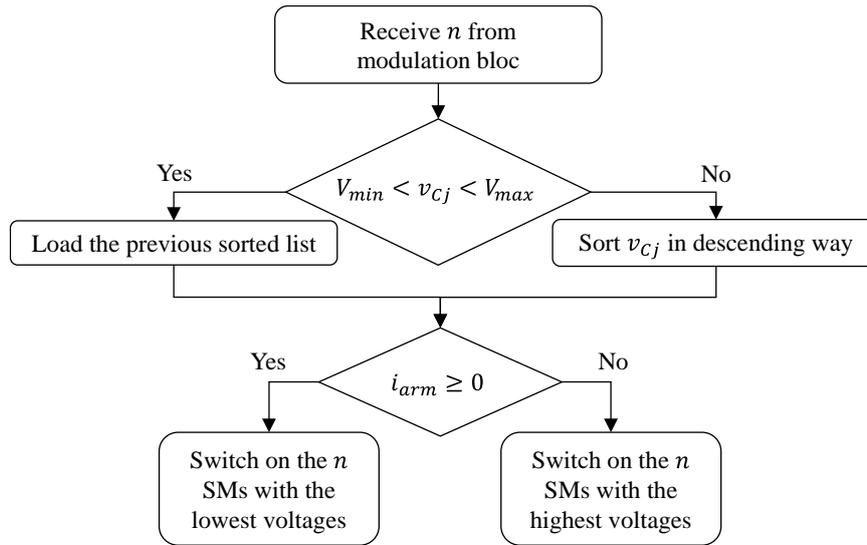
Figure III-15: Cell tolerance band algorithm flowchart.
