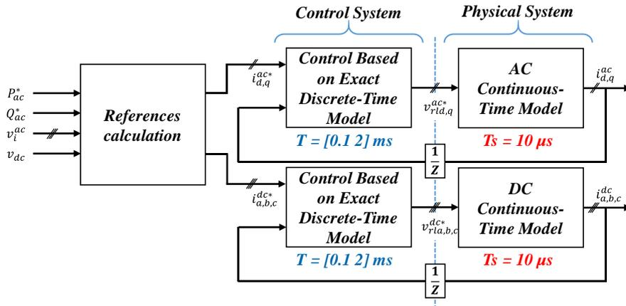
Figure IV-25: Simulation circuit for discrete-time controller validation.
