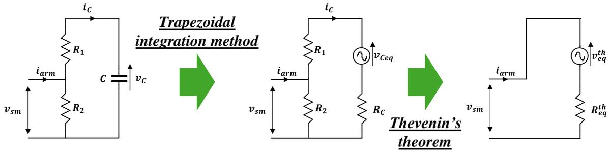
Figure II-11: From detailed to equivalent model.
