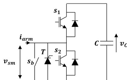
Figure I-18: Half-Bridge SM including protecting Thyristor and mechanical switch.
