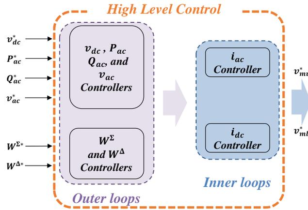
Figure III-37: Energy based control diagram (second version).
