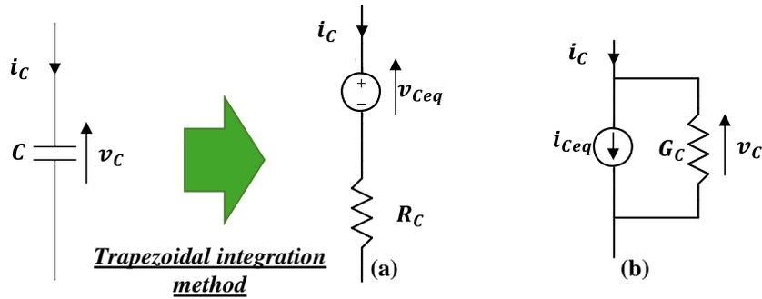
Figure II-10: Capacitor equivalent circuit: (a) resistive, (b) conductance.
