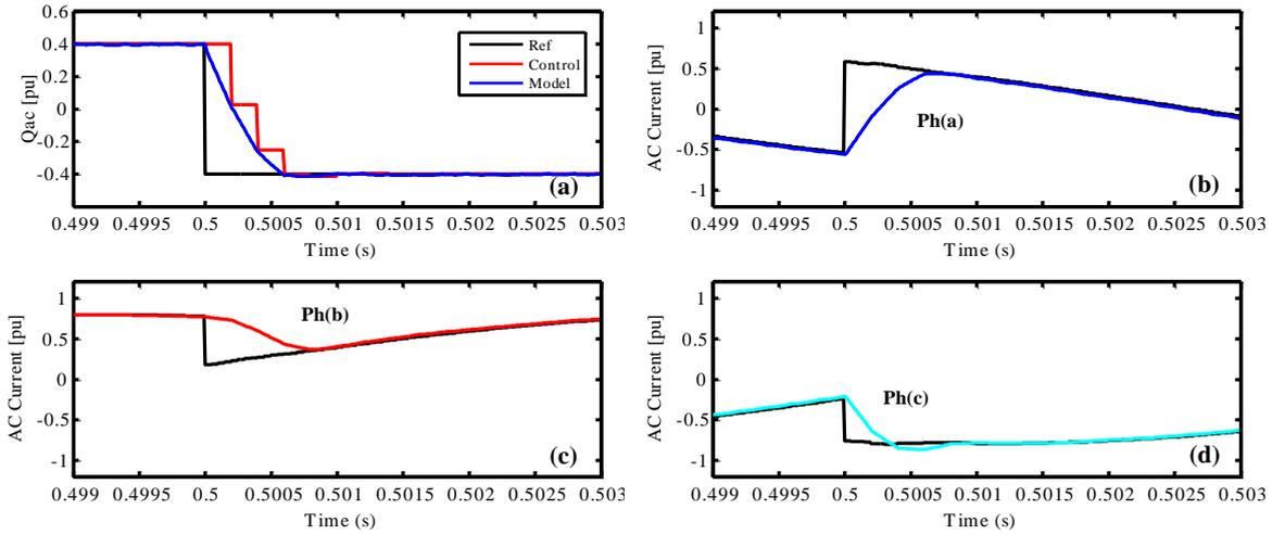
Figure IV-33 Zoom on simulation results with 0.2 ms sampling period: (a) reactive power, (b) AC current phase (a), (b) AC current phase (b), (b) AC current phase (c), (b) AC current phase (d).
