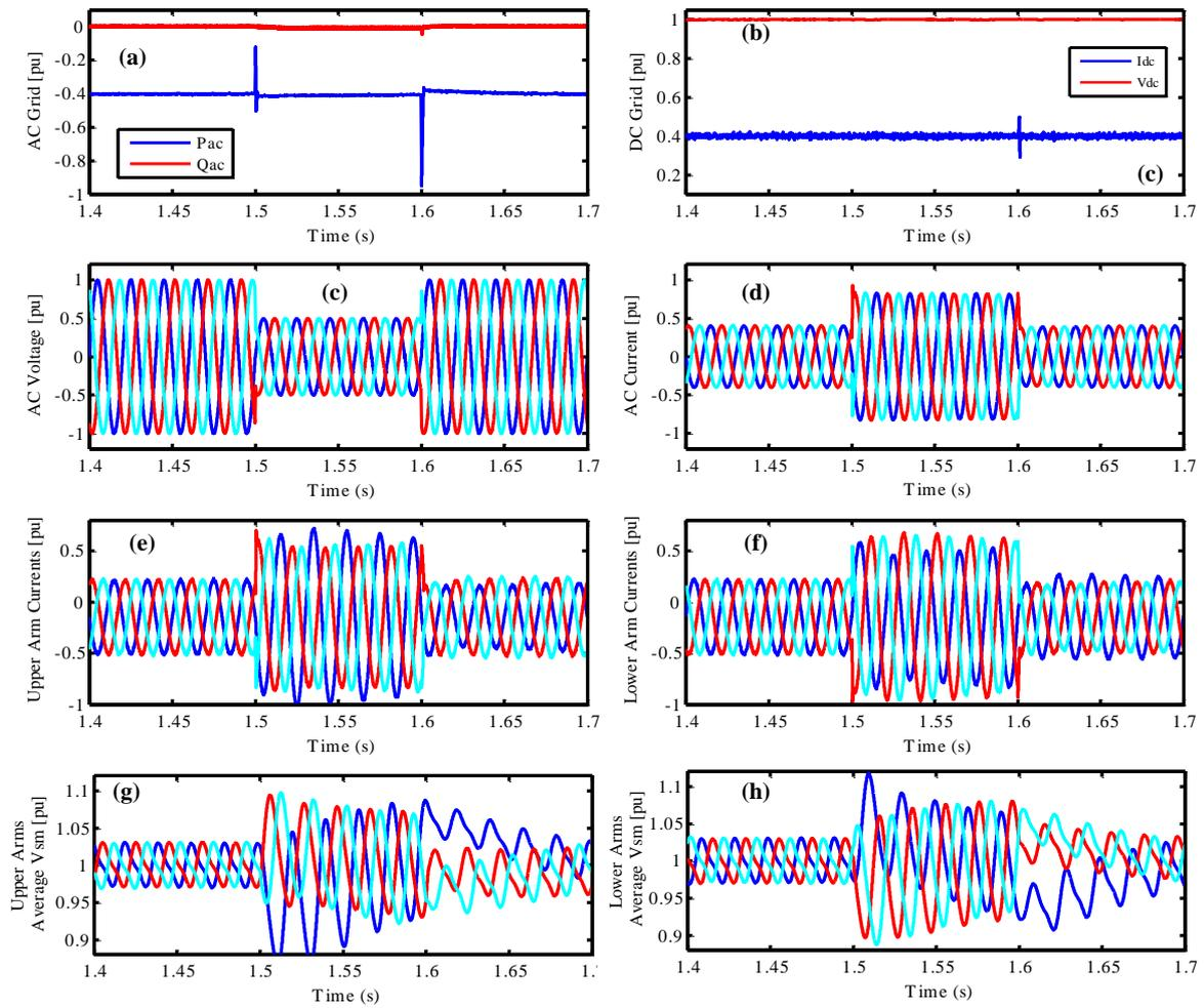
Figure A-26: Simulation results for symmetrical AC voltage dip with 0.2 ms sampling period: (a) active and reactive power, (b) DC current with DC voltage, (c) AC voltages, (d) AC currents, (e) upper arm currents, (f) lower arm currents, (g) average SM voltages for upper arms, (h) average SM voltages for lower arms.
