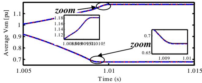
Figure II-32: Models dynamics of the detailed model for a three phase AC fault: average SMs voltages for upper and lower arm of phase a.
