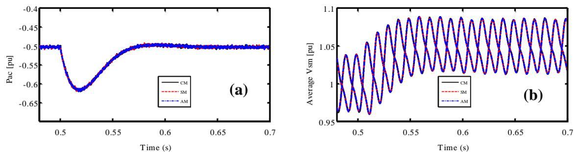
Figure A-9: Dynamics response of averaged models for a stored energy step change: (a) active power, (b) average SM voltages for upper and lower arms for phase a.
