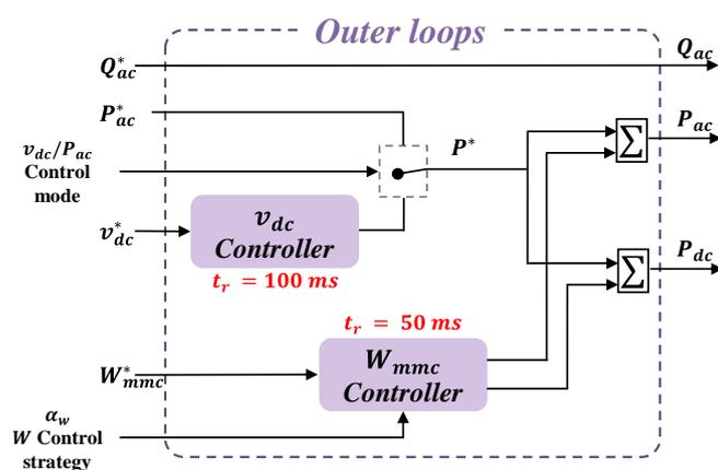
Figure III-40: Zoom on outer loops configuration.
