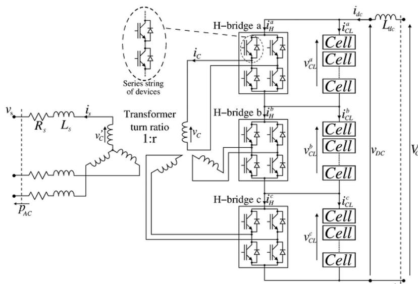
Figure I-23: Series bridge converter (SBC) [35].
