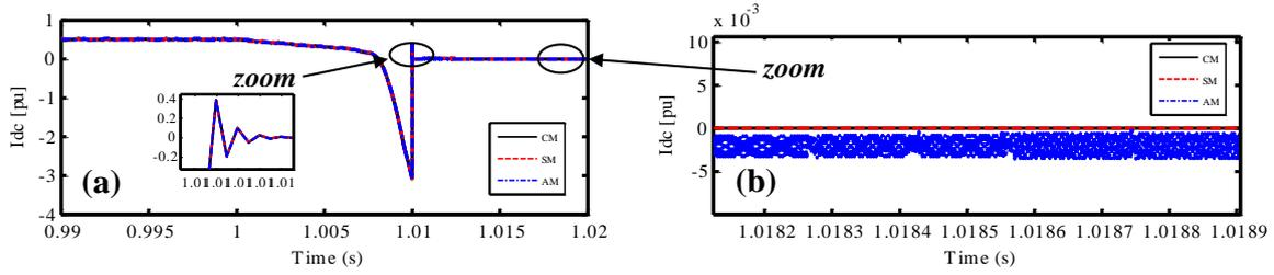
Figure II-31: DC current dynamics of detailed models for a three phase AC fault.
