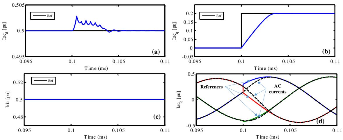
Figure IV-17: Simulation results for reactive power reference change with  $T=0.5$  ms ( $k_i^{ac}=k_i^{dc}=10000$ ,  $\sigma=50$ ,  $k_p^{ac}=k_p^{dc}=3200$ ): (a) direct component for AC currents, (b) quadrature component for AC currents, (c) DC current, (d) three phase AC currents.
