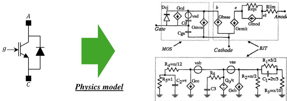
Figure II-1: Physics based model for IGBT [40].
