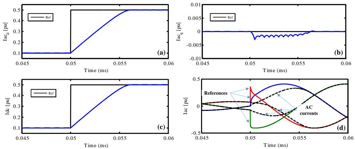
Figure IV-16: Simulation results for active power reference change with  $T=0.5$  ms ( $k_i^{ac}=k_i^{dc}=10000$ ,  $\sigma=50$ ,  $k_p^{ac}=k_p^{dc}=3200$ ): (a) direct component for AC currents, (b) quadrature component for AC currents, (c) DC current, (d) three phase AC currents.
