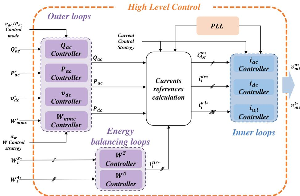
Figure III-39: Schematic diagram for the considered high level control for thesis contributions.
