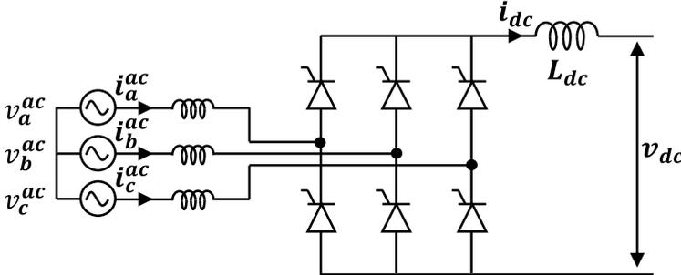
Figure I-8: Three phase Line-Commutated Converter (LCC).
