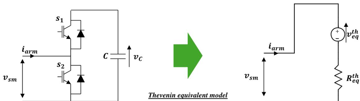
Figure II-3: Equivalent Thevenin model for one SM.
