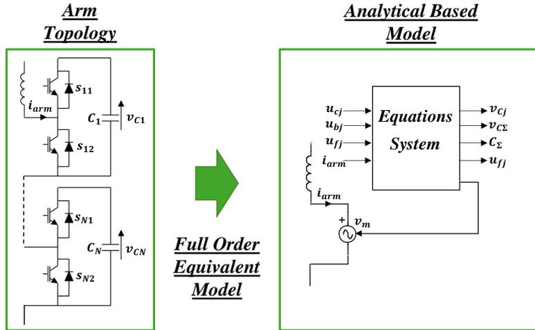
Figure II-24: Full order equivalent model based on analytical modeling technique.
