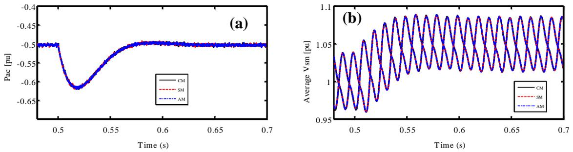
Figure A-2: Dynamics response of equivalent models for a stored energy step change: (a) active power, (b) average SM voltages for upper and lower arms for phase a.
