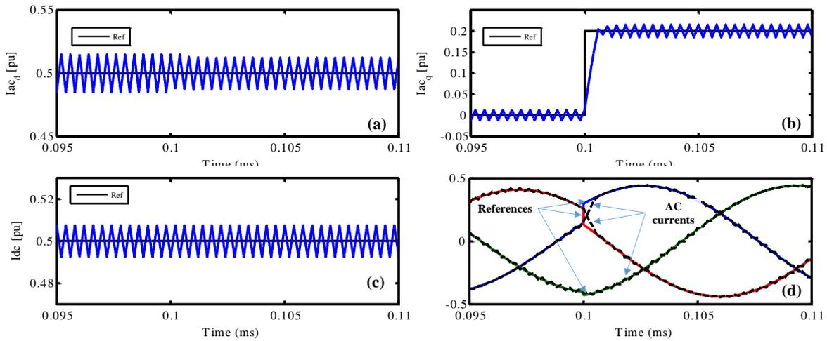
Figure IV-13: Simulation results for reactive power reference change ( $k_i^{ac}=k_i^{dc}=30000$ ,  $\sigma=50$ ): (a) direct component for AC currents, (b) quadrature component for AC currents, (c) DC current, (d) three phase AC currents.
