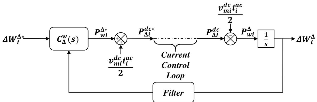
Figure A-22: Block diagram of energy difference control in closed loop.
