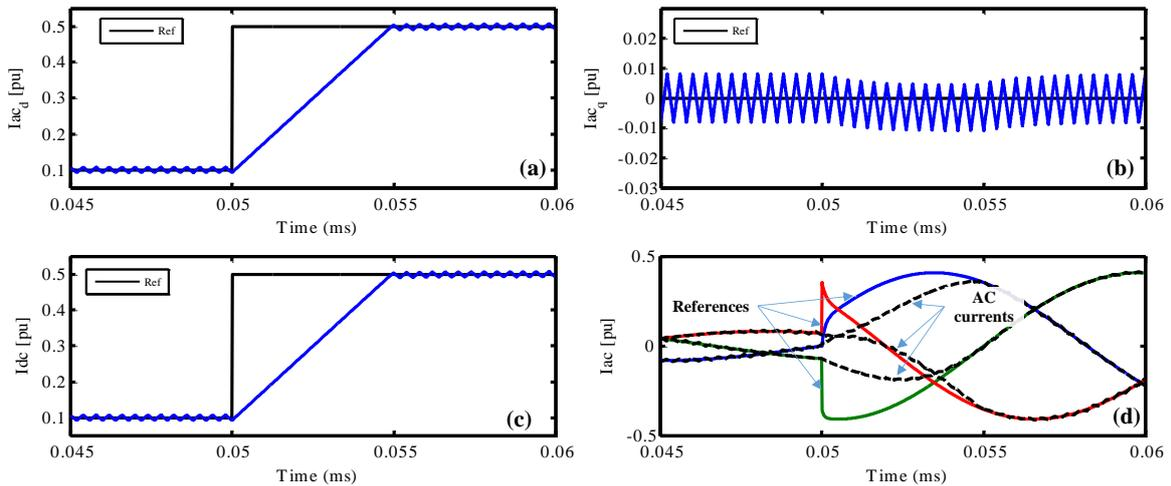
Figure IV-8: Simulation results for active power reference change ( $k_i^{ac}=k_i^{dc}=10000$ ): (a) direct component for AC currents, (b) quadrature component for AC currents, (c) DC current, (d) three phase AC currents.
