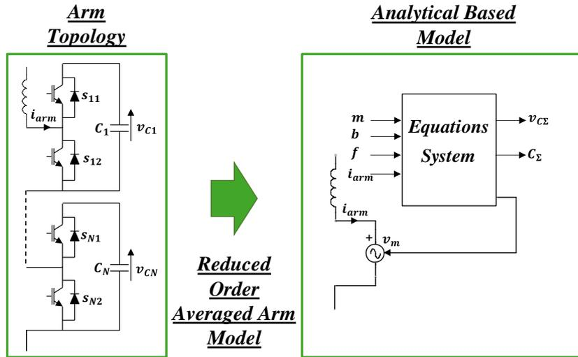
Figure II-25: Reduced order averaged arm model based on analytical modeling technique.
