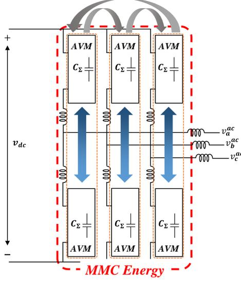
Figure III-29: Distribution of stored energy in the MMC.
