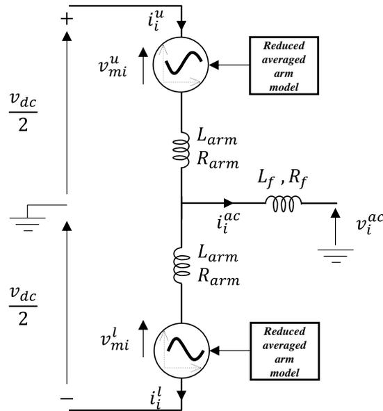
Figure III-24: Simplified circuit for one MMC leg.
