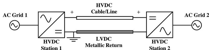
Figure I-4: Asymmetric monopolar scheme with metallic return.
