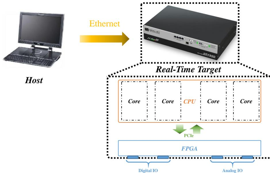
Figure V-2: Hardware in the loop simulation circuit.
