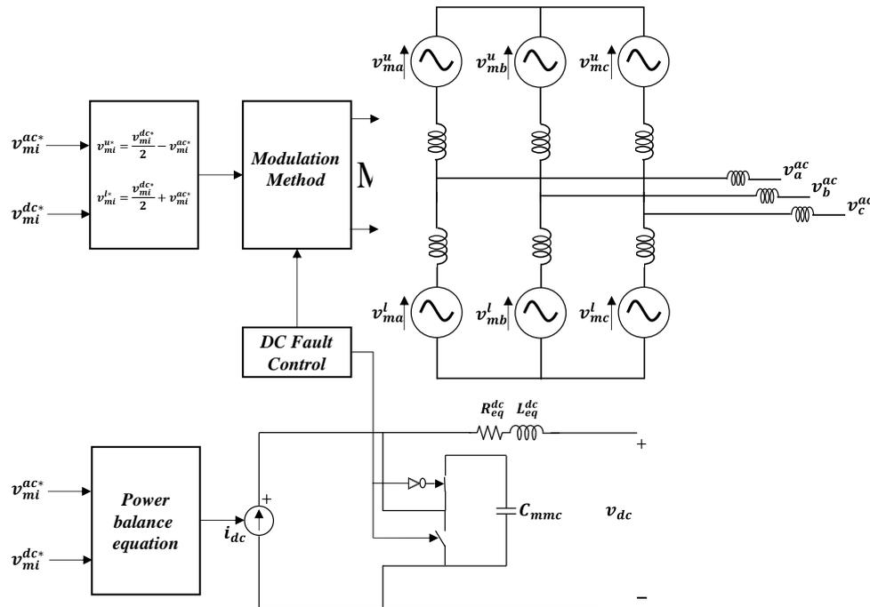
Figure II-14: Reduced order averaged model including blocking capability.
