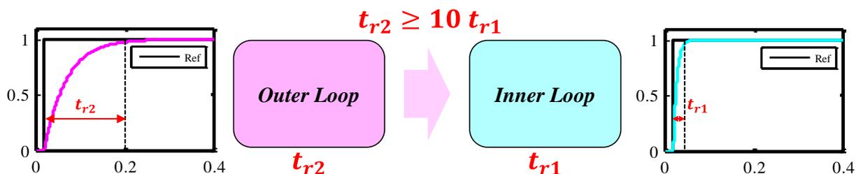
Figure III-31: Cascaded control principle.
