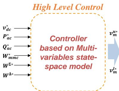
Figure III-30: Multivariable control diagram for MMC.
