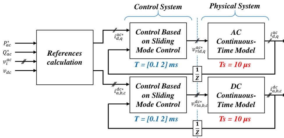
Figure IV-7: Simulation circuit for sliding mode control validation.
