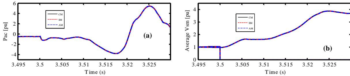
Figure A-7: Dynamics response of equivalent models for a loss of one arm: (a) active power, (b) average SM voltages for upper and lower arms for phase a.
