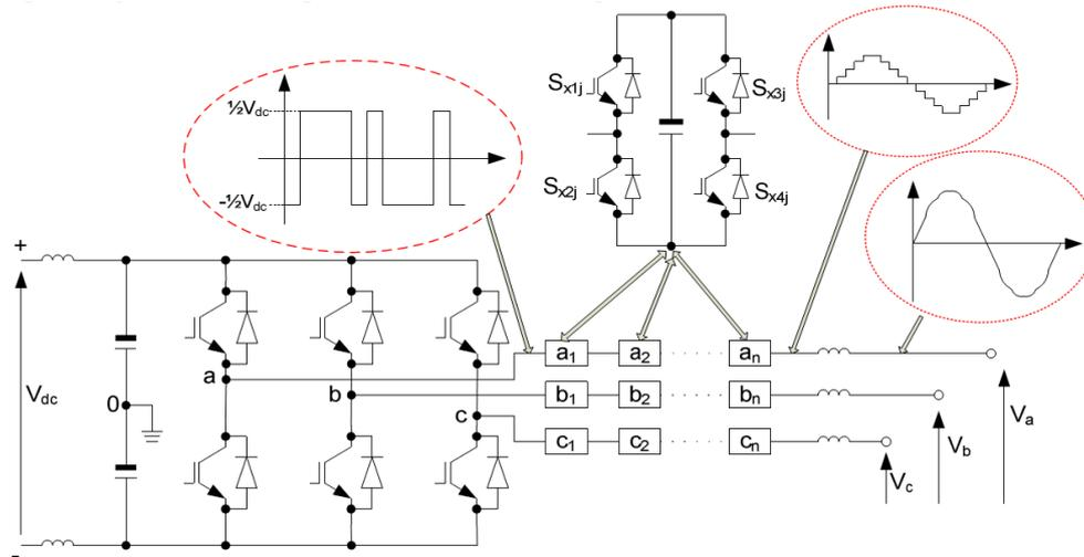
Figure I-21: New hybrid modular multilevel converter (2-level+FB SMs) [32].
