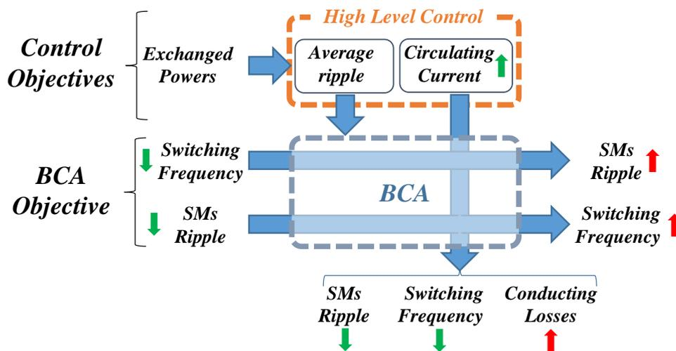
Figure III-10: Criteria and choices of balancing control algorithms.
