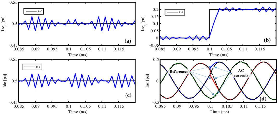
Figure IV-19: Simulation results for reactive power reference change with  $T=1$  ms ( $k_i^{ac}=k_i^{dc}=10000$ ,  $\sigma=50$ ,  $k_p^{ac}=k_p^{dc}=3200$ ): (a) direct component for AC currents, (b) quadrature component for AC currents, (c) DC current, (d) three phase AC currents.
