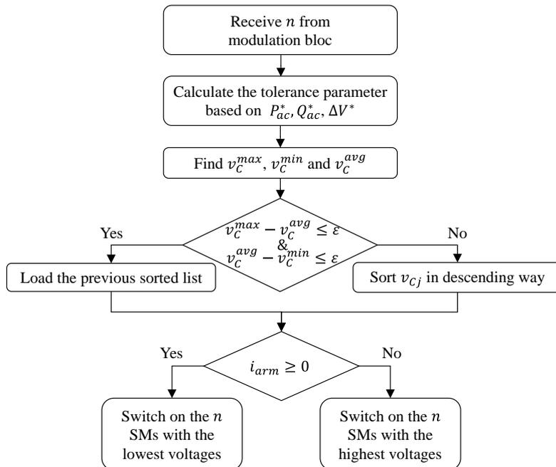
Figure IV-4: Proposed improved average tolerance band algorithm flowchart.
