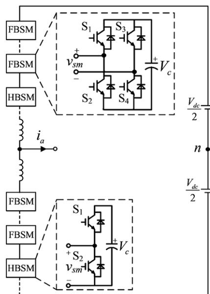
Figure I-20: Hybrid modular multilevel converter (FB+HB) SMs [30].
