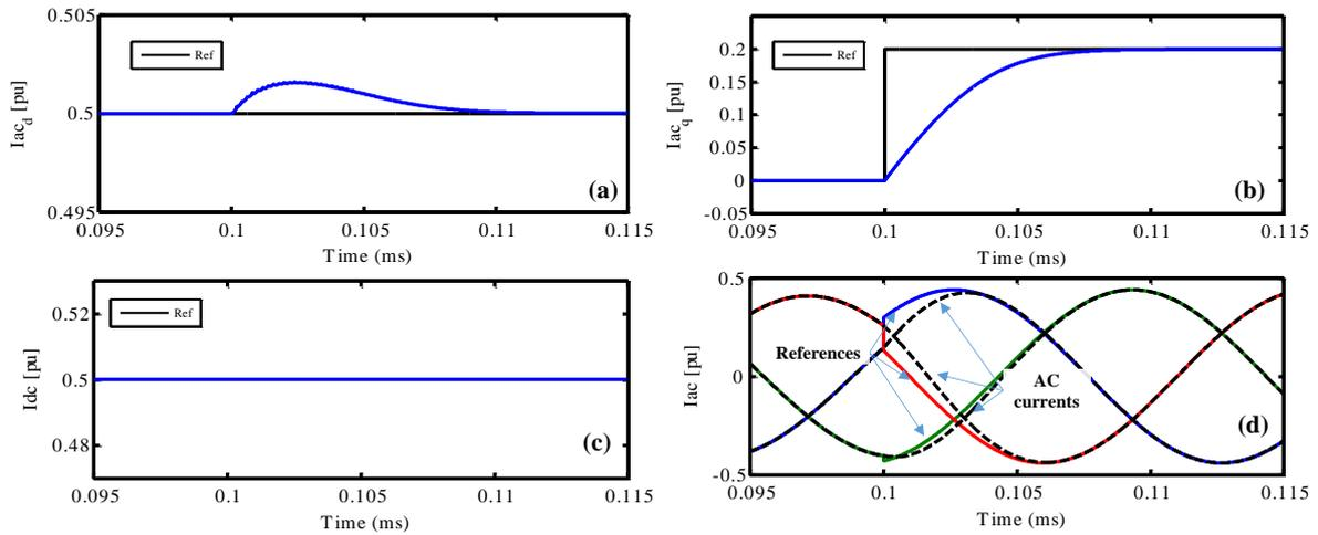
Figure IV-11: Simulation results for reactive power reference change ( $k_i^{ac}=k_i^{dc}=10000$ ,  $\sigma=50$ ): (a) direct component for AC currents, (b) quadrature component for AC currents, (c) DC current, (d) three phase AC currents.
