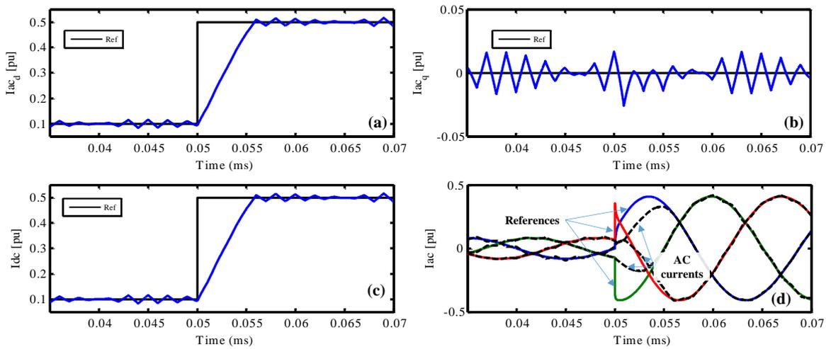
Figure IV-18: Simulation results for active power reference change with  $T=1 \text{ ms}$  ( $k_i^{ac}=k_i^{dc}=10000$ ,  $\sigma=50$ ,  $k_p^{ac}=k_p^{dc}=3200$ ): (a) direct component for AC currents, (b) quadrature component for AC currents, (c) DC current, (d) three phase AC currents.
