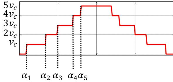
Figure III-6: Modulated arm voltage using SHE modulation technique.
