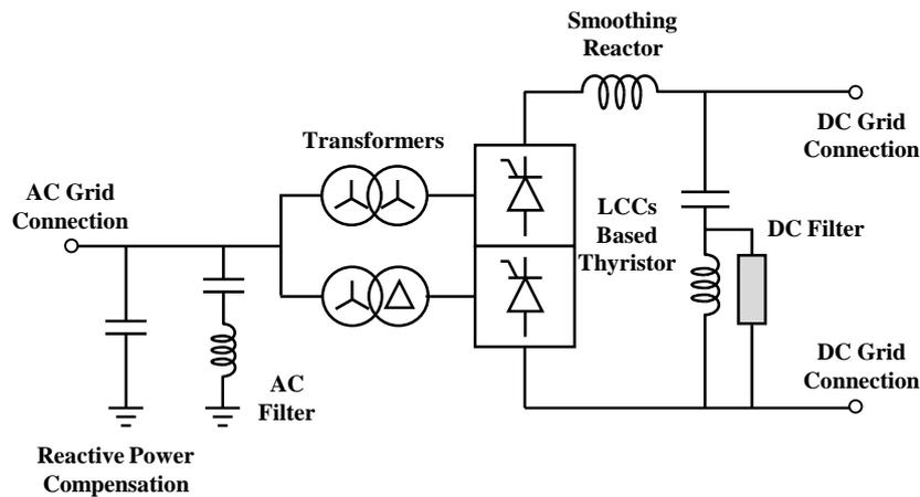
Figure I-10: LCC-HVDC station.
