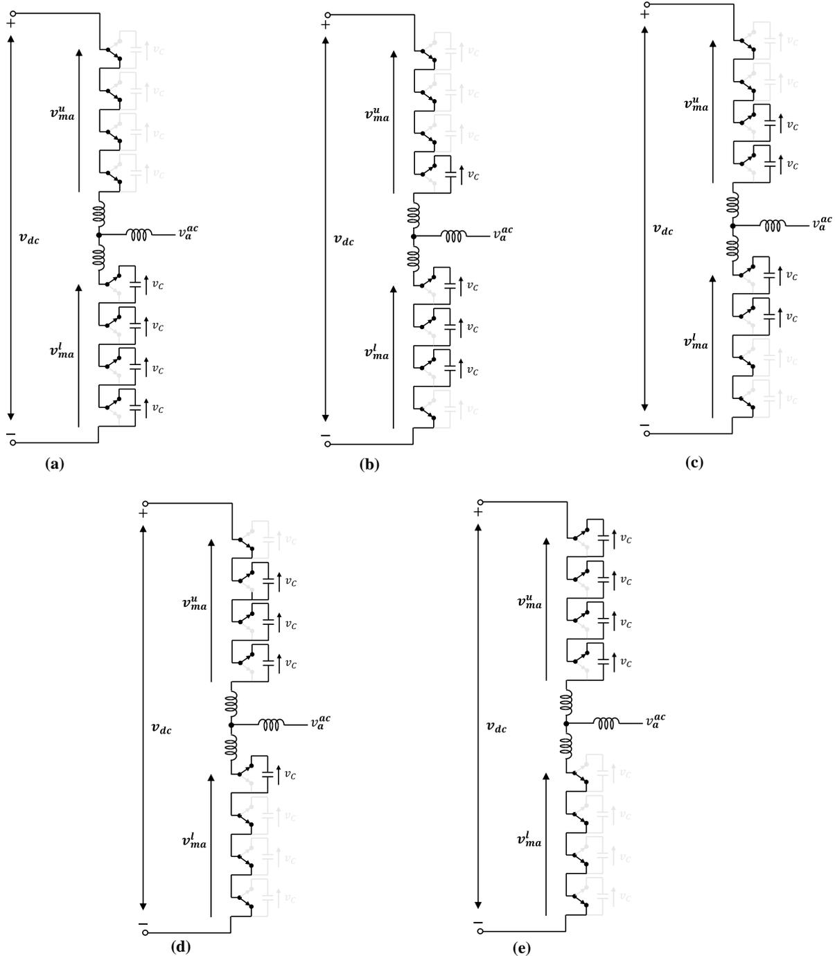
Figure I-16: Operation principle of 5-level MMC.
