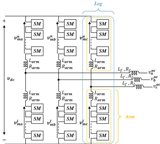
Figure I-15: Three-phase Modular Multilevel Converter (MMC).
