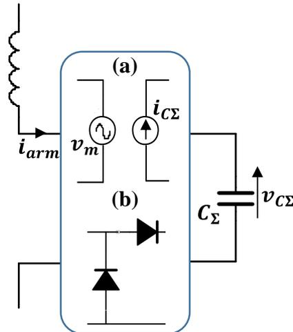
Figure II-15: Reduced order averaged arm model: (a) controlled state, (b) blocked state.
