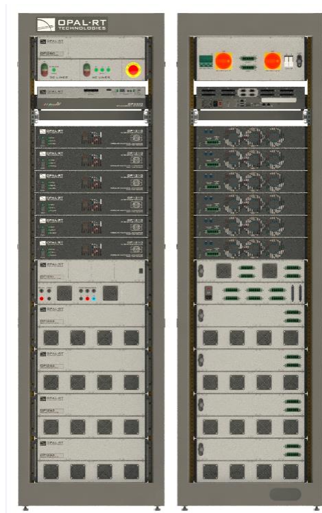
Figure V-8: Small scale MMC station.
