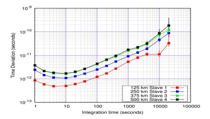
FIGURE 4.41: Time stability calculated from the frequency data for the cascaded 500 km White Rabbit link for default bandwidth of locking along with default PTP rate.
