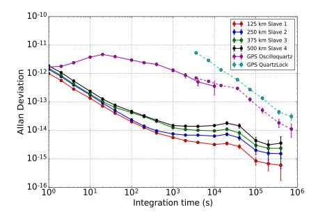
FIGURE 4.31: Allan Deviation for the 500 km cascaded White Rabbit link and comparison with different GPS receivers. Solid line depicts stability calculated from Frequency data, Dashed line depicts stability calculated from Phase data.
