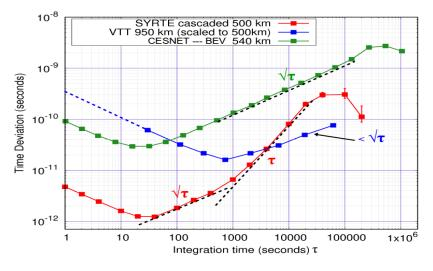
FIGURE 4.33: Time stability (calculated from phase data) for the cascaded 500 km White Rabbit link and comparison with infield applications.
