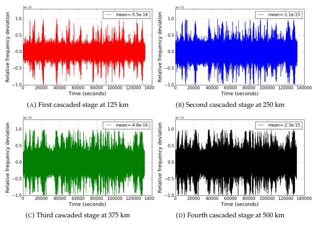
FIGURE 4.36: Relative frequency deviation for each of the cascaded stages of the 500 km White Rabbit link with default PTP rate.
