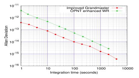
FIGURE 3.9: Comparison of Allan Deviation (NEQ BW=50 Hz) of our Improved Grandmaster WRS with OPNT enhanced WR.
