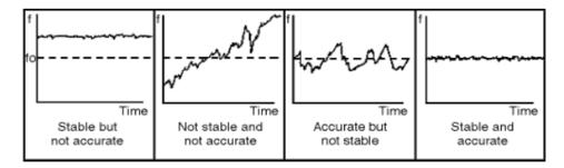
FIGURE 1.1: The relationship between accuracy and stability for a frequency standard of nominal frequency  $f_0$  [1].
