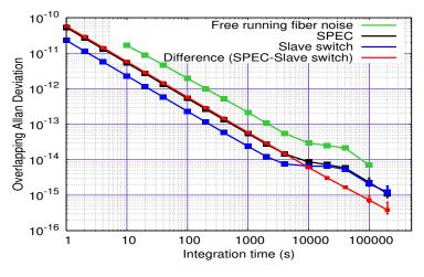
FIGURE 4.8: Overlapping Allan deviation (calculated from phase data) for the 100 km uni-directional WR link with evidence of the fiber thermal noise bump.
