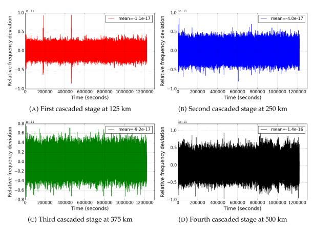
FIGURE 4.30: Relative frequency deviation for each of the cascaded stages of the 500 km White Rabbit link with increased PTP rate and increased BW of locking.
