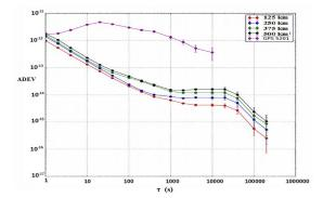
Fig. 8. Allan Deviation for the cascaded 500 km WR link and comparison with GPS Receiver.
