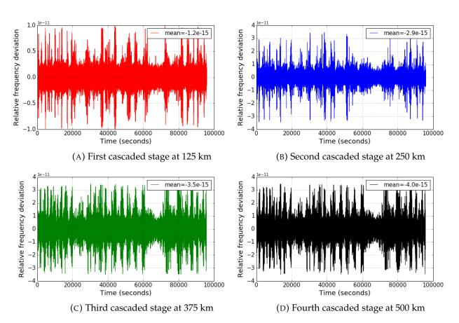
FIGURE 4.39: Relative frequency deviation for each of the cascaded stages of the 500 km White Rabbit link with default bandwidth of locking and default PTP rate.
