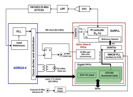
FIGURE 2.16: Clocking scheme of the White Rabbit switch hardware v3.4 (v3.3 lacks the 10 MHz clock output) [71].
