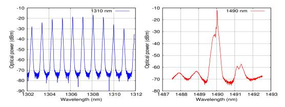
FIGURE 3.13: Optical spectrum of the 1310 and 1490 nm (Bidirectional) CWDM SFPs.
