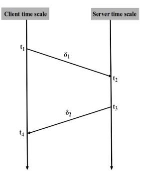
FIGURE 1.8: NTP two way message exchange process.
