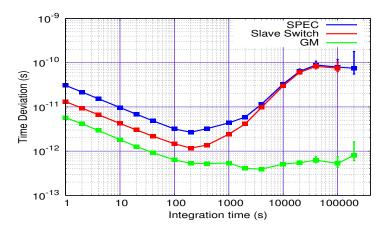
FIGURE 4.6: Time deviation (calculated from phase data) for the 100 km uni-directional WR link.
