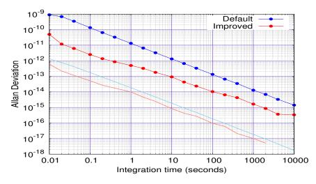
FIGURE 3.8: Allan Deviation (NEQ BW=500 Hz) for default and Improved Grandmaster WR clock (the solid light blue and red lines are their respective noise floors).
