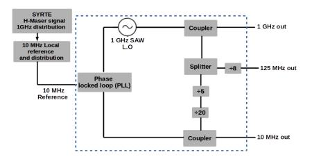
FIGURE 3.3: Schematic of the external 1 GHz local oscillator box.
