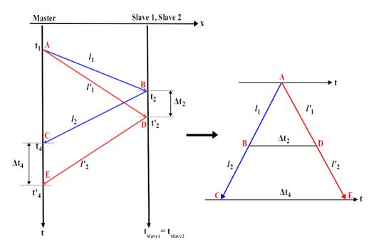
FIGURE 6.6: The two way PTP scheme for dual wavelength technique with Thales theorem representation.
