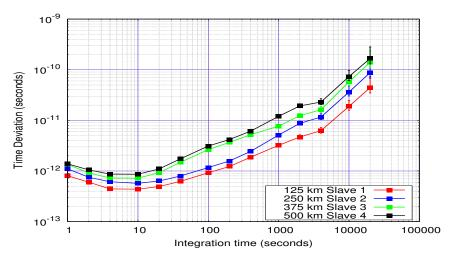
FIGURE 4.38: Time stability calculated from the frequency data for the cascaded 500 km White Rabbit link for default PTP rate.
