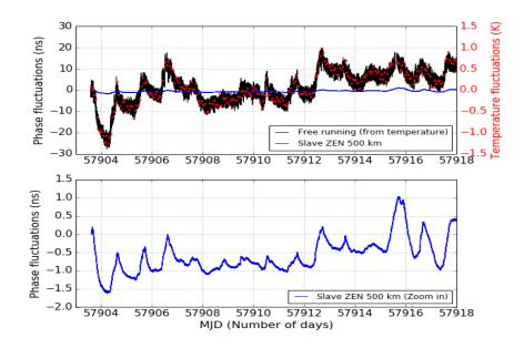
FIGURE 4.32: Top: Free running phase fluctuations calculated from the temperature fluctuations of the experimental room (constant offset removed for both), and the Slave ZEN phase fluctuations (blue trace). The blue trace is zoomed in the bottom figure. We observe a compression factor of about 20.
