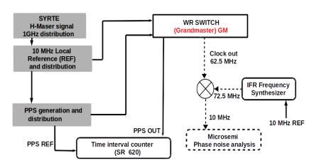
MHz from the IFR frequency Synthesizer which was locked to the 10 MHz reference of the laboratory.
