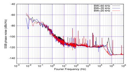
FIGURE 3.7: Phase noise power spectral density of the improved Grandmaster WR clock for PLL bandwidth optimization.
