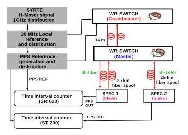
FIGURE 3.12: Experimental setup for comparison of uni-directional (Bi-fiber) and bi-directional (Bi-color) 25 km White Rabbit links.
