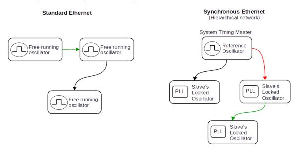
FIGURE 2.2: Comparison between Standard and Synchronous Ethernet [56].
