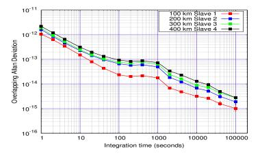
FIGURE 4.22: Overlapping Allan Deviation (calculated from frequency data) for the 400 km cascaded White Rabbit link.
