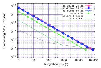
Figure 5. Overlapping Allan deviation for unidirectional and bidirectional link setup.
