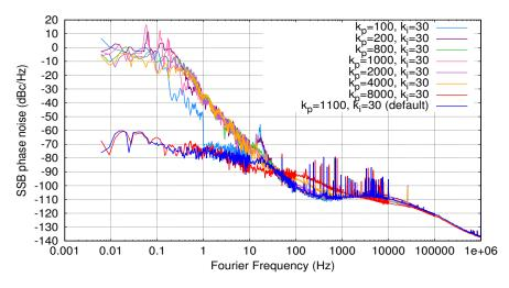
FIGURE 3.20: Power spectral density of the Slave clock for different  $k_p$  values for a constant  $k_i$  =30.
