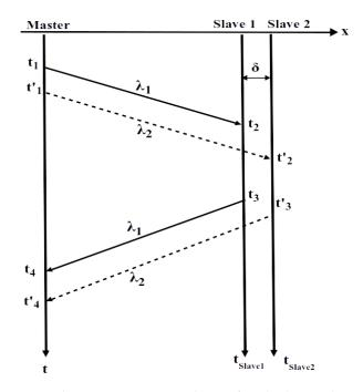
FIGURE 6.5: The two way PTP scheme for dual wavelength technique.
