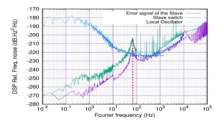
FIGURE 3.29: Relative frequency noise for the Slave switch, error signal of the Slave switch and for the local oscillator of the WRS.
