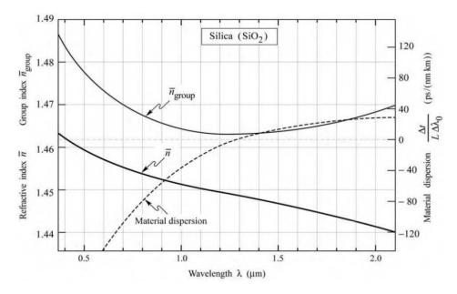
FIGURE 2.15: Refractive index, group index and material dispersion of silica fibers [63].
