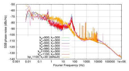
FIGURE 3.24: Power spectral density of the Slave clock for fine tuning of  $k_p$  values for a constant  $k_i$  =300.
