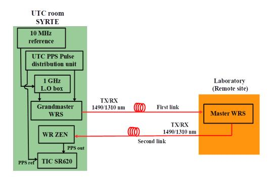
FIGURE 5.1: Experimental setup of the UTC room to Laboratory White Rabbit link.
