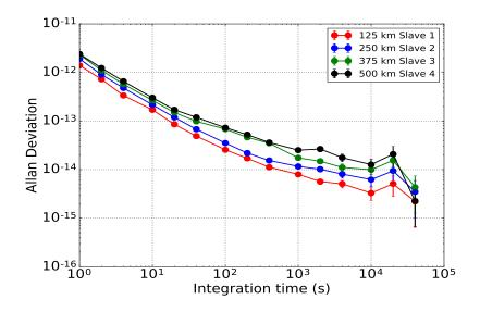
FIGURE 4.37: Allan Deviation (calculated from frequency data) for the 500 km cascaded White Rabbit link for default PTP rate.
