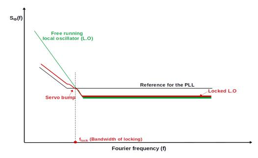
FIGURE 2.17: Illustration of a typical Phase noise power spectral density for a free running local oscillator, for the external reference signal and for the locked local oscillator.
