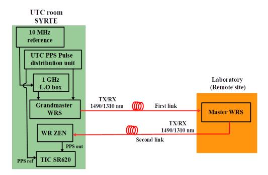
FIGURE 6.3: Experimental setup of the UTC room to Laboratory White Rabbit link.
