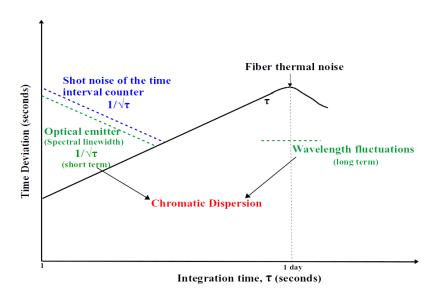
FIGURE 4.47: Pictorial representation of the short term and long term limitations for time stability performance of a long haul White Rabbit link.
