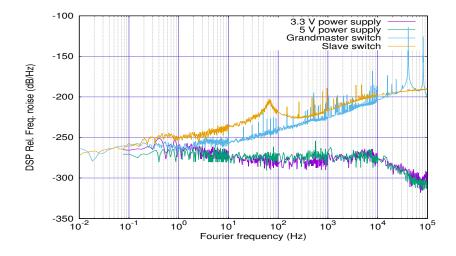
FIGURE 3.30: Relative frequency noise contribution from the 3.3 V and 5 V internal power supply, for the Grandmaster and the Slave switch.
