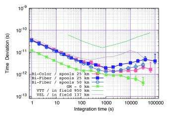
Figure 4. Time deviation for the unidirectional and bidirectional links.
