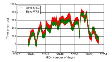
FIGURE 4.4: Phase data for the two Slaves (constant offset removed).
