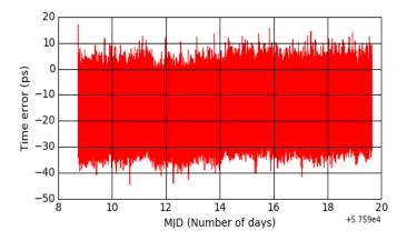
FIGURE 3.10: Phase data for the improved Grandmaster WRS (constant offset has been removed).
