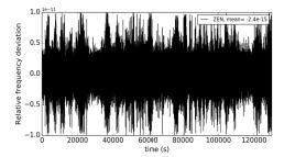
Fig. 5. Relative frequency deviations for WR-ZEN clock out with default PTP rate.
