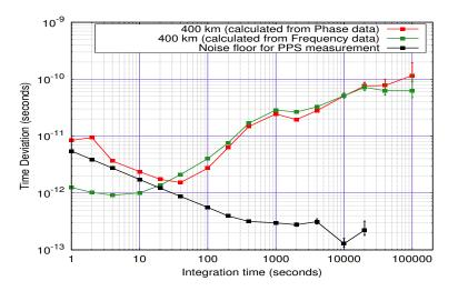
FIGURE 4.28: Time stability comparison for the frequency data and phase data for the 400 km cascaded link.
