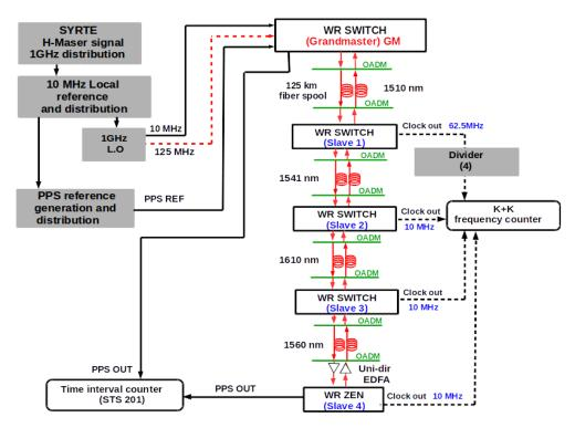
FIGURE 4.29: Experimental setup for the cascaded 500 km White Rabbit link.
