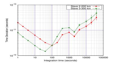
FIGURE 4.19: Time Deviation (calculated from the phase data) for the 200 and 300 km cascaded stages.
