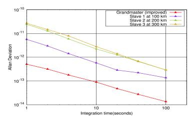
FIGURE 4.16: Allan Deviation (NEQ BW=500 Hz) for the cascaded stages.
