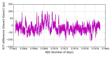
FIGURE 6.9: Fluctuations of the round trip time difference Slave2-Slave1 (offset has been removed).
