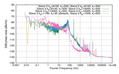
FIGURE 4.13: Phase noise power spectral density of the third Slave clock for default gain values and different  $k_p$  values for constant  $k_i$ =500.
