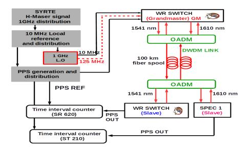
FIGURE 4.1: Experimental setup for a 100 km White Rabbit unidirectional link.
