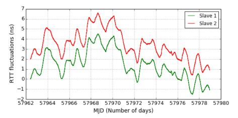
FIGURE 6.8: Round trip time fluctuations for both the Slaves over 16 days of measurement (offset has been removed for both). The trace for Slave 2 has been shifted by 2 ns for clarity.
