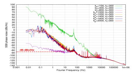
FIGURE 3.22: Power spectral density of the Slave clock for different  $k_p$  values for a constant  $k_i$  =300.
