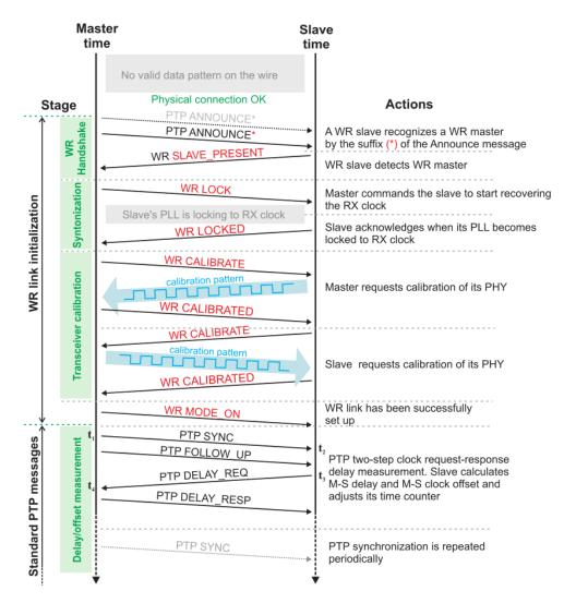
FIGURE 2.9: WR-PTP message exchange flow [56].
