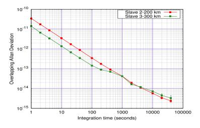
FIGURE 4.18: Overlapping Allan Deviation (calculated from the phase data) for the 200 and 300 km cascaded stages.
