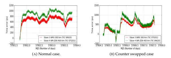
FIGURE 4.25: Phase data measurement for the 300 and 400 km cascaded link for the test of short term stability limitation.
