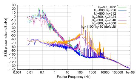
FIGURE 3.21: Power spectral density of the Slave clock for different  $k_i$  values for a constant  $k_p$  =800.
