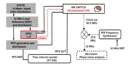
FIGURE 3.5: Experimental setup for the "improved" GM switch performance analysis.
