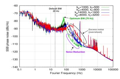
FIGURE 4.2: Phase noise power spectral density of the Slave clock for  $k_p$ =4000 and  $k_i$  values.
