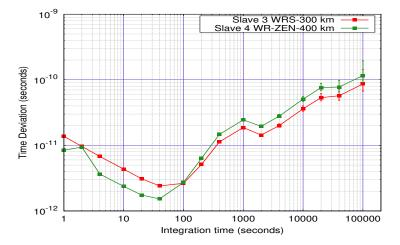
FIGURE 4.24: Time Deviation calculated from the phase data for the 300 km cascaded stage and for the user end node at 400 km.
