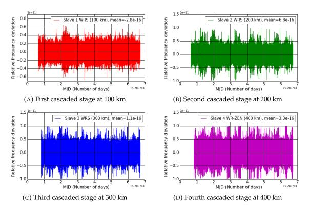
FIGURE 4.21: Relative frequency deviation for each of the cascaded stages of the 400 km cascaded White Rabbit link.
