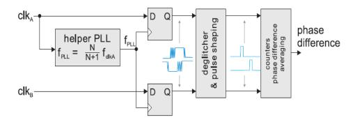
FIGURE 2.4: Schematic of a digital DMTD phase detector [56].
