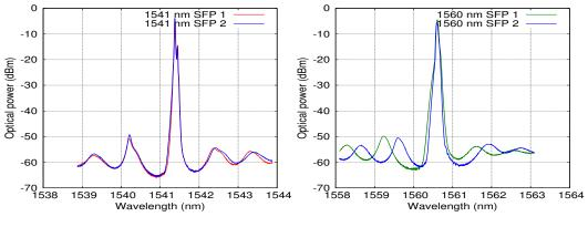
FIGURE 3.14: Optical spectrum of the 1541 and 1560 nm (Unidirectional) DWDM SFPs.
