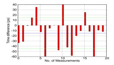
FIGURE 6.2: Variation of the delay (offset has been removed) for connecting/disconnecting the fiber link.
