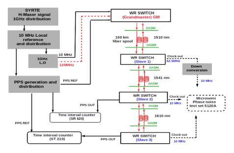
FIGURE 4.11: Experimental setup for the cascaded 300 km White Rabbit link.
