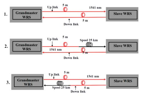
the fiber link from the Slave to Grandmaster as the down link.
