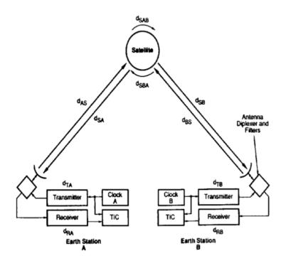
FIGURE 1.7: Two way satellite time and frequency transfer [18].
