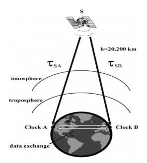
FIGURE 1.5: GPS common-view technique [10].
