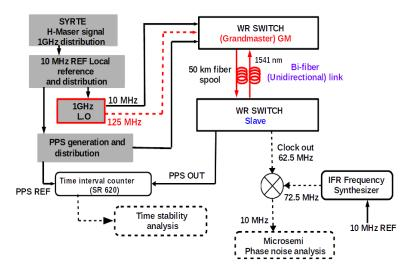
FIGURE 3.23: Experimental setup for a 50 km White Rabbit unidirectional link.
