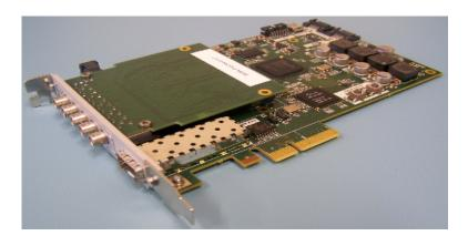
FIGURE 2.11: SPEC board hosting the five channel FMC card DIO [60].
