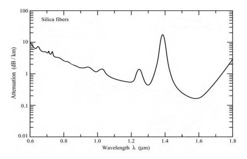
FIGURE 2.14: Optical attenuation variation with wavelength [63].
