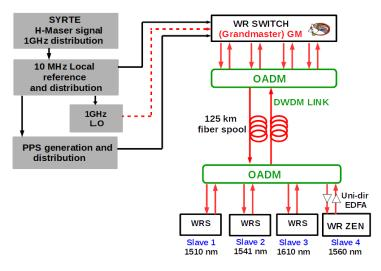
FIGURE 4.43: Experimental setup for the multi user 125 km White Rabbit link.
