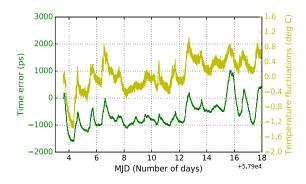
Fig. 7. Phase data for WR-ZEN and the temperature fluctuations of the experimental room (constant offset removed for both).
