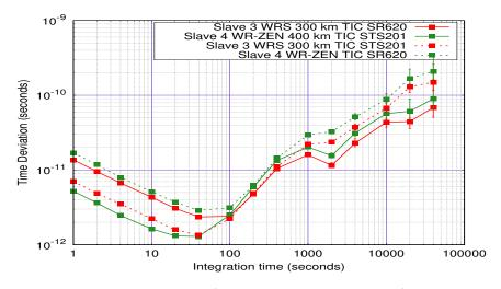
FIGURE 4.27: Comparison of Time Deviation (calculated from phase data) for the 300 and 400 km cascaded stages for counter swapped case.
