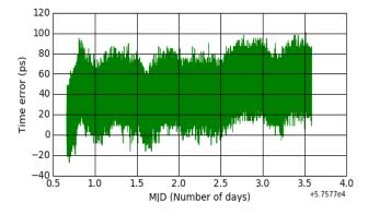
FIGURE 3.26: Phase data of the Slave WRS for the 50 km WR link (constant offset has been removed).
