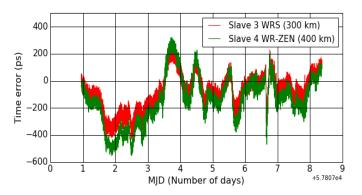
FIGURE 4.23: Phase data for the cascaded 300 km stage and for the user end node at 400 km (constant offset removed).
