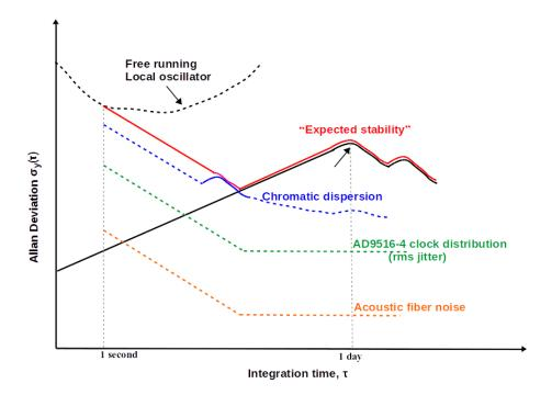
FIGURE 2.19: Pictorial representation of the potential noise sources that could limit the frequency stability performance of a typical Grandmaster and Slave White Rabbit Switch.
