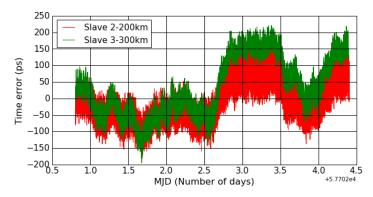
FIGURE 4.17: Phase data for the 200 and 300 km cascaded stages (constant offset removed).
