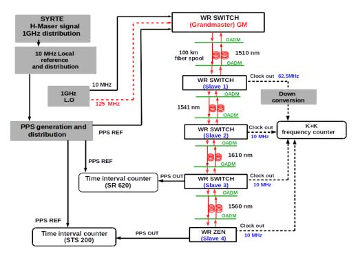
FIGURE 4.20: Experimental setup for the cascaded 400 km White Rabbit link.
