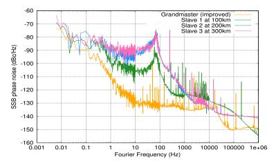
FIGURE 4.15: Phase noise power spectral density comparison for the cascaded stages.
