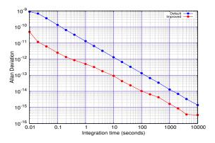
Fig. 2. Allan Deviation for default and Improved Grandmaster WR clock.
