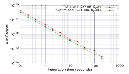
FIGURE 3.25: Allan deviation (NEQ BW=50 Hz) for the Slave switch for default and optimized gain parameters.
