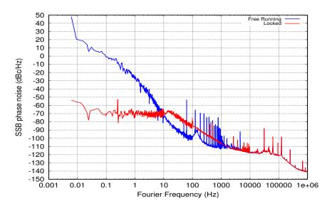
FIGURE 3.2: Phase noise power spectral density for the Grandmaster WR clock.
