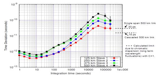
FIGURE 4.34: Time stability calculated from the frequency data for the cascaded 500 km White Rabbit link.
