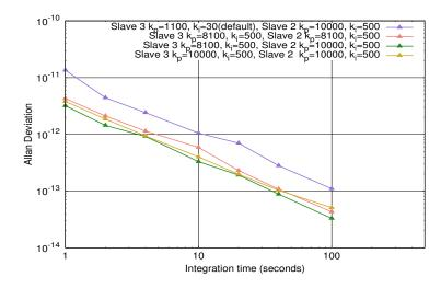
FIGURE 4.14: Allan Deviation (NEQ BW=5 Hz) for the third Slave clock for default gain values and higher  $k_p$  values for constant  $k_i$ =500.
