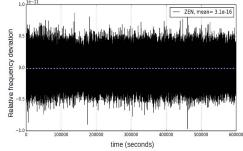
Fig. 6. Relative frequency deviations for WR-ZEN clock out with increased PTP rate.
