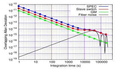
FIGURE 4.5: Overlapping Allan deviation (calculated from phase data) for the 100 km uni-directional WR link.
