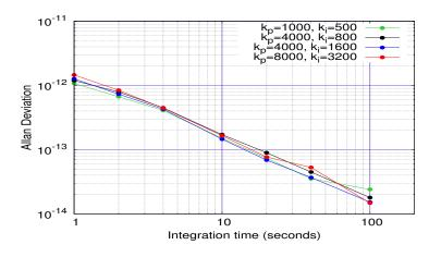
FIGURE 4.3: Allan Deviation of the Slave clock for different  $k_p$  and  $k_i$  values.
