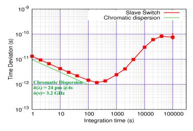
FIGURE 4.10: Chromatic dispersion contribution to the time stability performance of the Slave switch (100 km telecom span uni-directional link).
