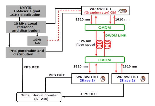
FIGURE 6.7: Experimental setup for a 125 km White Rabbit unidirectional link for two Slave WRS.
