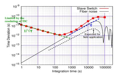
FIGURE 4.9: Limitations for the time stability (calculated from phase data) performance of the 100 km White Rabbit link.
