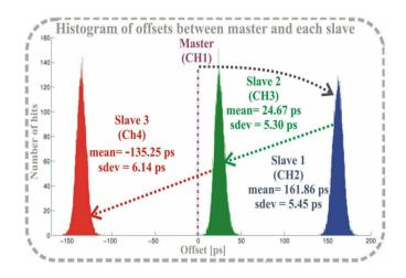
FIGURE 1.9: WR synchronization performance for initial experiments by CERN[42].
