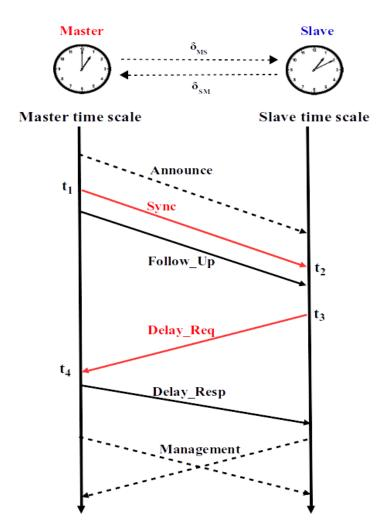
FIGURE 2.1: PTP two way messsage exchange mechanism [39].
