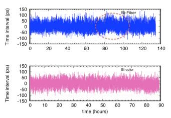
Figure 3. Time intervals raw data using the bi-fiber and the bi-color end-node modules. The time offset were removed.
