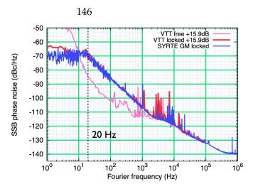
Figure 2. Power spectral density of the White Rabbit switch clock output in locked and free running modes, showing the results of this work and the previous measurements by A. Wallin of VTT [17].
