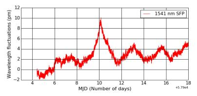
FIGURE 4.35: Wavelength fluctuations for the 1541 nm SFP (constant offset removed).
