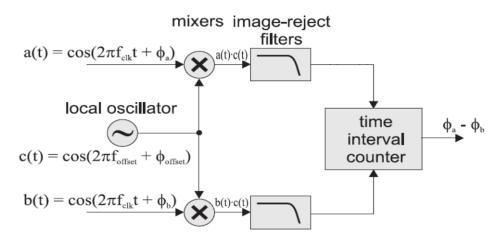
FIGURE 2.3: Schematic of an analog DMTD phase detector [56]
