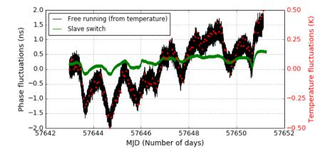
FIGURE 4.7: Ambient temperature variations experienced and recorded by the time interval counter STS201 and the calculated phase fluctuations. The green trace is the Slave switch data as in Fig. 4.4. We observe a compression factor of about 5 at half a day.
