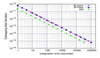
FIGURE 3.16: Overlapping Allan Deviation (calculated from phase data) for the unidirectional and bidirectional setups (Bandwidth of measurement = 1 Hz).
