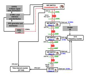
Fig. 4. Experimental Setup for the 500 km cascaded WR link.
