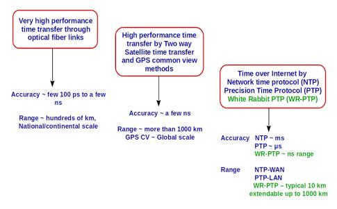
FIGURE 1.10: Performance comparison of some time transfer methods.
