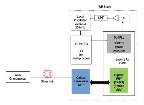
FIGURE 2.18: A WR Slave system review for studying its potential performance limitations [71].
