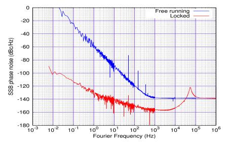
FIGURE 3.4: Phase noise power spectral density of the 10 MHz output signal of the 1 GHz local oscillator box.
