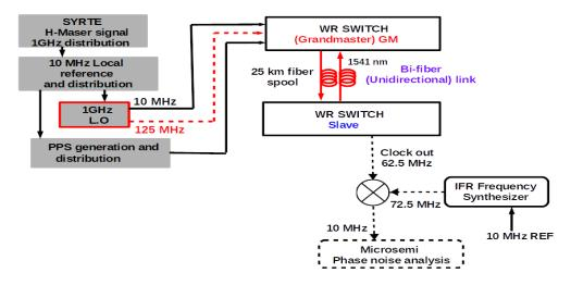
FIGURE 3.19: Experimental setup for a 25 km White Rabbit unidirectional link.
