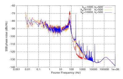
FIGURE 4.12: Phase noise power spectral density of the Second Slave clock for different  $k_p$  values with constant  $k_i$ =500.
