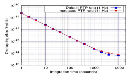
FIGURE 3.31: Frequency stability (calculated from phase data) comparison for default and increased PTP rate for the Slave WRS (100 km link).
