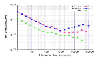
FIGURE 3.17: Time Deviation (calculated from phase data) for the unidirectional and bidirectional setups (Bandwidth of measurement = 1 Hz).
