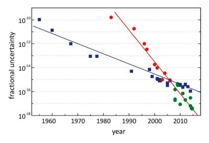
FIGURE 1.2: The time evolution of the uncertainty of Cesium and Optical clocks. Fractional uncertainty of primary Cesium atomic clocks to realize the second in the SI (squares) and optical frequency clocks (dots). Green dots represent optical clocks with estimated standard uncertainties whose optical frequency can be determined only with the accuracy of the frequency comparison with a primary Cesium clock [7].
