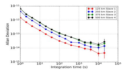
FIGURE 4.40: Allan Deviation (calculated from frequency data) for the 500 km cascaded White Rabbit link for default bandwidth of locking along with default PTP rate.
