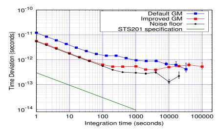
FIGURE 3.11: Time Deviation for default and Improved Grandmaster switch (Bandwidth of measurement = 1 Hz).
