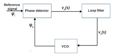
FIGURE 3.18: Block diagram of a typical phase locked loop [81].
