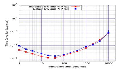
FIGURE 4.42: Time stability comparison calculated from phase data for the cascaded 500 km White Rabbit link for default bandwidth of locking along with default PTP rate.
