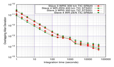
FIGURE 4.26: Comparison of Overlapping Allan Deviation (calculated from phase data) for the 300 and 400 km cascaded stages for counter swapped case.
