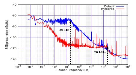
FIGURE 3.6: Phase noise power spectral density for default and improved Grandmaster WR clock.
