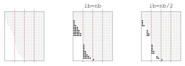
Figure 3.6: The effect of internal blocking on the generated fill-in. The light gray dots show the frontal matrix structure if no blocking of operations is applied whereas the dark gray dots show the additional fill-in introduced by blocked operations.
