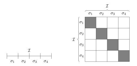
Figure 5.2: An example of clustering and its associated flat block-clustering and BLR representation where we have assumed a weak admissibility condition.
