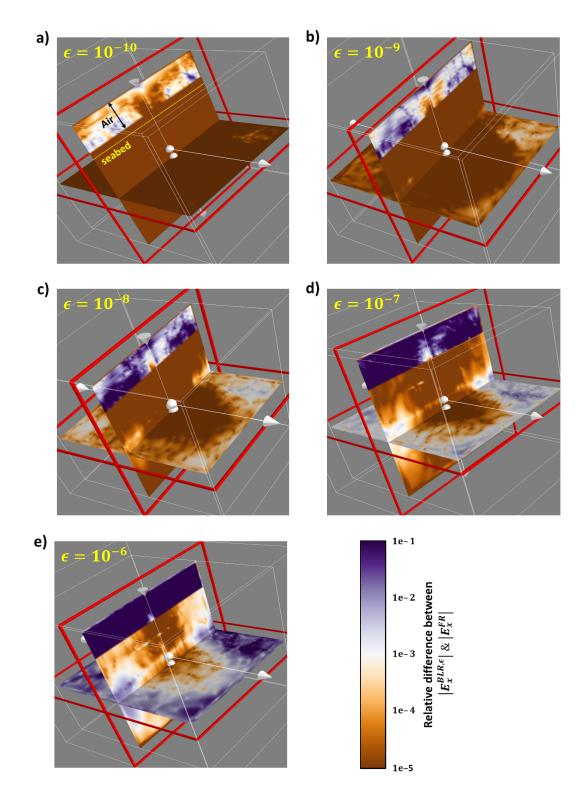
Figure 5.14: Relative difference between the BLR solution  $x^{\varepsilon}$  for different low-rank thresholds  $\varepsilon$ , and the FR solution x for a linear system corresponding to matrix H3. For  $\varepsilon = 10^{-7}$ , the solution accuracy is acceptable everywhere except in the air layer at the top. The results are for the *x*-component of the electric field. The air and PML layers are not to scale.
