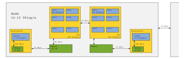
Figure 2.18: Illustration of a typical HPC computing platform architecture.
