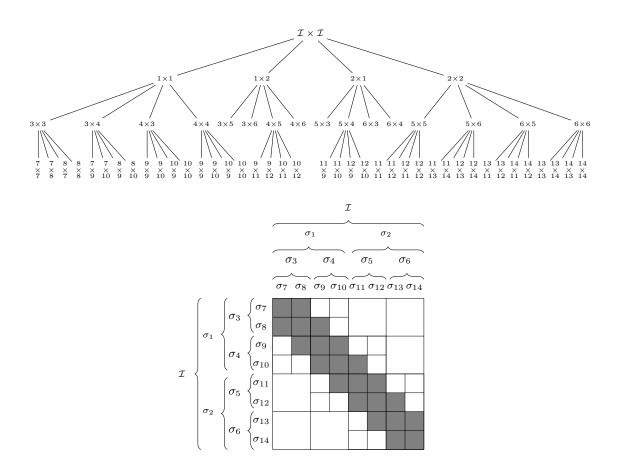
Figure 5.3: An example of block-cluster tree on top  $(\sigma_i \times \sigma_j)$  has been abbreviated as  $i \times i$  and its associated  $\mathcal{H}$ -admissible block-partition at the bottom; the white blocks are admissible whereas the gray ones are non admissible but smaller than  $c_{min}$ .
