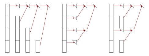
Figure 3.12: Possible panel reduction trees for the 2D front factorization. On the (*left*), the case of a flat tree, i.e., with  $bh = \infty$ . In the (*middle*), the case of a binary tree, i.e., with (bh = 1). On the (*right*) the case of an hybrid tree with bh = 2.
