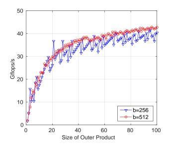
Figure 5.23: Performance benchmark of the Outer Product step on brunch. Please note that the average sizes (first line) and speed values (eighth line) of Table 5.17 cannot be directly linked using this figure because the average size would need to be weighted by its number of flops.
