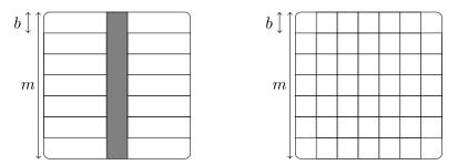
Figure 5.15: Illustration of the BLR-admissibility condition. On the left an example of a non-BLR-admissible partition. Here, the gray subdomain has  $N_{na} = O(m/b) \neq O(1)$  neighbors. On the right example of a BLR-admissible partition when  $q \geq N_{na} = 9 = O(1)$ , the maximal number of neighbors of any block.
