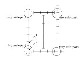
(b) Zoom on current separator and border. The separator's clustering has been computed with the halo method. The border's clustering is inherited from several separator clusterings. At some corners, a cluster maybe not be entirely involved in current front so that tiny clusters may appear.
