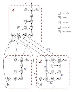
Figure 3.3: The DAG associated with supernodes 1, 2 and 3 of the problem in Figure 2.9; for the panel, update and assemble operations, the corresponding block-column index is specified. For this example, the block-column size is chosen to be one.
