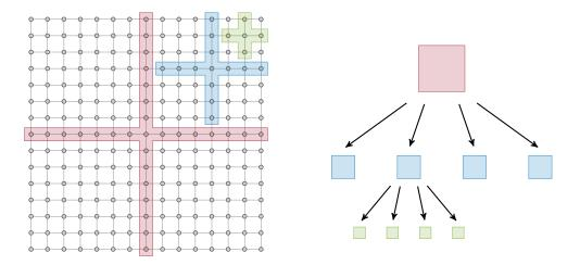
Figure 2.13: On the left, three level of nested dissection with cross-shaped separators on a 2D square domain. On the right, the corresponding separators/assembly tree.
