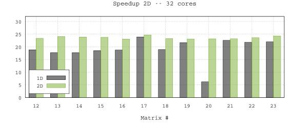
Figure 3.17: Speedup of the 1D and 2D algorithms with respect to the sequential case on ada (32 cores).
