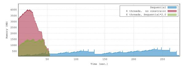
Figure 4.2: The memory profiles for matrix #12 from Table A.1 for a sequential (in blue) and 6-threaded parallel QR factorization without memory constraint (in red) and with a constraint equal to 2.0 times the sequential peak (in green).
