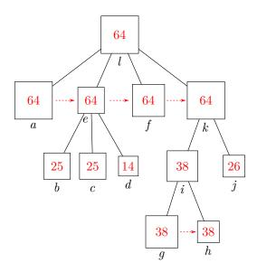
Figure 4.8: Simple example of memory-aware mapping. The tree shown in Figure 4.7(a) is mapped using the flat memory-aware mapping with  $M_0 = 160$  MB. The scheduling constraints resulting from tree serialization are shown with arrows. The subtree rooted at a is processed first and is followed by the subtrees rooted at e and f, and the subtree rooted at k is processed last. Similarly, the subtree rooted at i is mapped using a local tree serialization mapping.
