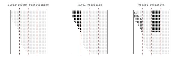
Figure 3.1: Block-column partitioning of a frontal matrix (*left*) and panel and update operations pattern (*middle* and *right*, respectively); dark gray coefficients represent data read by an operation while black coefficients represent written data.
