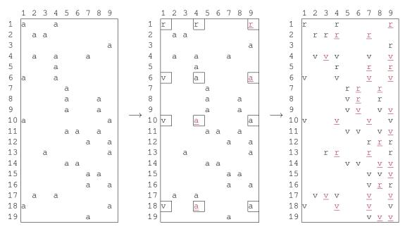
Figure 2.7: A sparse, overdetermined matrix on the left side; the nonzero coefficients of the matrix are denoted with the letter a. In the middle part, the first step of the Householder QR factorization. This modifies rows 1, 6, 10 and 18. After this step, the computed coefficients of the R factor and of the V matrix are denoted, respectively, with the letters rand v; fill-in coefficients are underlined. On the right size, the result of the complete QR factorization.
