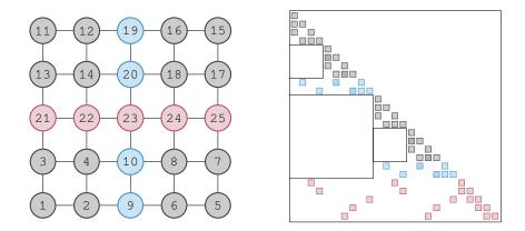
Figure 2.12: An example of nested dissection on a  $5 \times 5$  grid. The topmost separator cuts the domain horizontally in two halves which are then cut vertically by other separators. The resulting permuted matrix is shown on the right side.
