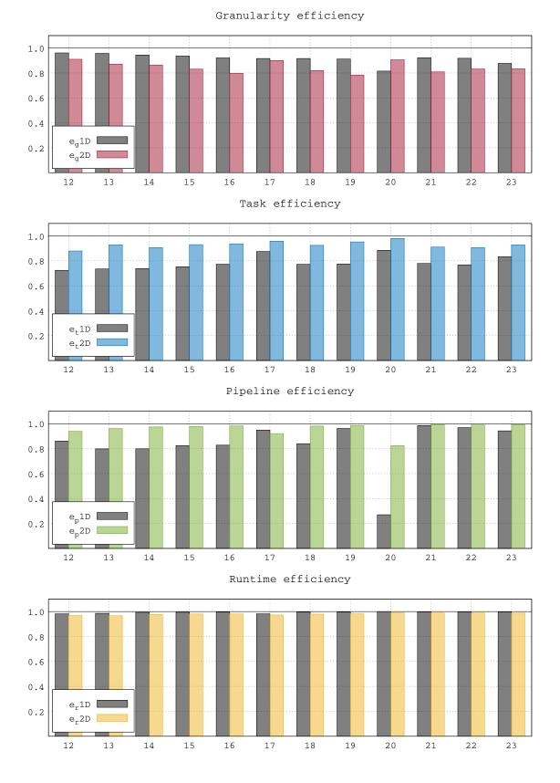
Figure 3.24: Efficiency measures for the STF 1D and 2D algorithms on ada (32 cores).
