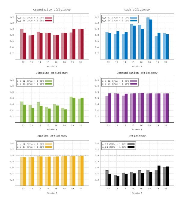
Figure 3.25: Efficiency measures for the STF heterogeneous algorithm on Sirocco with both configurations 12 CPUs ( $1 \times \text{E5-2680}$ ) + 1 GPU ( $1 \times \text{K40M}$ ) and 24 CPUs ( $2 \times \text{E5-2680}$ ) + 1 GPU ( $1 \times \text{K40M}$ ). Note that due to technical issues in StarPU, we are currently unable to obtain the efficiency measures for matrix # 17.
