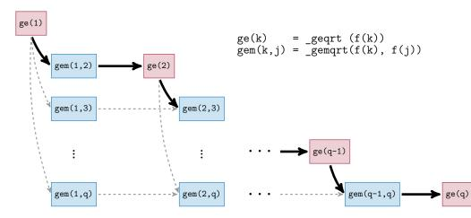
Figure 3.10: Task graph for the block-column QR factorization of a dense matrix with q block columns. Arrows show tasks dependencies; the critical path is shown with thick solid edges.
