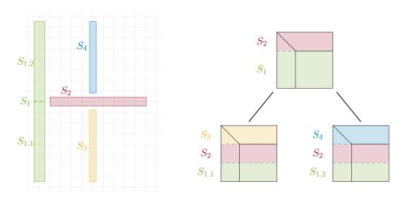
Figure 5.4: Some separators of a 2D regular grid ( $S_1$  being the topmost) and the associated fronts.
