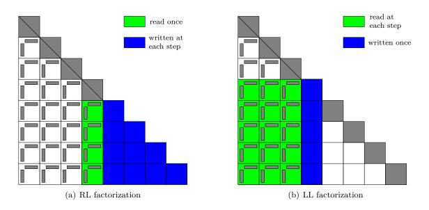
Figure 5.22: Illustration of the memory access pattern in the RL and LL BLR Update during step k of the factorization of a matrix of  $p \times p$  blocks (here, p = 8 and k = 4).
