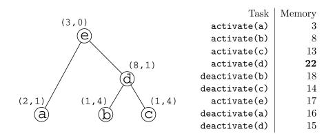
Figure 4.1: The memory consumption (right) for a 5-nodes elimination tree (left) assuming a sequential traversal in natural order. Next to each node of the tree the two values corresponding to the factors (permanent) and the contribution block (temporary) sizes in memory units.
