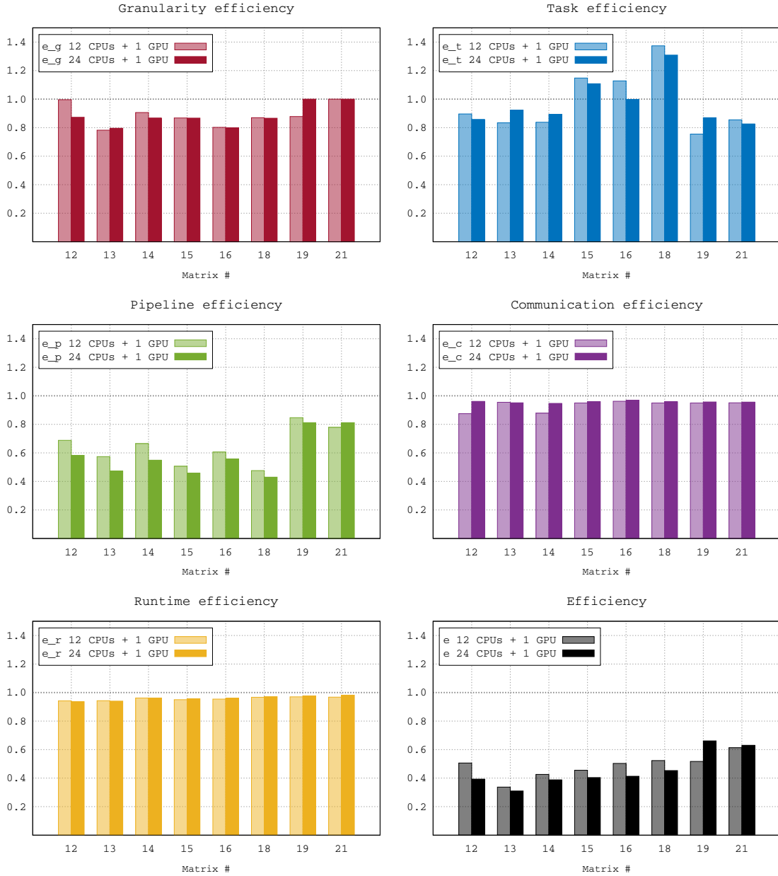
Figure 3.25: Efficiency measures for the STF heterogeneous algorithm on Sirocco with both configurations 12 CPUs ( 1 \times E5-2680 ) + 1 GPU ( 1 \times K40M ) and 24 CPUs ( 2 \times E5-2680 ) + 1 GPU ( 1 \times K40M ). Note that due to technical issues in StarPU, we are currently unable to obtain the efficiency measures for matrix # 17.
