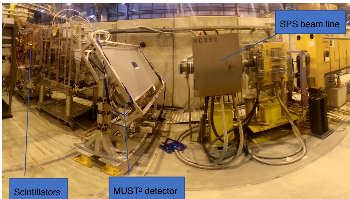
Figure 7. 1 Latency scan setup within the SPS' beam test facilities.
