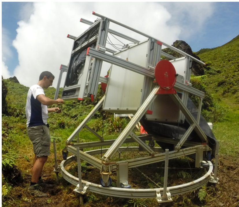
Figure 3. 3 Muon telescope from Diaphane project composed of aligned scintillator planes.
