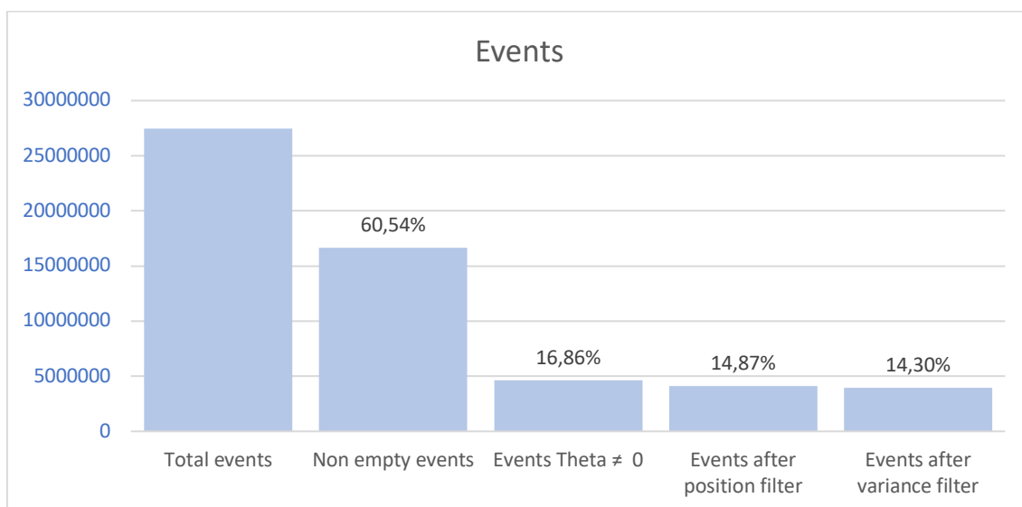
Figure 8. 16 Distribution of recorded events according to track reconstruction.
