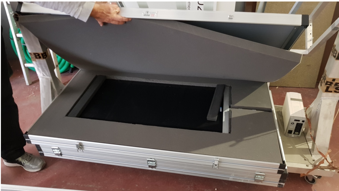
Figure 5. 37 Scintillators used for external trigger.
