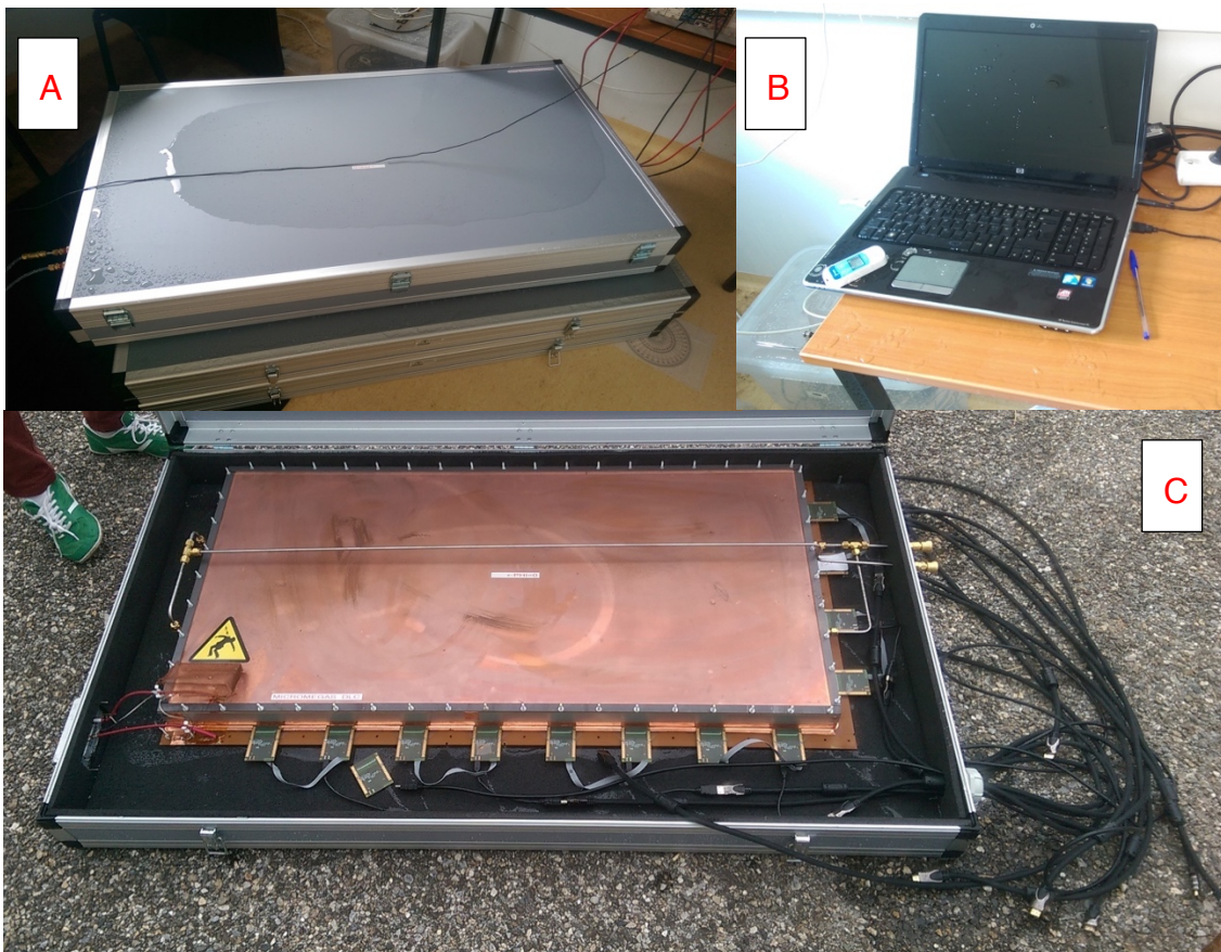
Figure 7.22 (A) Presence of water in the experimental setup after the storm, (B) damaged acquisition computer, and (C) presence of water inside the protection box.
