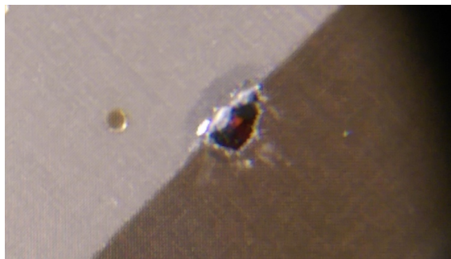
Figure 5. 45 Micromesh consolidated after body extraction.
