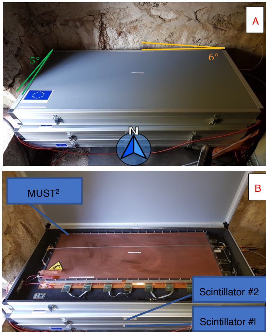
Figure 8. 14 Detector setup during the data acquisition at the valve house.
