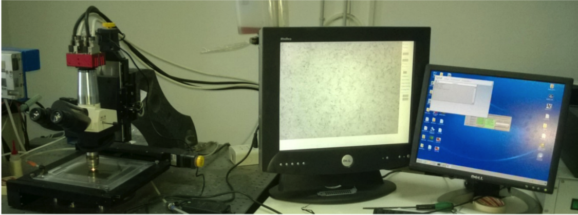
Figure 3. 1 Readout robot analyzing a nuclear emulsion with an automatic microscope.
