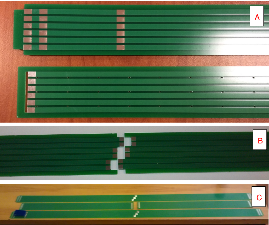
Figure 5. 27 Electric field cage PCB components.
