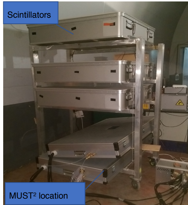
Figure 7. 14 Experimental setup with MUST 2 detectors and liquid scintillators.
