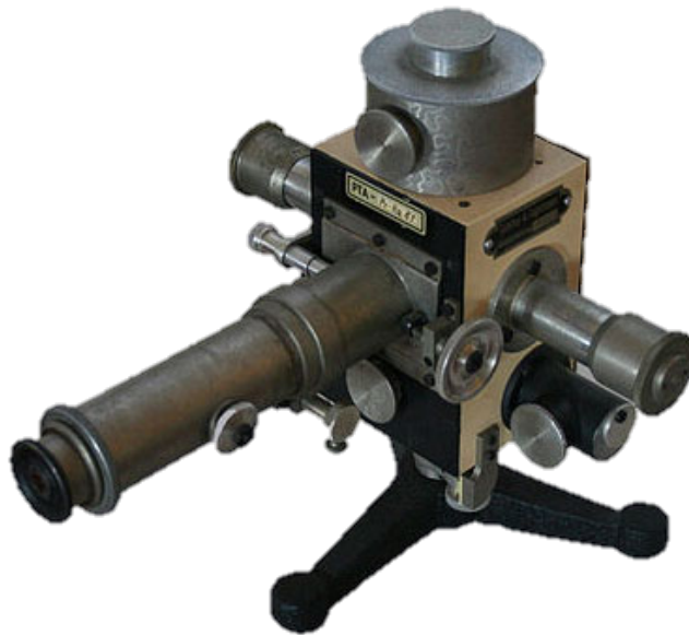
Figure 2. 3 Wulf's original electroscope.
