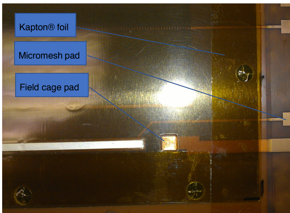
Figure 5. 28 Detail of the Kapton® foil added to isolate the micromesh.
