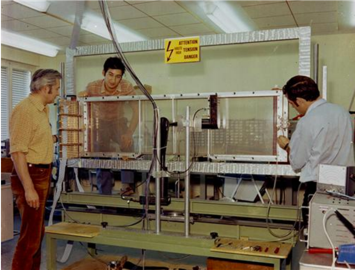
Figure 3. 4 From left to right, Georges Charpak, Fabio Sauli and Jean-Claude Santiard working on a multiwire chamber in 1970. Image from CERN document server, original ref.: 8-8-70.
