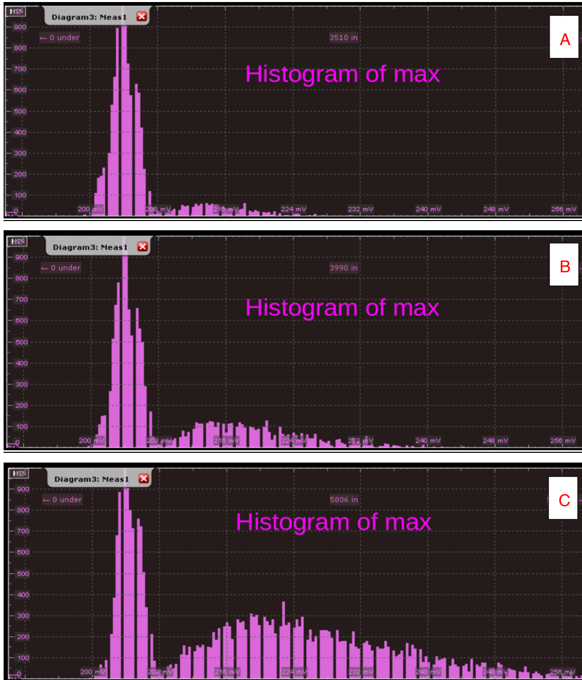
Figure 5. 40 Signal recovered from the micromesh for E_{drift} = 600 V/cm and a resistive layer voltage of 510 V (A), 530 V (B) and 560V (C).
