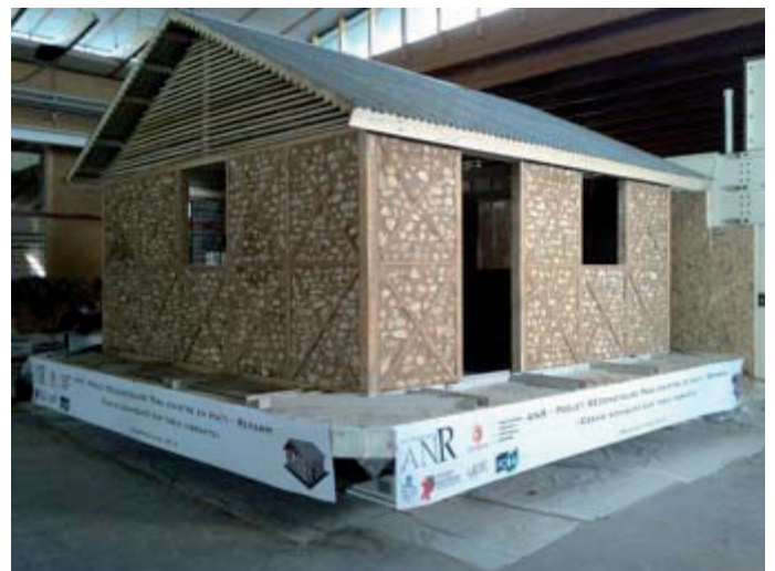
Figure 4. Prototype ready to be tested on FCBA vibrating table at FCBA in Bordeaux (credits: Christian Belinga Nko'o)
