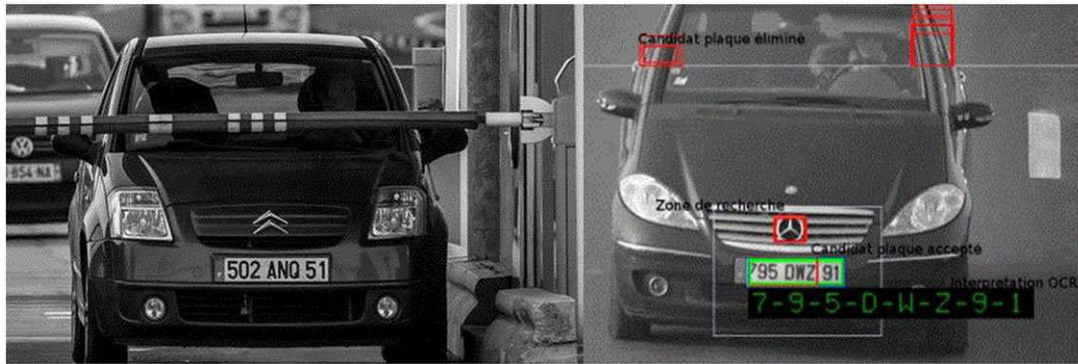
FIGURE 2 License plate detection and recognition in a configuration of 2 monitored toll lanes (2-lane license plate recognition) [Colour figure can be viewed at wileyonlinelibrary.com]
