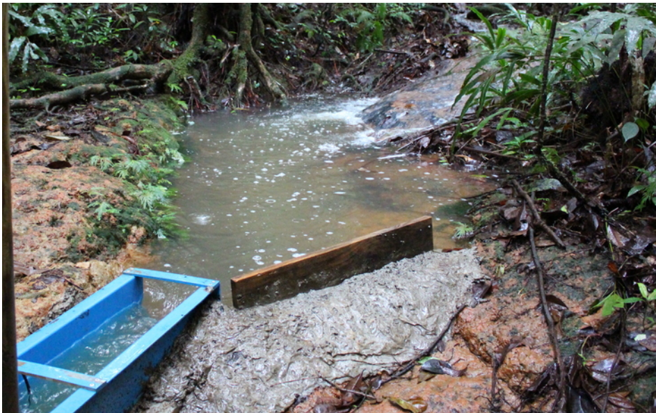
Figure 4.5: Picture of the concrete dam which focuses the stream into the Venturi flume, up to a water height of about 24.7 cm.
