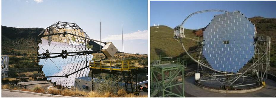
Figure 3.1: Telescopes of the VERITAS array (left) and the MAGIC array (right). The reflectors of these telescopes are composed by small mirror facets.
