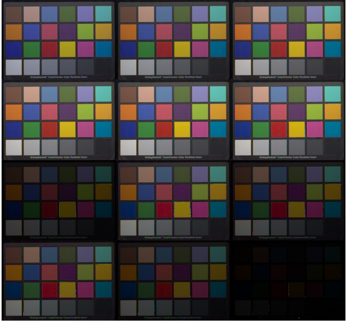
Figure 6-10: Effect of \lambda_\sigma on demosaicing for the Macbeth chart in Finlayson database for 4x4 SFA size, 16 filters. Left to Right, then Top to Bottom \lambda_\sigma goes [0.25, 0.5, 1, 2, 3, ..., 10]
