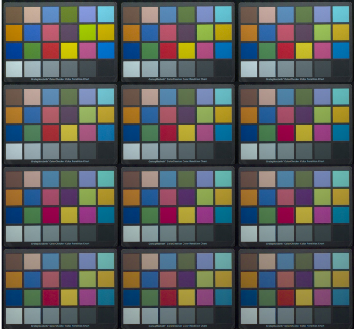
Figure 6-7: ] Effect of \lambda_\sigma on demosaicing for the Macbeth chart in Finlayson database for Bayer SFA. Output images are white-balanced by ratio of average Red, Green and Blue pixel values. Left to Right, then Top to Bottom \lambda_\sigma goes [0.25, 0.5, 1, 2, 3, ..., 10]
