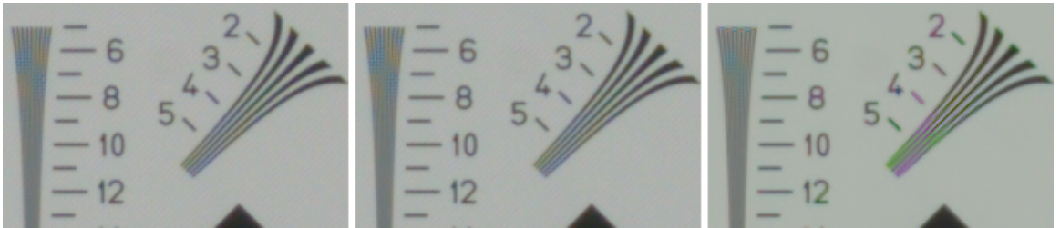
Figure 7-7: Demosaiced RAW Image from Monno5ch SFA camera. Left to Right: Ours NN, LMMSE, WGF. Notice less false colors with NN and LMMSE, however there are artifacts in flat regions.
