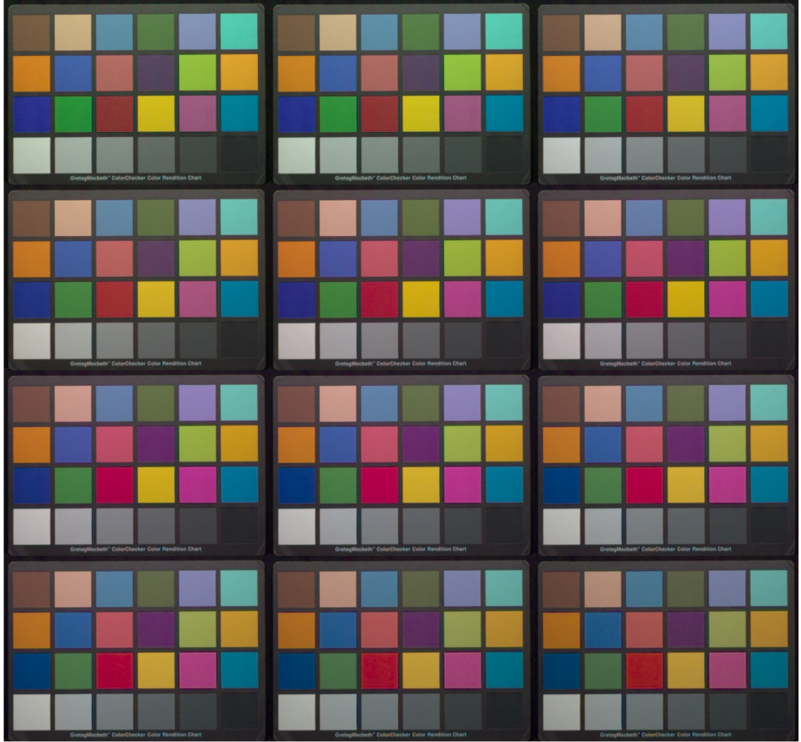
Figure 6-8: Effect of \lambda_\sigma on demosaicing for the Macbeth chart in Finlayson database for 2x2 SFA size, 4 filters. Left to Right, then Top to Bottom \lambda_\sigma goes [0.25, 0.5, 1, 2, 3, ..., 10]
