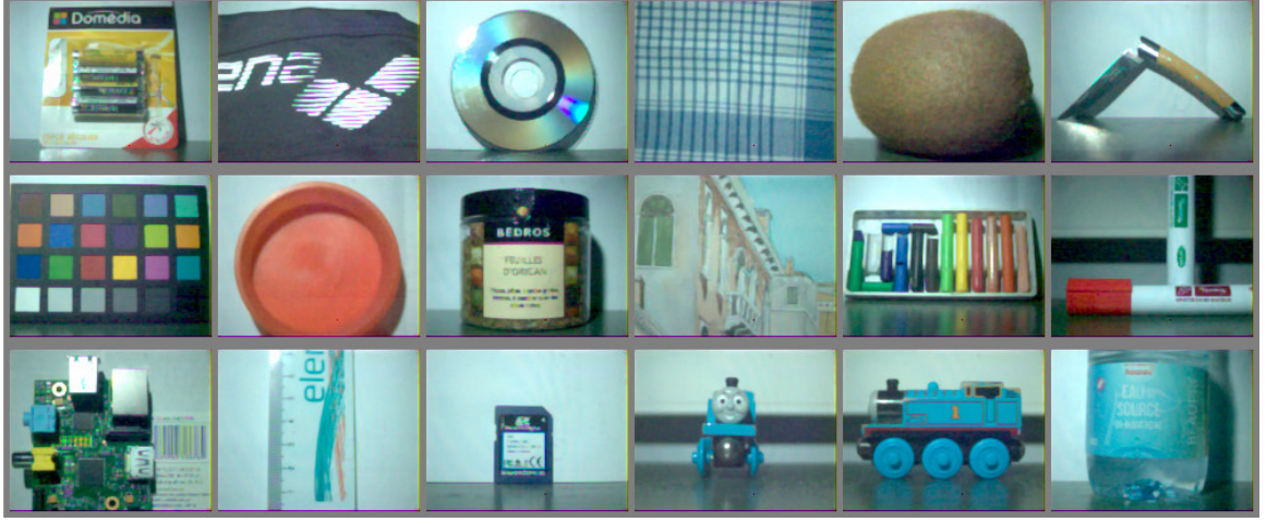
Figure 5-9: Visualization of SFA images demosaiced by the binary-tree and rendered in sRGB space.
