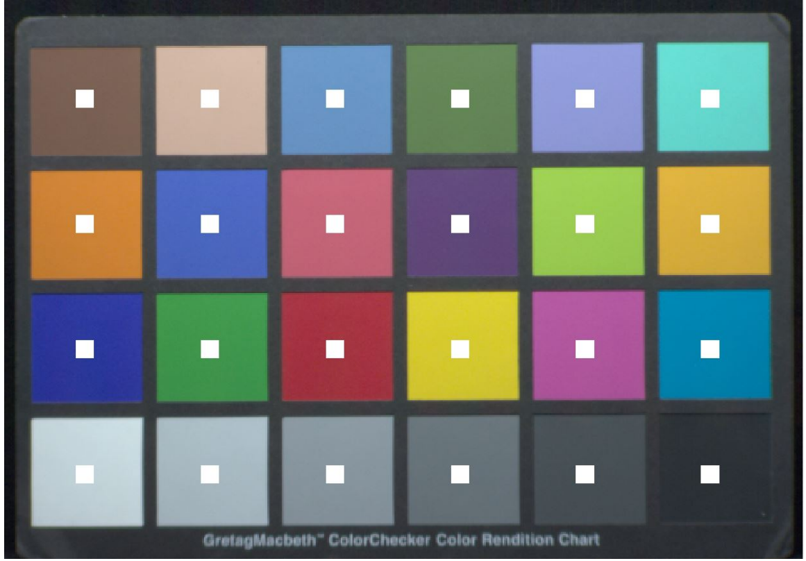
Figure 6-11: Macbeth chart image from the Finlayson database is overlaid with white patches of 10 \times 10 pixels. We average pixels from each patch to get an average reflectance value for each color. This average reflectance value is used to determine the PSNR of reflectance \mu_{z(chart)} between measured (in Finlayson database) and estimated from demosaicing operator D_s
