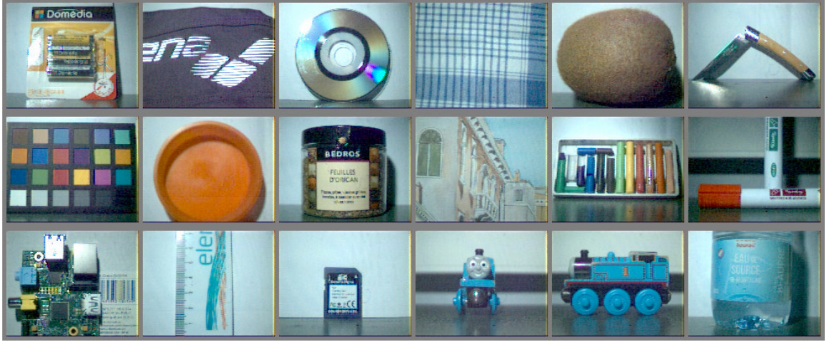
Figure 5-10: Visualization of SFA images demosaiced by N-LMMSE and rendered in sRGB space.
