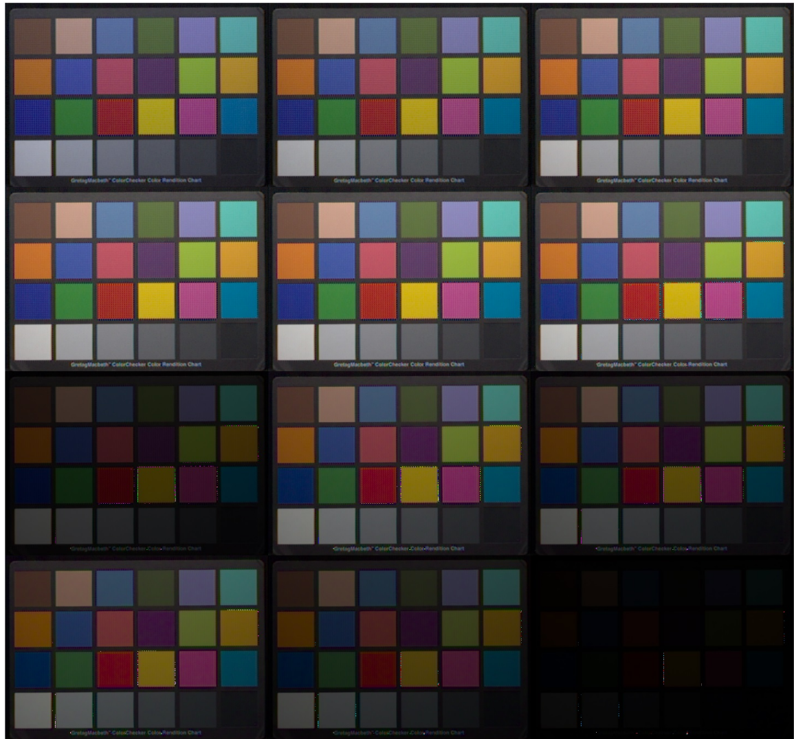
Figure 6-10: Effect of \lambda_\sigma on demosaicing for the Macbeth chart in Finlayson database for 4x4 SFA size, 16 filters. Left to Right, then Top to Bottom \lambda_\sigma goes [0.25, 0.5, 1,2,3,...10]
