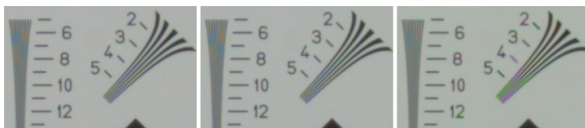
Figure 7-7: Demosaiced RAW Image from Monno5ch SFA camera. Left to Right: Ours NN, LMMSE, WGF. Notice less false colors with NN and LMMSE, however there are artifacts in flat regions.
