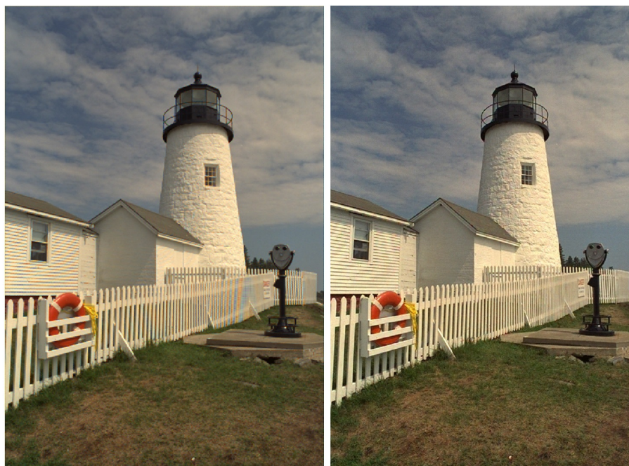
Figure 3-20: Left: Demosaiced Lighthouse image for the Bayer CFA using bilinear interpolation. Right: Demosaiced image using our approach considering totally random CFA. We see that we have no false colors in the fence region in the random case.
