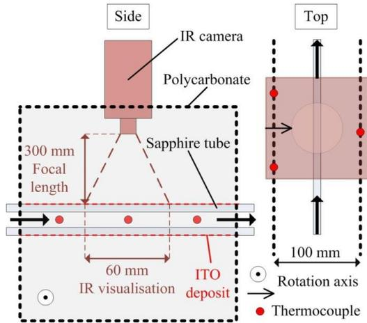
Figure 3-33. Top and side view of the IR test section. Polycarbonate plates enable to measure the equivalent temperature of the test section surroundings (Layssac et al., 2018b)
