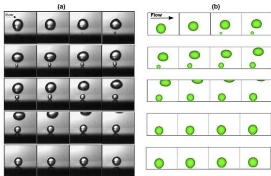
Figure 3-6. Example of comparison between experiments and simulations of a growing bubble in a subcooled convective flow (Lal et al., 2015)
