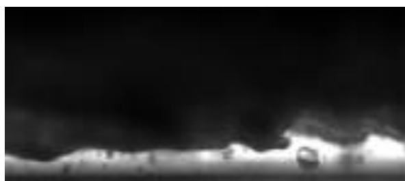
Figure 3-10 Example of liquid film LIF visualization (Schubring et al., 2010)
