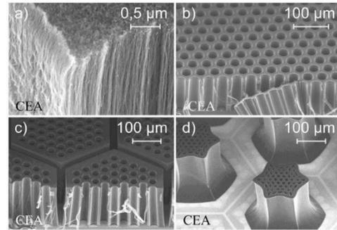
Figure 4-11. SEM images of different configurations of the CNT array: edge of a standard CNT array (a), array with holes (b), array with holes and hexagonal splits before (c) and after (d) densification (images and fabrication: CEA-Liten) (Kinkelin et al., 2017)
