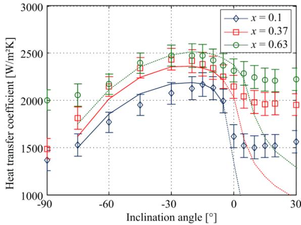
Figure 3-44. Comparison of the model predictions with experimental results ( $G = 200 \text{ kg/m}^2\text{s}$ ). Dashed lines mean that the flow is not stratified according to Crawford et al. (1985)(Lips and Meyer, 2012c)
