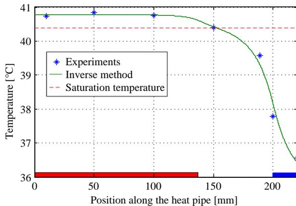
Figure 2-17. Example of comparison between an experimental temperature profile and the corresponding profile calculated by the inverse method ( $\dot{Q} = 20$  W; horizontal orientation) (Revil-Baudard and Lips, 2015)
