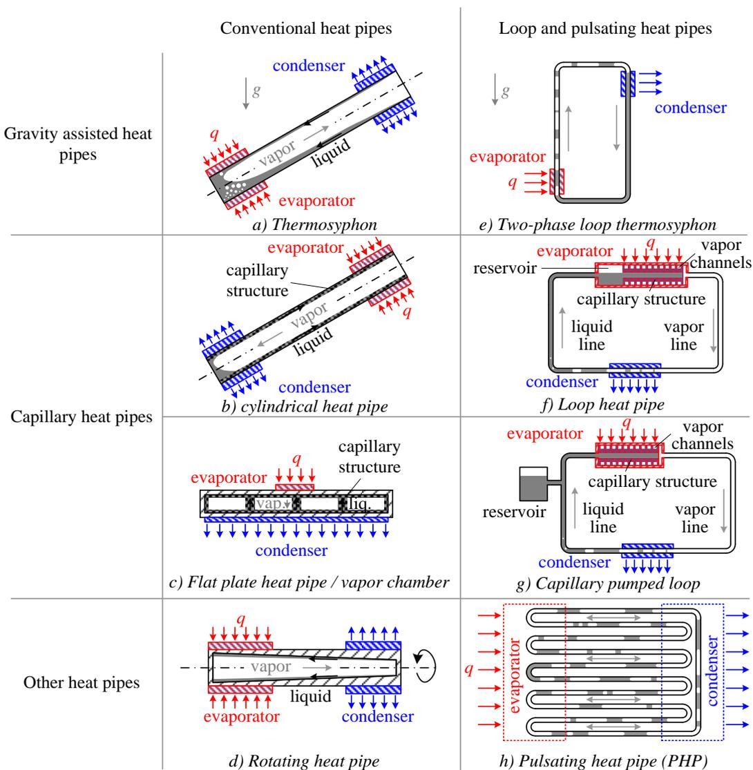
Figure 2-1. Different heat pipe technologies (Lips, 2015)
