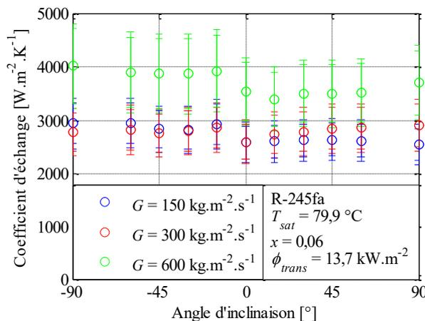
Figure 3-46. Variations of the heat transfer coefficient with the inclination angle for various mass fluxes ( $x = 0.06$ ) (Layssac, 2018)
