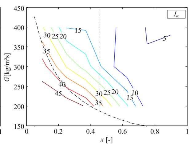
Figure 3-67. Map of the inclination effect on the heat transfer coefficient (R134a,  $d = 8.38 \text{ mm}$ ) (Lips and Meyer, 2012e)
