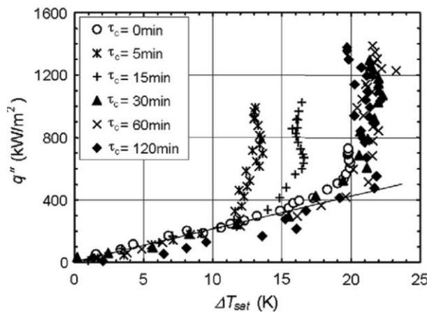
Figure 2-7. Example of the effect of the nanostructuring of the wall on the boiling curve obtained with  $\gamma$ -Fe<sub>2</sub>O<sub>3</sub> nanoparticle on a 100  $\mu$ m platinum wire.  $\tau_c$  is the nano-particle coating duration with pure water (Stutz et al., 2011)
