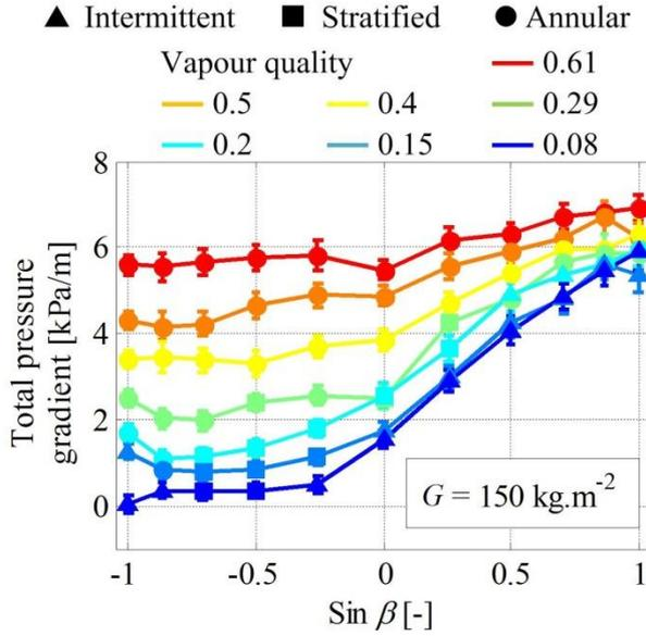
Figure 3-52. Evolution of total pressure gradient as a function of the inclination angle for convective boiling of R245fa in a 1.6 mm tube and a mass velocity of  $150 \text{ kg.m}^{-2}.\text{s}^{-1}$  (Laysac et al., 2018a)
