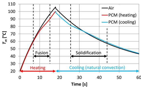
Figure 4-18. Temperature history of prototype thermal dampers with and without PCM (Kinkelin et al., 2017)
