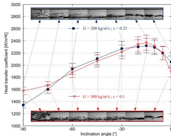
Figure 3-40. Flow patterns and heat transfer coefficients for downward flows at low mass fluxes and low vapour qualities (Lips and Meyer, 2012a)
