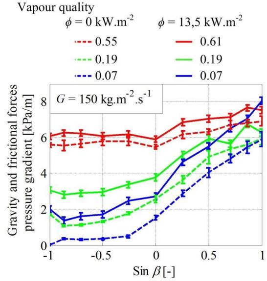
Figure 3-53. Comparison of pressure gradient evolution with inclination angle with an imposed heat flux of  $13.5 \text{ kW.m}^{-2}$  (filled lines) and without heat flux (dot lines) (Laysac et al., 2018a)
