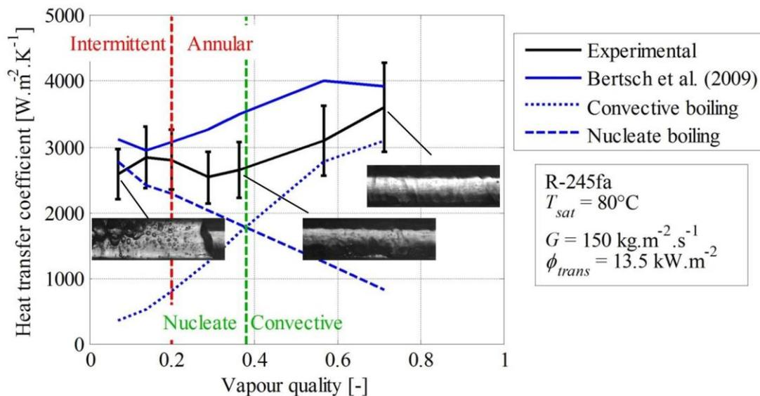
Figure 3-49. Prediction of the variations of the nucleate and convective heat transfer mode with vapour quality from Bertsch et al. (2009) model for a mass velocity of  $150 \text{ kg.m}^{-2}.\text{s}^{-1}$  (Layssac, 2018)
