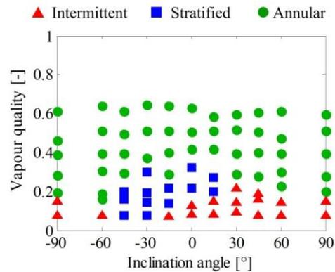
Figure 3-23. Example of experimental flow pattern map of Layssac et al. (2018a) (R245fa,  $d = 1.6$  mm,  $G = 150$  kg.m<sup>-2</sup>.s<sup>-1</sup>;  $\varphi = 0$  kW.m<sup>-2</sup>)
