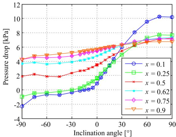
Figure 3-50. Measured pressure drops for different vapour qualities (R134a,  $d = 8.38$  mm;  $G = 300$  kg/m<sup>2</sup>s) (Lips and Meyer, 2012b)
