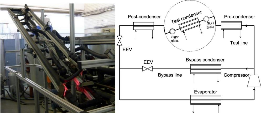
Figure 3-16. Picture and schematic diagram of the experimental setup of Lips and Meyer (2011b) for the study of convective condensation in an inclined orientation
