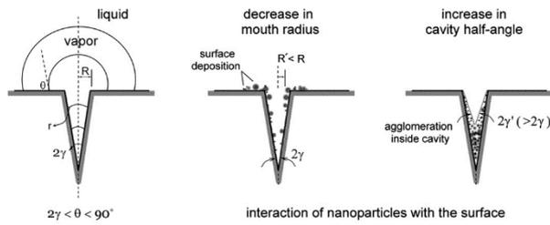
Figure 2-5. Possible clogging of nanoparticles in a nucleating cavity affecting the boiling phenomenon (Khandekar et al., 2008)
