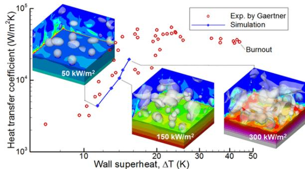
Figure 3-7. Example of boiling modelling taking into account the bubble merging (Sato and Niceno, 2017)
