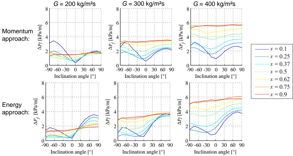
Figure 3-61. Impact of the approach for the frictional pressure drop determination (Lips and Revellin, 2013)
