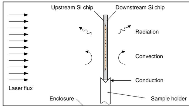
Figure 4-17. Thermal boundary conditions for the TIM-TS (Kinkelin et al., 2015)
