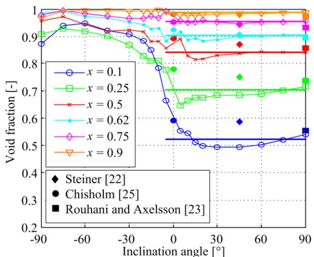
Figure 3-57. Effect of inclination angle on the apparent void fraction and comparison with different correlations (R134a,  $d = 8.38 \text{ mm}$ ,  $G = 300 \text{ kg/m}^2\text{s}$ ). The thick horizontal lines represent the mean apparent void fraction between  $-5^\circ$  and  $90^\circ$  (Lips and Meyer, 2012b)
