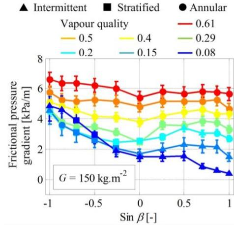
Figure 3-55. Evolution of the frictional pressure gradient as a function of the inclination angle for a mass velocity of  $150$  kg.m<sup>-2</sup>.s<sup>-1</sup> (Layssac et al., 2018a)
