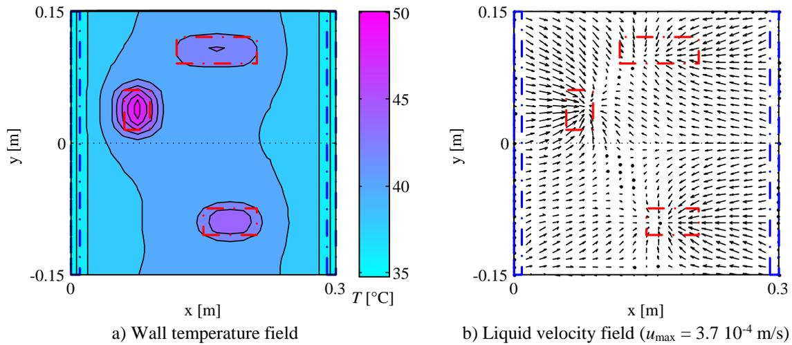
Figure 2-11. Example of thermal and hydrodynamic results obtained with the analytical model for a flat plate heat pipe with three heat sources and two heat sinks (Lips and Lefèvre, 2014)
