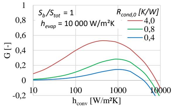
Figure 2-38. Thermal gain for various PCB spreading efficiency, characterized by  $R_{cond,0}$  (Lips et al., 2017b)
