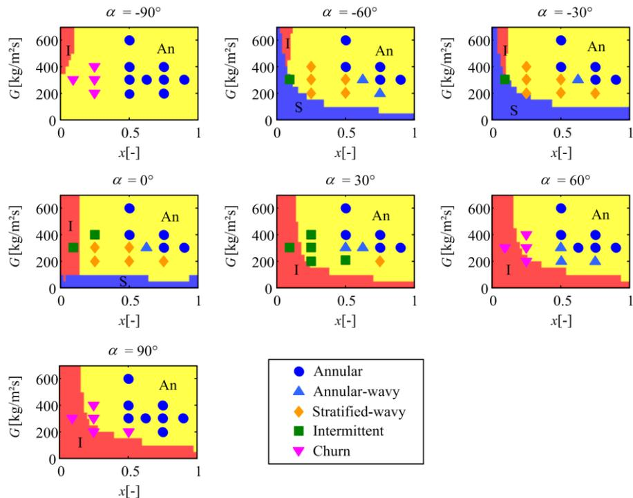
a) flow patterns of Lips and Meyer (2012a) (R134a,  $d = 8.38$  mm)
