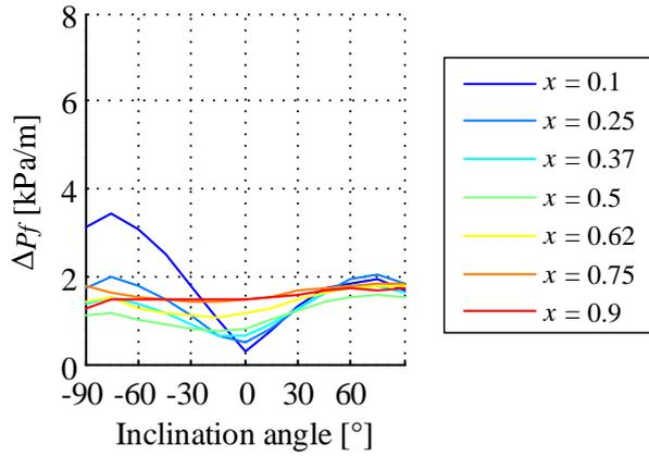
Figure 3-54. Evolution of the frictional pressure gradient as a function of the inclination angle (R134a,  $d = 8.38$  mm;  $G = 200$  kg/m<sup>2</sup>s)
