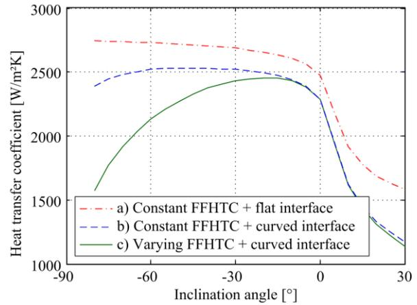
Figure 3-45. Influence of different assumptions on the model predictions. FFHTC: Falling film heat transfer coefficient ( $G = 200 \text{ kg/m}^2\text{s}$ ;  $x = 0.3$ ;  $\Delta T = 2 \text{ K}$ ) (Lips and Meyer, 2012c)
