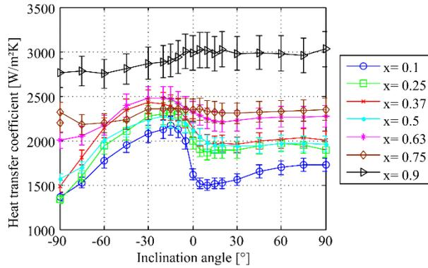
Figure 3-37. Experimental heat transfer coefficient during convective condensation of R134a in a 8.38 mm tube ( $G = 200 \text{ kg/m}^2\text{s}$ ,  $-90^\circ$  : downwards,  $0^\circ$  : horizontal;  $90^\circ$  vertical upwards) (Lips and Meyer, 2012c)
