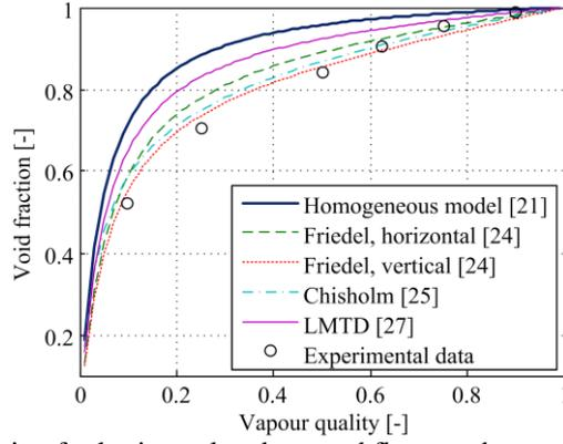
Figure 3-58. Apparent void fraction for horizontal and upward flows and comparison with different correlations (R134a,  $d = 8.38$  mm,  $G = 300$  kg/m<sup>2</sup>s) (Lips and Meyer, 2012b)
