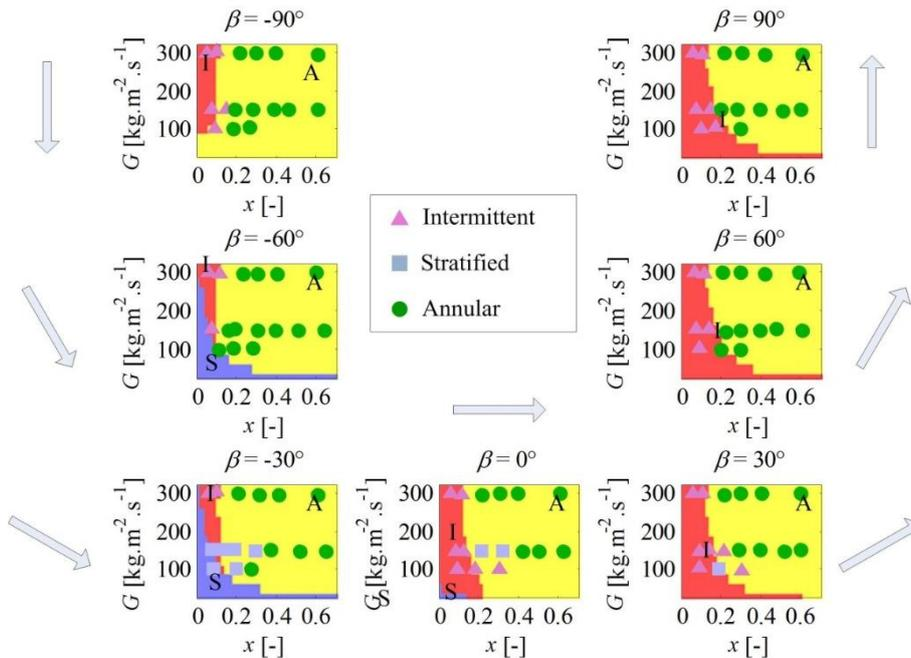
b) flow patterns of Layssac et al. (2018a) (R245fa,  $d = 1.6$  mm,  $\varphi = 0$  kW.m<sup>-2</sup>)
