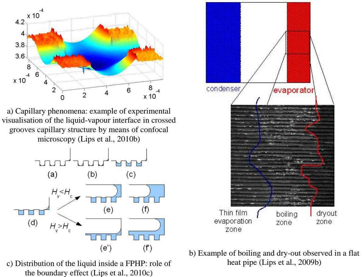
Figure 2-12. Example of phenomena occurring in heat pipes
