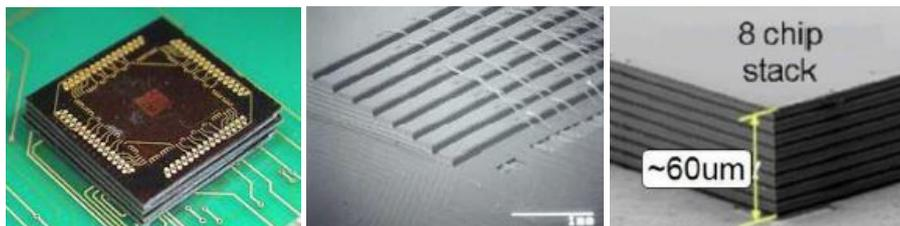
Figure 1-4. 3D electronic component (sources left: Fraunhofer IZM; centre: ITRS 2009; right: AES, Samsung)
