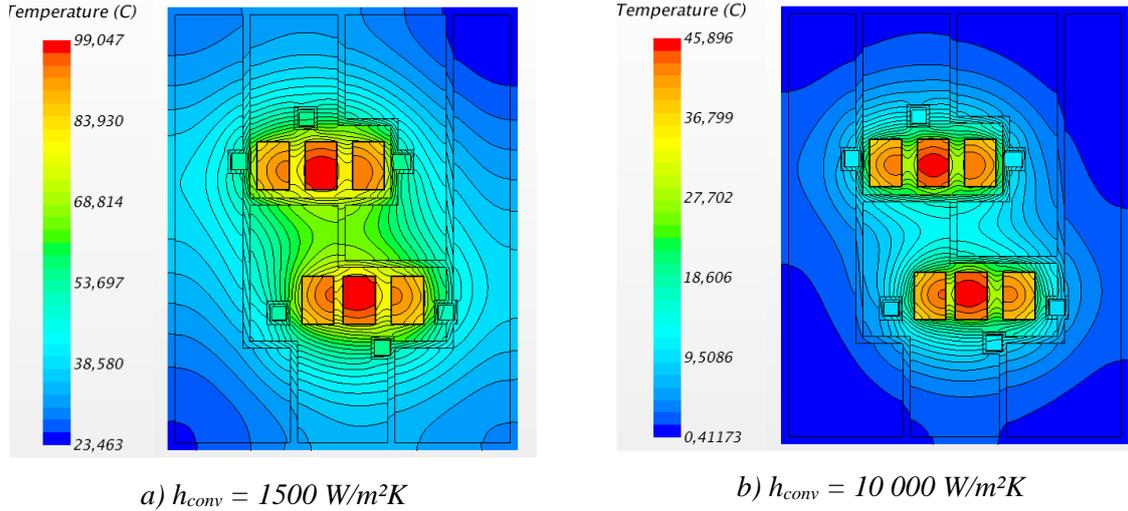
Figure 2-34. Examples of temperature fields in the PCB, calculated by CFD modelling for two different heat transfer coefficient with the heat sink ( $Q = 25$  W/components and  $T_{amb} = 0^\circ\text{C}$ ) (Lips et al., 2017b)
