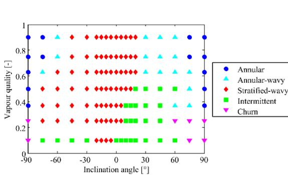
Figure 3-22. Example of experimental flow pattern map of Lips and Meyer (2012c) (R134a,  $d = 8.38$  mm,  $G = 200$  kg/m<sup>2</sup>s)
