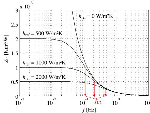
Figure 4-3. Thermal impedance in the single-phase zone of the ideal thermal damper associated to the geometry considered in figure 4-2 (Kinkelin et al., 2017)
