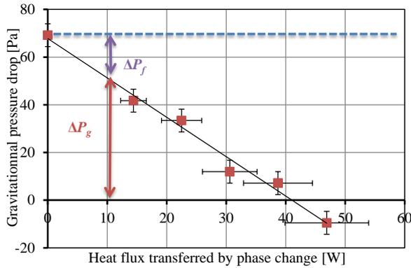
Figure 2-19. Example of evolution of the gravitational pressure drop as a function of the heat transfer rate transferred by phase change ( $L_{\text{evap}} = 140 \text{ mm}$ ) (Revil-Baudard and Lips, 2015)
