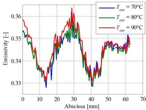
Figure 3-35. Variations of the ITO deposit emissivity with abscissa for sapphire outer wall temperature of 70°C, 80°C and 90°C (Layssac et al., 2018b)
