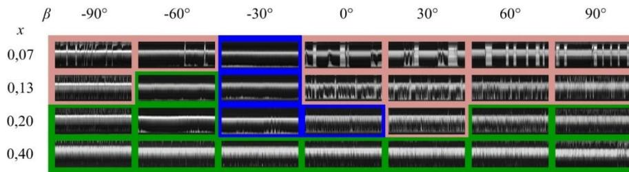
Figure 3-21. Evolution of flow patterns (pink: intermittent; blue: stratified; green: annular) and time representative frames for various vapour qualities and inclination angles (R245fa,  $d = 1.6$  mm,  $G = 150$  kg.m<sup>-2</sup>.s<sup>-1</sup>) (Layssac et al., 2018a)
