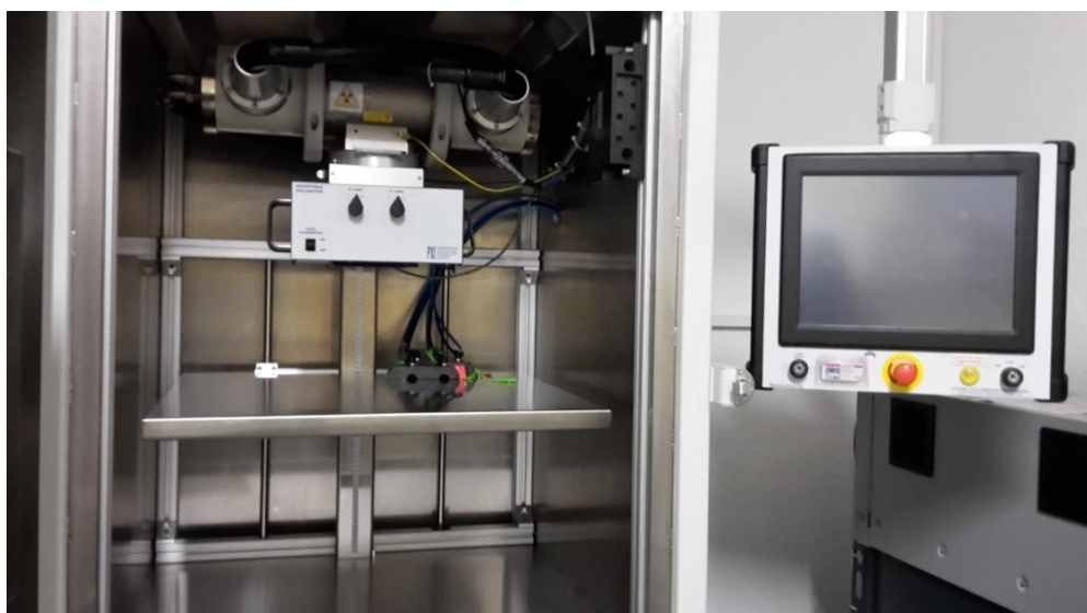
Figure 48: Photo of the interior of the X-ray irradiator (Laboratory of Cellular and Molecular Radiobiology, Lyon-Sud Medical School, Lyon, France).
