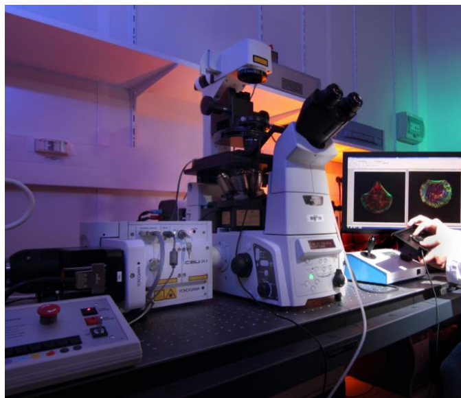
Figure 50 : Confocal spinning-disk microscope ( \mu Life Platform, CEA-Grenoble, Grenoble, France). A kinetic study was also done in order to observe the internalization of AGuIX® in time: 1h – 2h – 4h – 6h.
