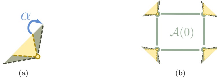
Figure 1.17: (a) A 2D tangent cone before (yellow) and after (green) dilation by an angle \alpha . (b) Shape \mathcal{A} from Figure 1.18 after decomposition into a simplicial complex, with all its vertices tangent cone polars (yellow) and their dilated versions (green).
