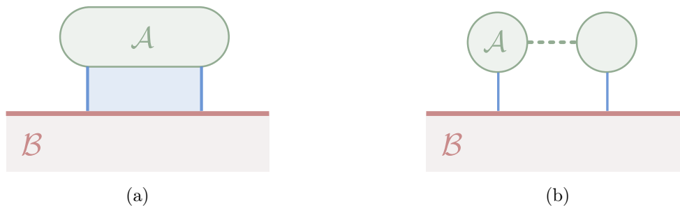
Figure 1.7: Two scenarios with identical feasible spaces. (a) is composed of a capsule \mathcal{A} and an infinite horizontal plane \mathcal{B} . (b) replaces the capsule by a pair of rigidly linked disks. In both scenarios, \mathcal{A} has three degrees of freedom (two translations and one rotation) and \mathcal{B} is static. In the two illustrated configurations, only a finite number of constraints (blue in (b)) is sufficient even if (a) has an infinite number of local minimizers of the distance function.
