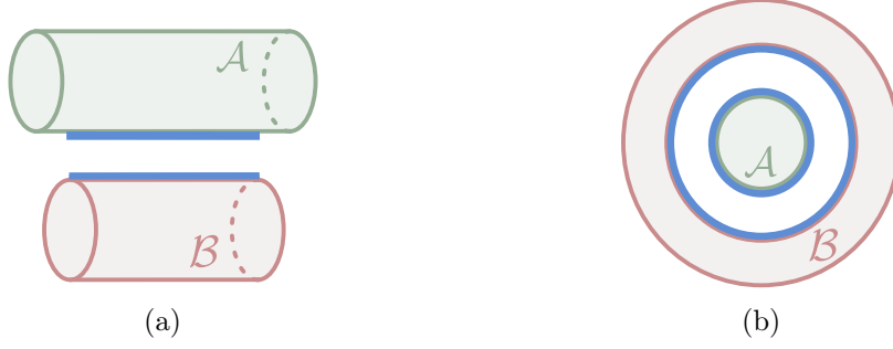
Figure 4.7: Two configurations considered ‘conformal’ even if there is no effective contact between \mathcal{A} and \mathcal{B} . The conformal contact areas, i.e., the footpoints of the non-punctual non-strict local minima of the squared distance function, are highlighted in blue.
