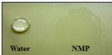
Figure 3.25. Droplets water and NMP on the surface of PEEK.
