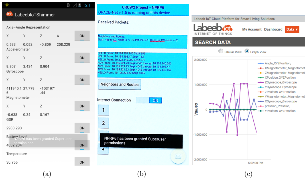
FIGURE 4.4: (a) A screen-shot from the Labeeb-IoT Shimmer sensing mobile app, which collects data from Shimmer [120] sensors and pushes them to the Internet of Things platform (Labeeb-IoT). (b) Testbed: a photo of the ORACE-Net mobile devices displaying the real-time events (received "Hello" and Advertisement ("ADV") packets) and the current route. (c) The Labeeb-IoT [121] interface shows the variation of the sensed data from the Shimmer sensor connected to the mobile node.
