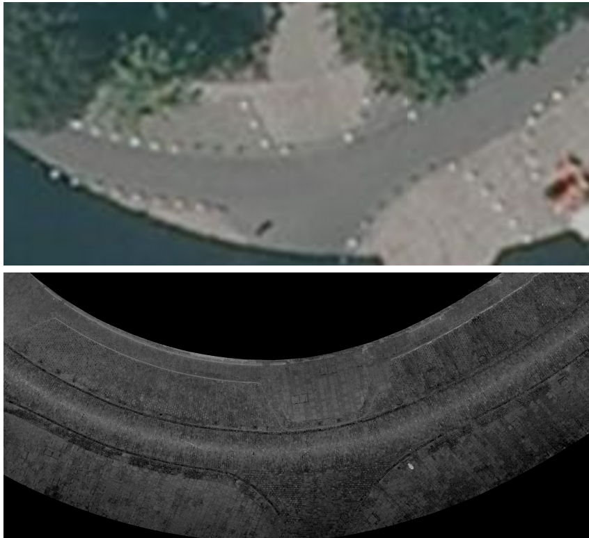
Figure 2.11: Comparison between aerial orthophotography (top) and MLS orthoimage (bottom). The MLS reconstruction contains \sim 6.10^6 px in which 72% were obtained by diffusion, and 10% by exemplar-based inpainting.
