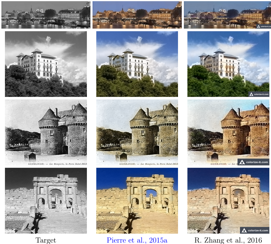
Figure 4.3: Comparison of the colorization results from our models in RGB (Pierre et al., 2015a) and in YUV (Pierre et al., 2014b) and from the fully automatic CNN approach of R. Zhang et al., 2016 (files obtained using http://demos.algorithmia.com/colorize-photos/ ). CNNs provide very impressive results for this task but some artifacts still remain.
