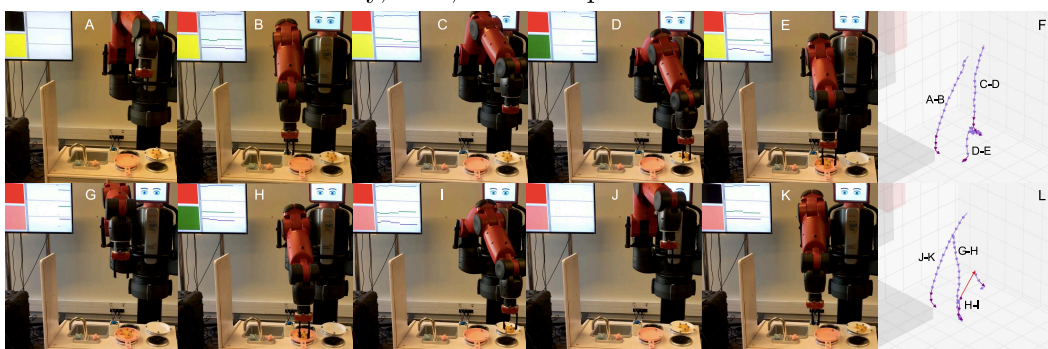
Figure 6.17: Actions of a successful execution of the task heating the croissant. From A to E, screenshots pushing the button, grasping the croissant, and putting it into the pan. In F, virtual representation of these actions. From G to H, screenshots grasping again the croissant, putting it back into the dish, and pressing the button. In L, virtual representation of these actions.
