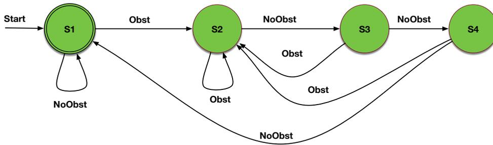
Figure 5.5 – Simple collision avoidance modelling as a *FSM*
