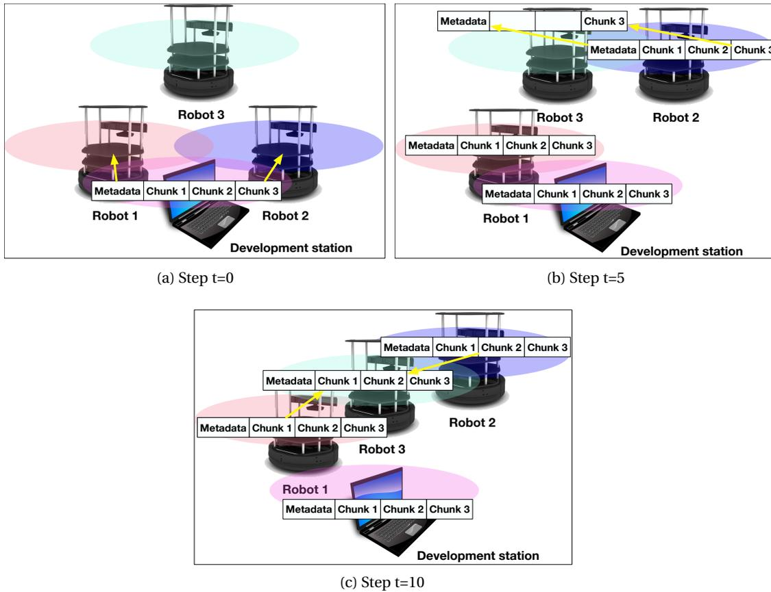
Figure 5.25 – ROSMDB fleet deployment process
