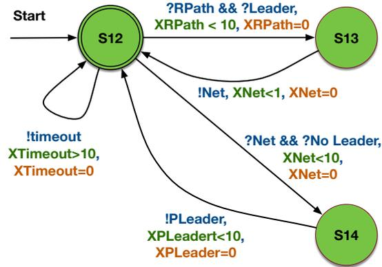
Figure C.6 – Networking component Event Recording Automaton
