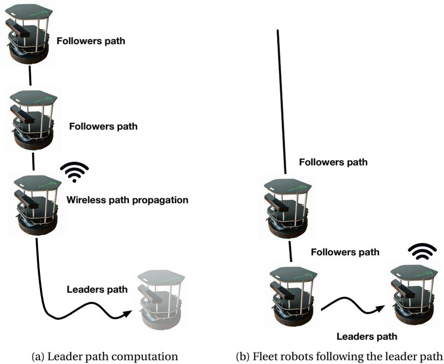
Figure 5.4 – Centralized fleet platooning via wireless communication
