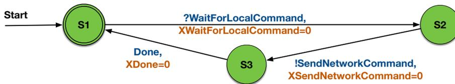
Figure 6.3 – Networking Model executed on each drone assigned laptop
