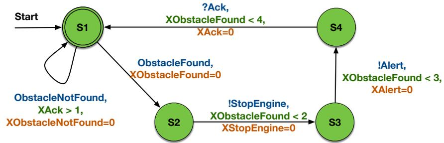
Figure 6.14 – Engine stopper Model executed on each robot
