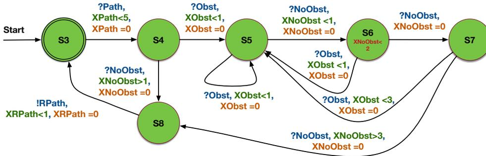
Figure C.2 – Navigation component Event Recording Automaton
