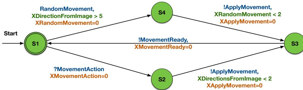
Figure 6.17 – Movement Model executed on each robot
