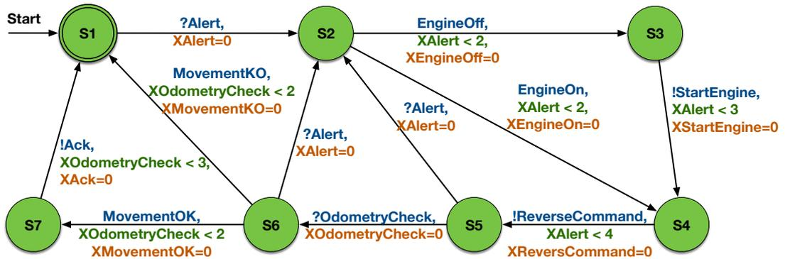
Figure 6.15 – Avoidance Model executed on each robot
