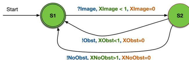
Figure C.1 – Optical sensor component Event Recording Automaton
