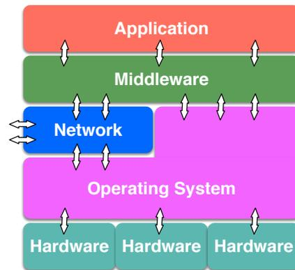
Figure 2.1 – Middleware layer interaction with the runtime stack
