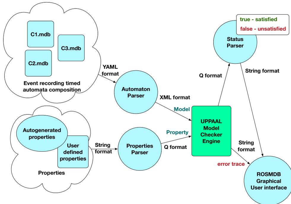
Figure 5.19 – Integration of ROSMDB with UPPAAL model-checker engine
