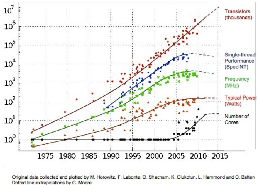
Figure 5.2 – Computing speed developments <sup>2</sup>over the years
