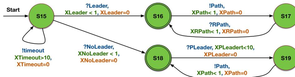
Figure C.7 – Platooning manager component Event Recording Automaton
