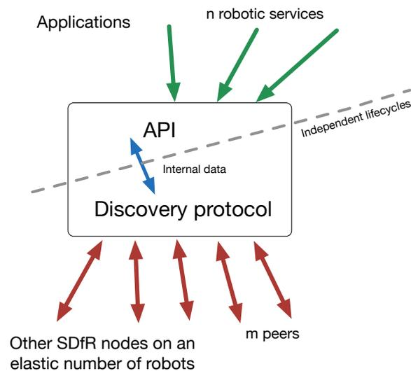
Figure 4.6 – Sdfr service architecture.
