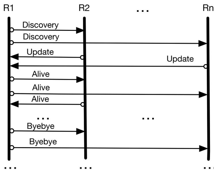
Figure 4.1 – SSDP and SDfR protocol timed diagram.
