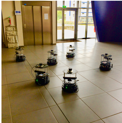
Figure 6.18 – Experimenting Random movement object search with Turtlebots
