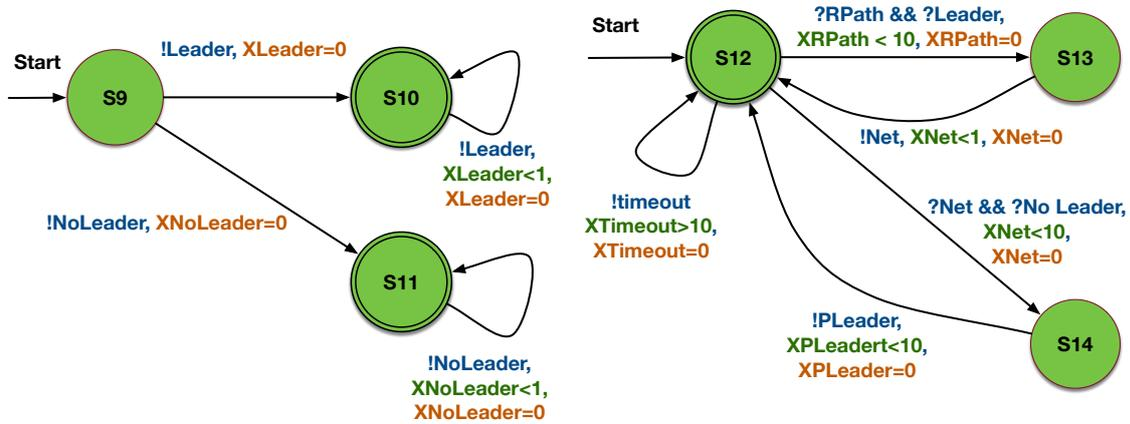
(a) Leader component Event Recording Automaton (b) Networking component Event Recording Automaton
