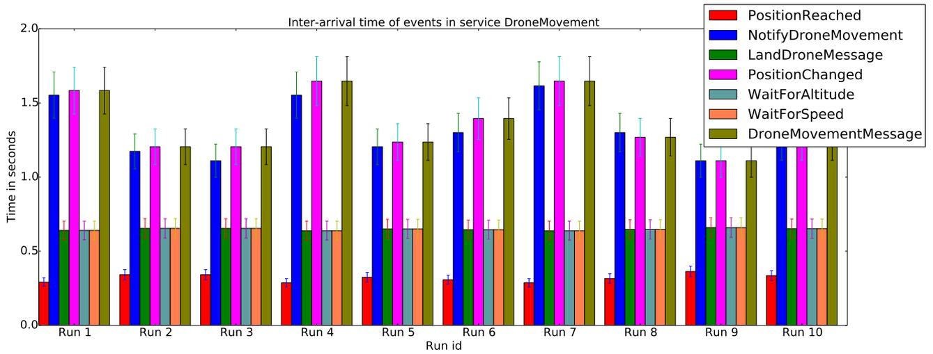
Figure 6.9 – Drone movement messages inter-arrival time
