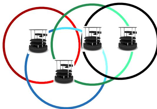
Figure 2.8 – Ad-hoc fleet infrastructure with per-robot communication ranges.
