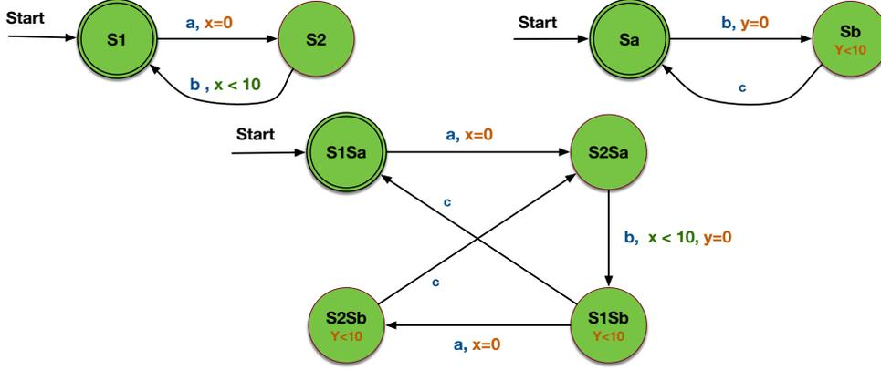
Figure 5.12 – Timed automata product construction example
