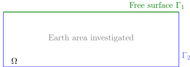
Figure 2.7: Distinction between artificial boundary conditions and free surface. The interface between the air and the medium, \Gamma_1 is a free surface. In seismic numerical applications, \Gamma_2 must ensure no reflection from incident waves.
