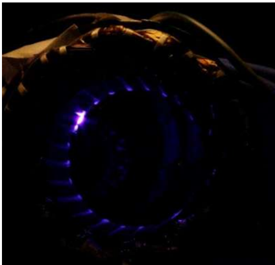
Figure I.8: Partial discharges in the slot (100 mbar)
