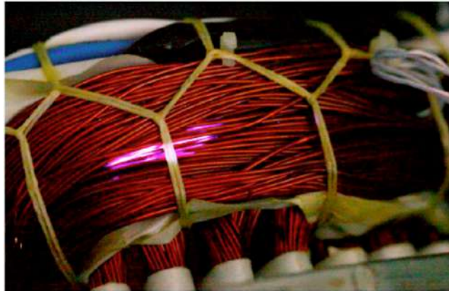
Figure I.25: Photo of the winding and presence of PD in the endwindings.
