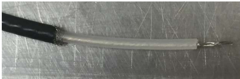
Figure I.20: Sensor based on coaxial cable
